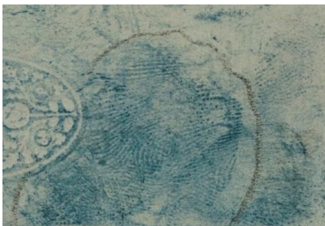
Fingermarks visualised by blue toning on old documents. A Physical Developer mark on a 1940s document (a) before toning, and (b) after toning showing increase in contrast
