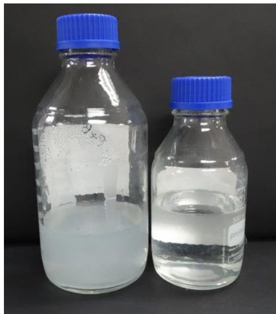
Stock detergent solutions made with Tween 20 (left) and Synperonic N (right) showing differences in solubility and thus cloudiness of the solution.
