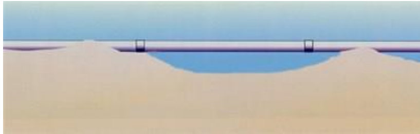
Figure 3.2 – Illustration of a pipeline freespan
