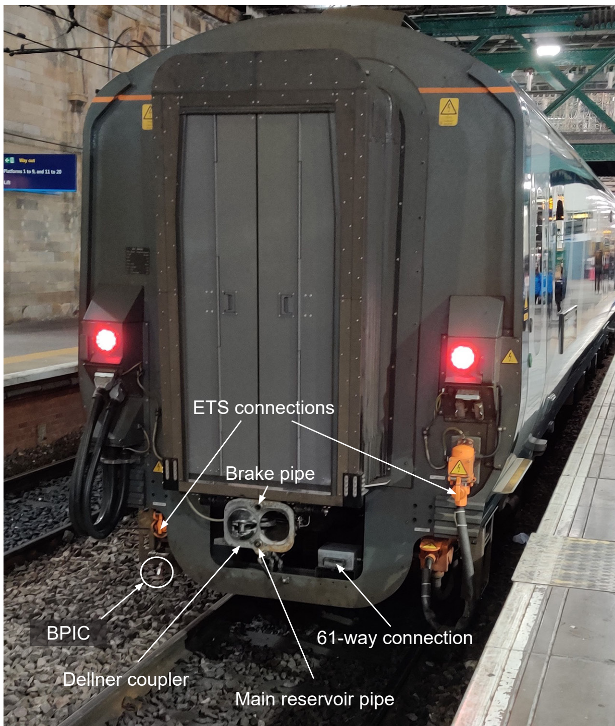
Figure 5: Mark 5 sleeper coach end, showing Dellner coupler and other connections
