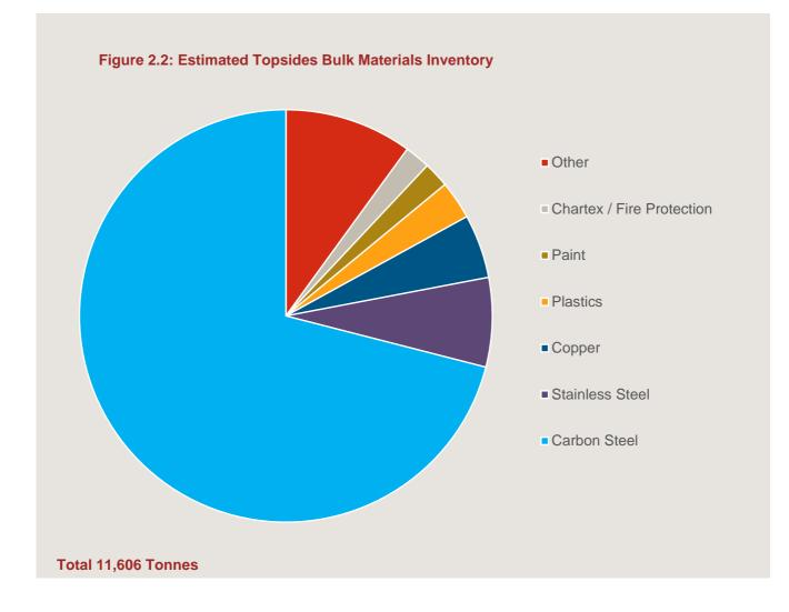
Please refer to Table 2.1 within the Environmental Appraisal for detailed materials inventory data. The total Topsides weight of 11,606te is inclusive of an estimated 731te of hazardous waste such as paint, passive fire protection and NORM, as shown in Figure 2.3.
