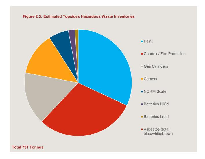
Please refer to Table 2.2 within the Environmental Appraisal for detailed materials inventory data. The total Topsides weight of 11,606te is inclusive of an estimated 731te of hazardous waste such as paint, passive fire protection and NORM, as shown above in Figure 2.3.
