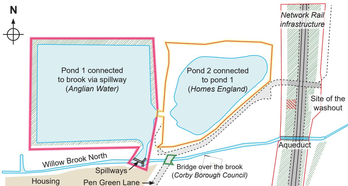
Figure 5: The assets relevant to the flooding in the Pen Green Lane area
