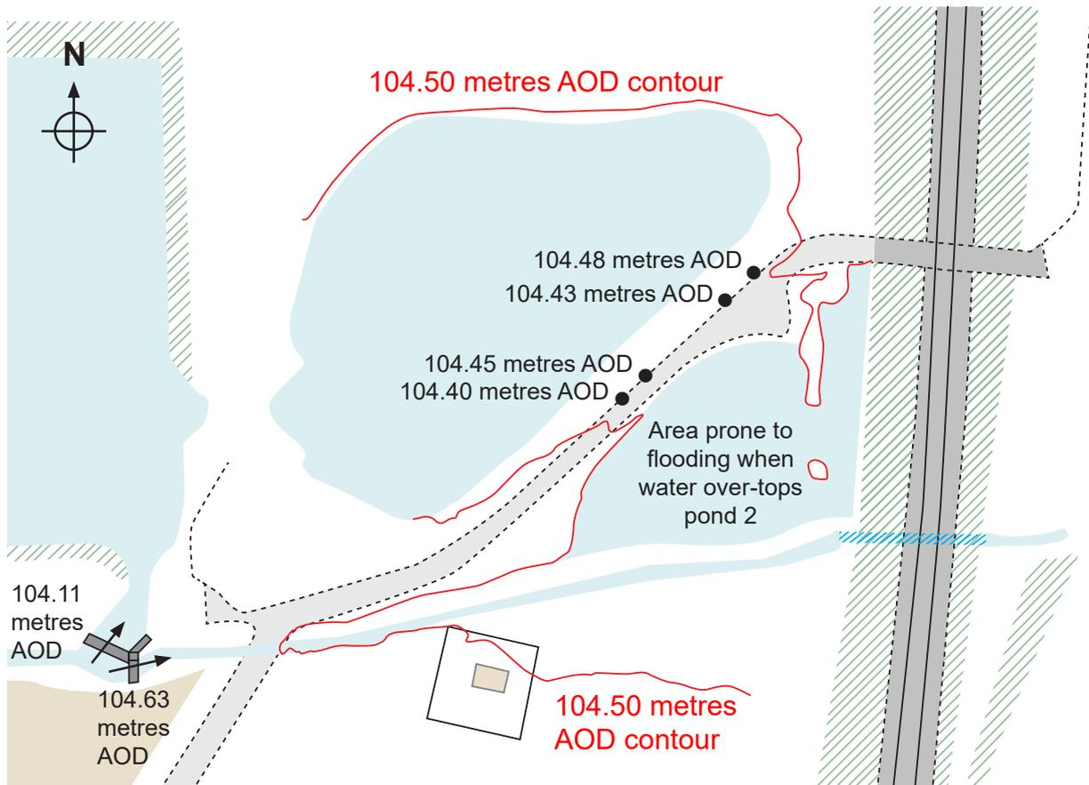
Figure 14: The levels as recorded by the surveys for the spillways and ground showing the low point on the eastern bank of pond 2
