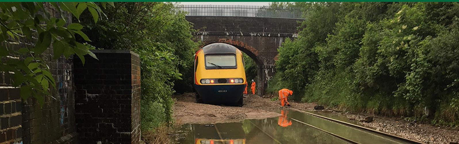
**Train collision with material washed out from a cutting slope at Corby, Northamptonshire
