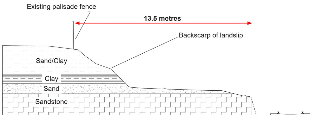
Figure 17: The geology of the failed cutting slope
