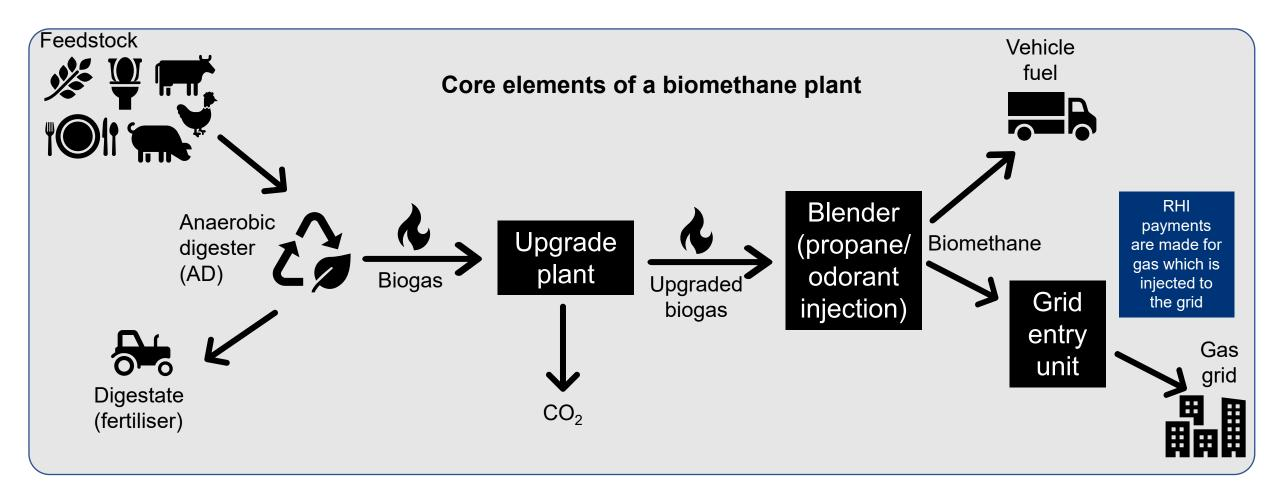
10 **Core elements of a biomethane installation**
