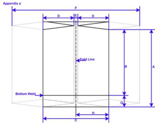
This is a double gusseted bag folded down the centre and heat sealed to create the star seal
