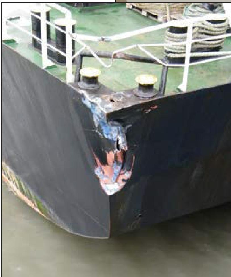
Figure 3: Damage to shell plating
