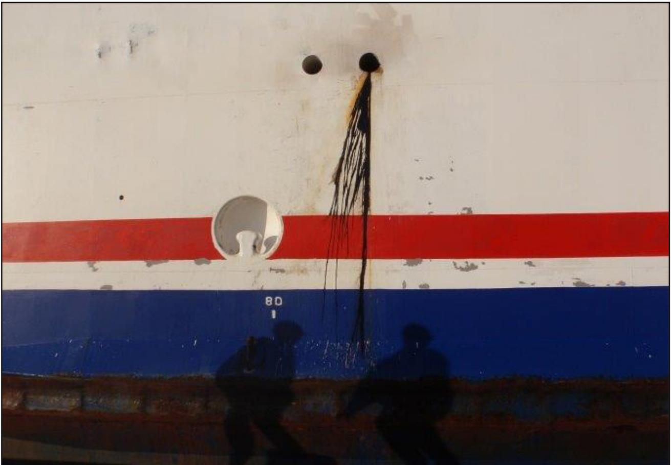
Figure 3: Oily water discharge on ship's side
