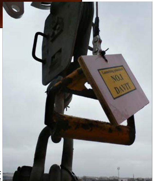
Figure 3: Slewing control wire triangular handle
