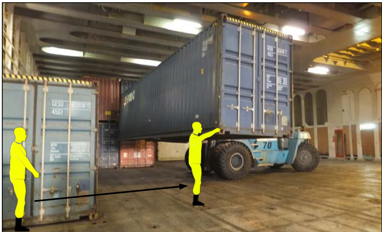
Figure 2: The crewman moves forward to remove an underslung twistlock
