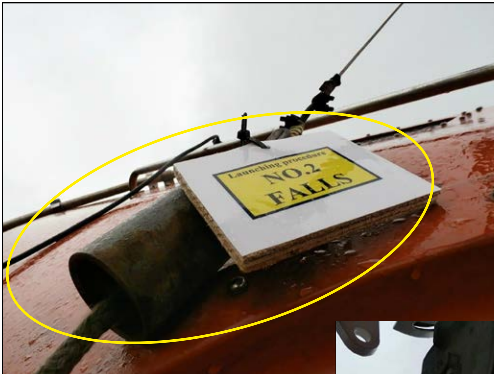
Figure 2: Brake release and falls lowering control wire cylindrical handle
