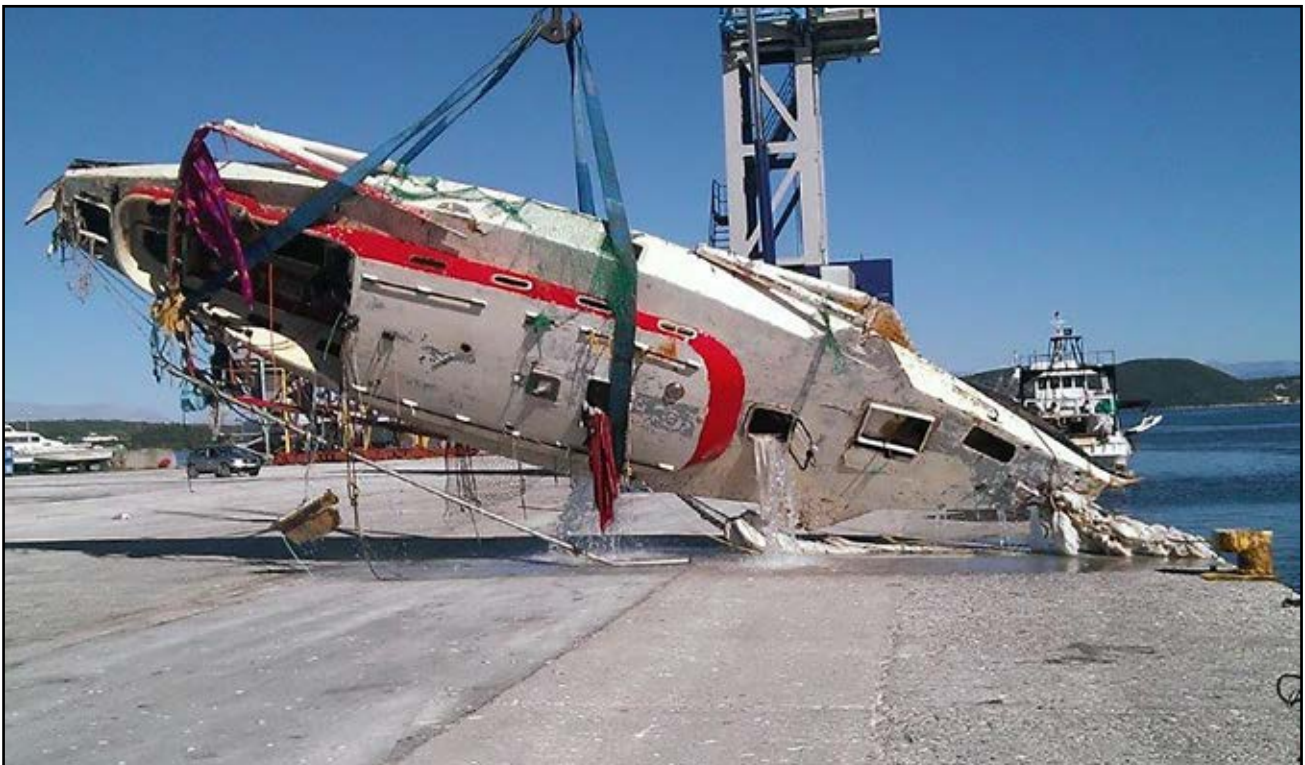
Figure 2: Hull lifted out of the water
