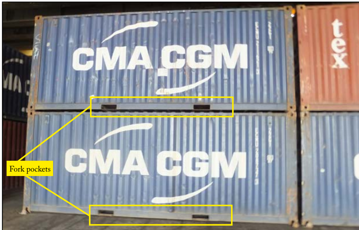
Figure 4: Fork pockets fitted to 20 foot containers which are not present on 40 foot units
