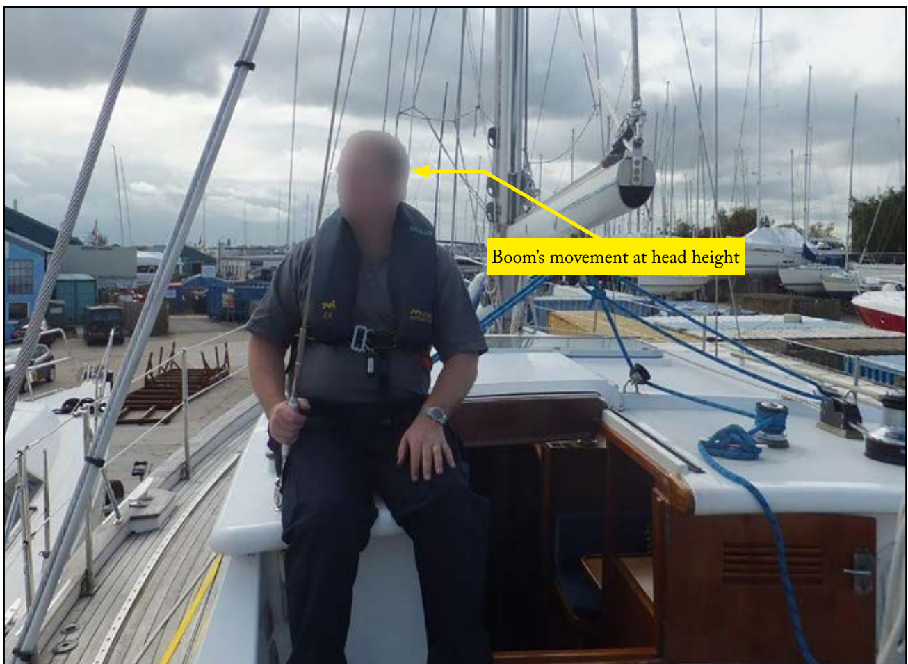
Reconstruction of the crewman's sitting position on the coach roof showing the boom at the same height as his head
