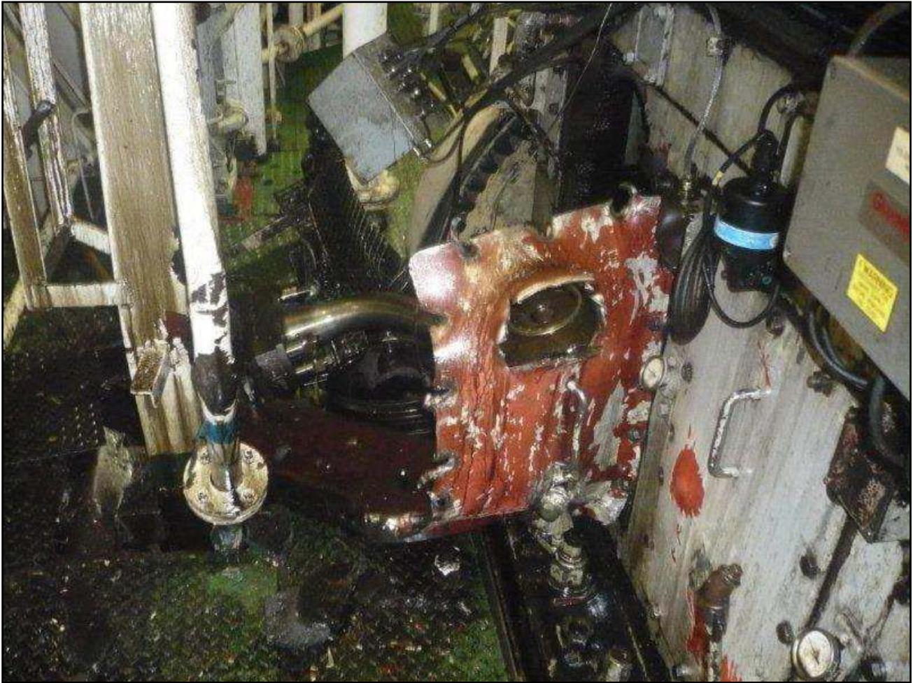
Condition of engine immediately after over-speed
