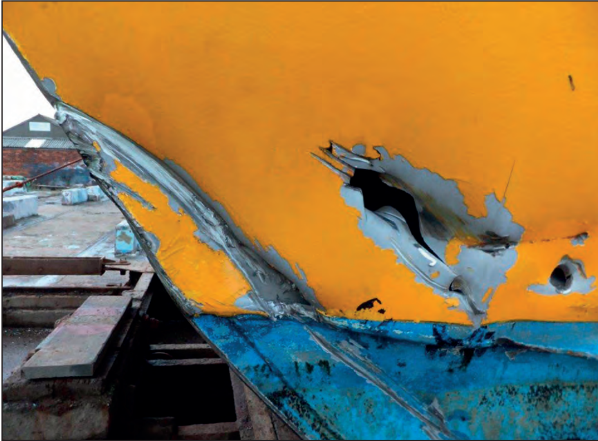
Figure 2: Penetration to the port hull shell plating
