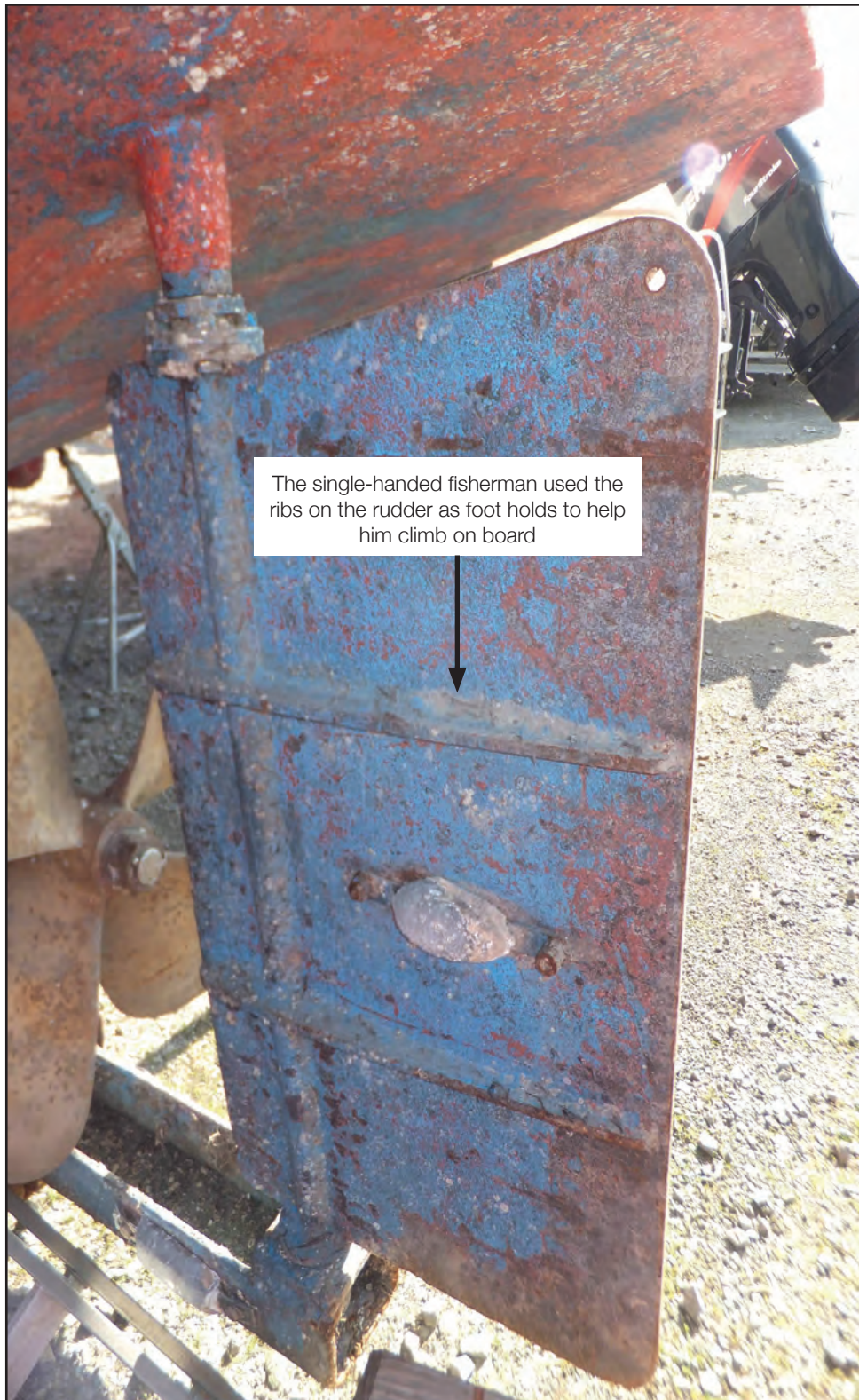
An example of a typical externally ribbed rudder
