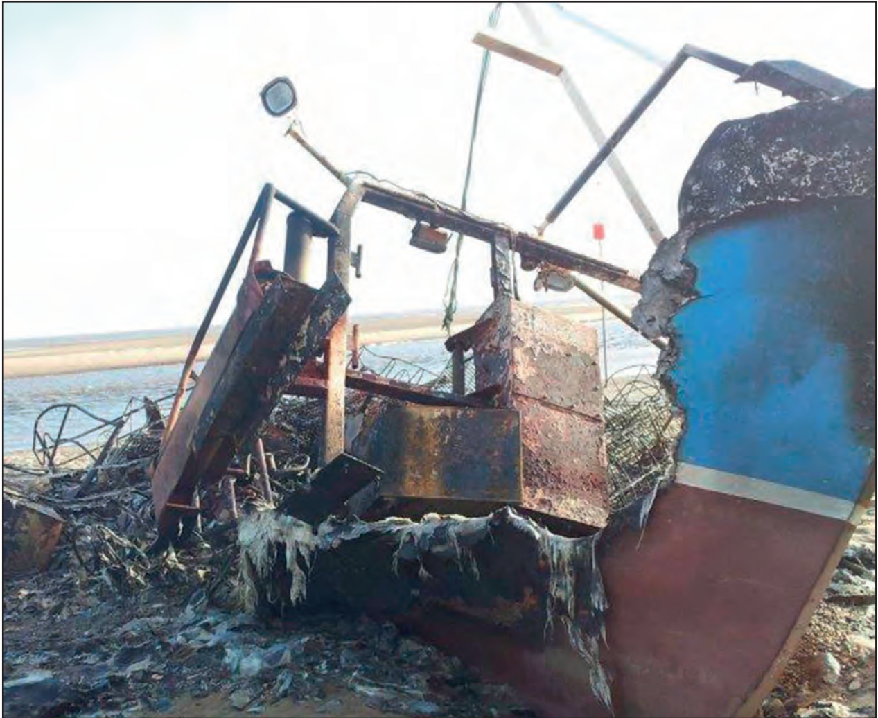
Figure 1: Burnt out wreck of the fishing vessel (looking aft)
