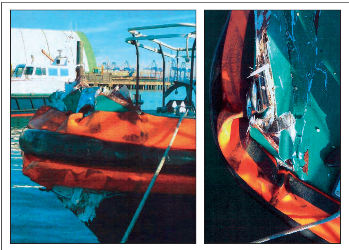
Figure 1: Damage sustained to the pilot boat
