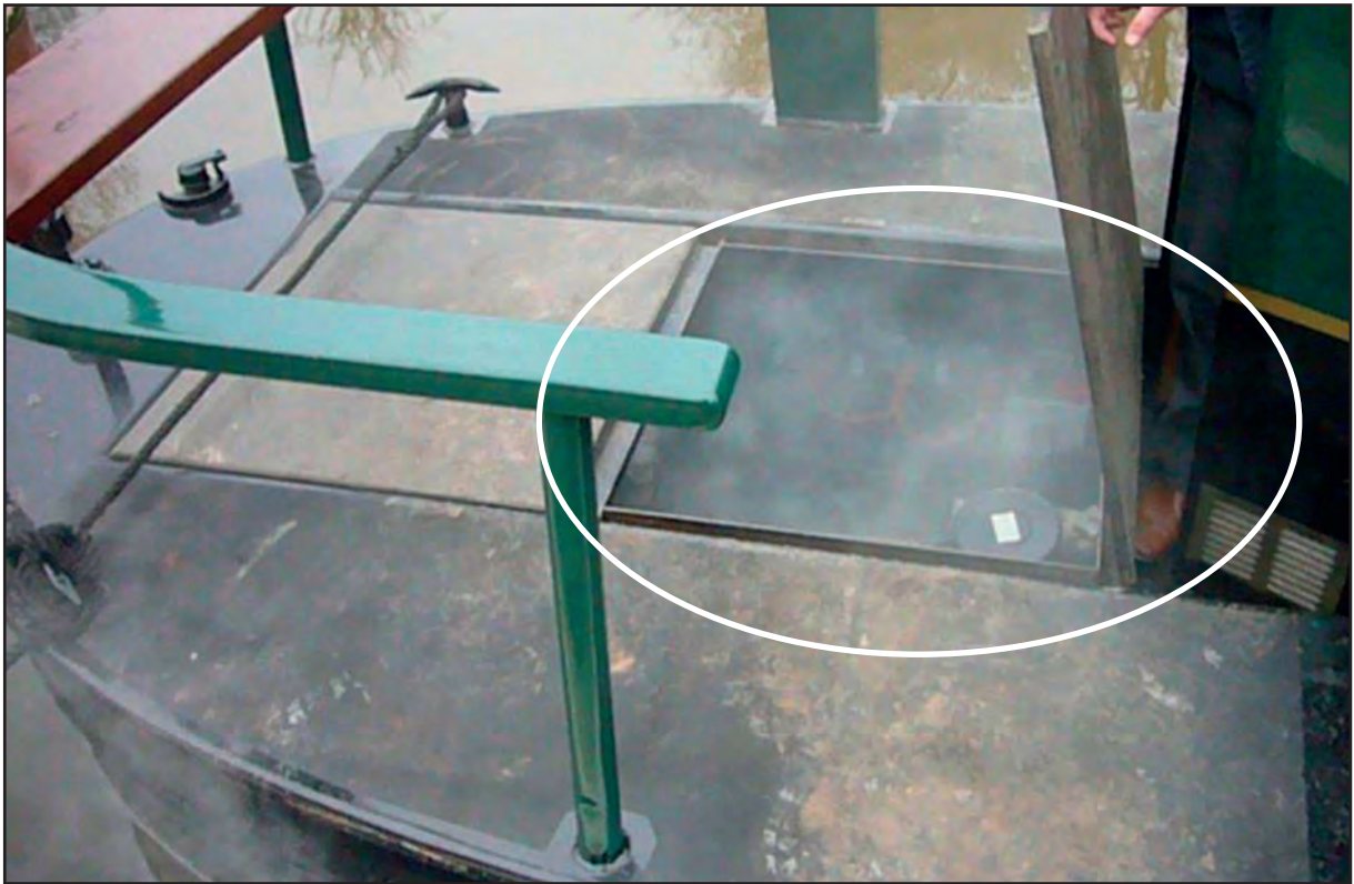
Figure 2: Smoke-logged engine compartment
