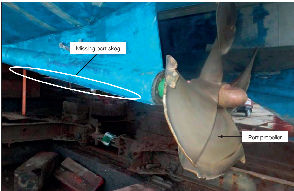
Figure 3: Missing port skag and port propeller blade damage
