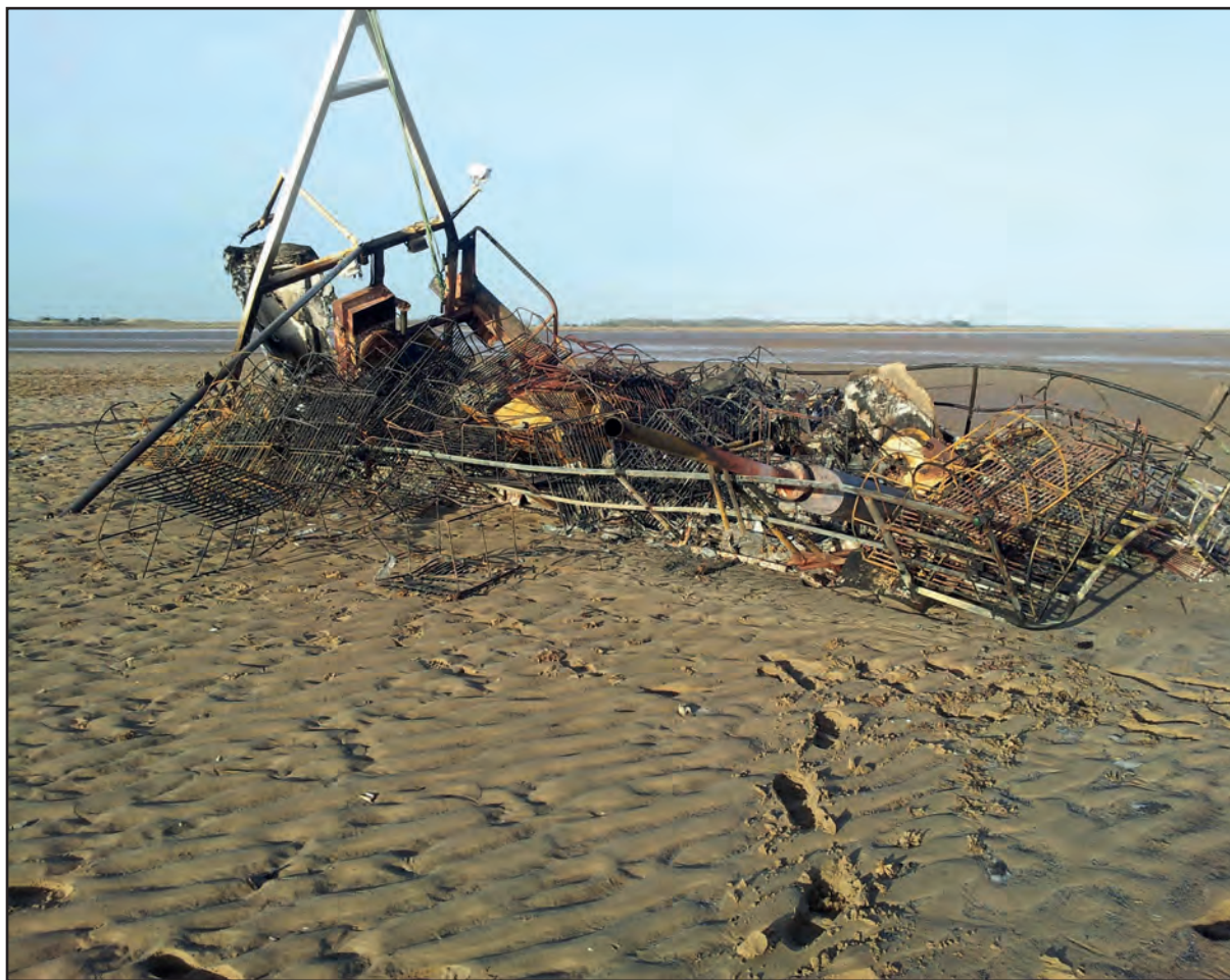
Figure 2: Burnt out wreck of the fishing vessel (view from port side)
