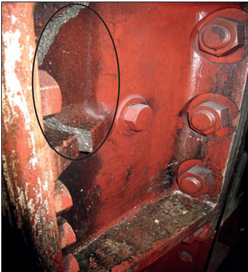
Figure 2: Gearcase middle section crack
