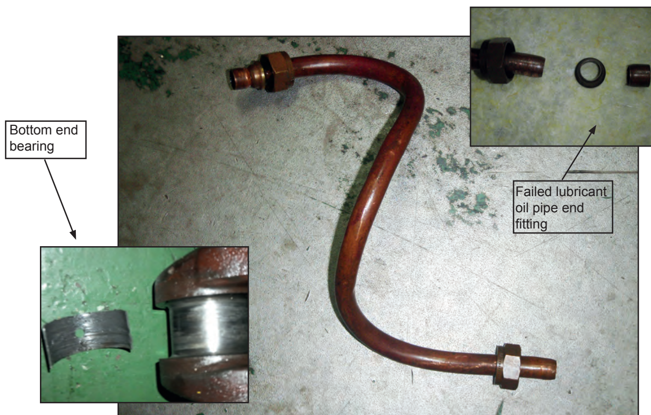
Damage to lubrication oil pipe and bottom end bearing
