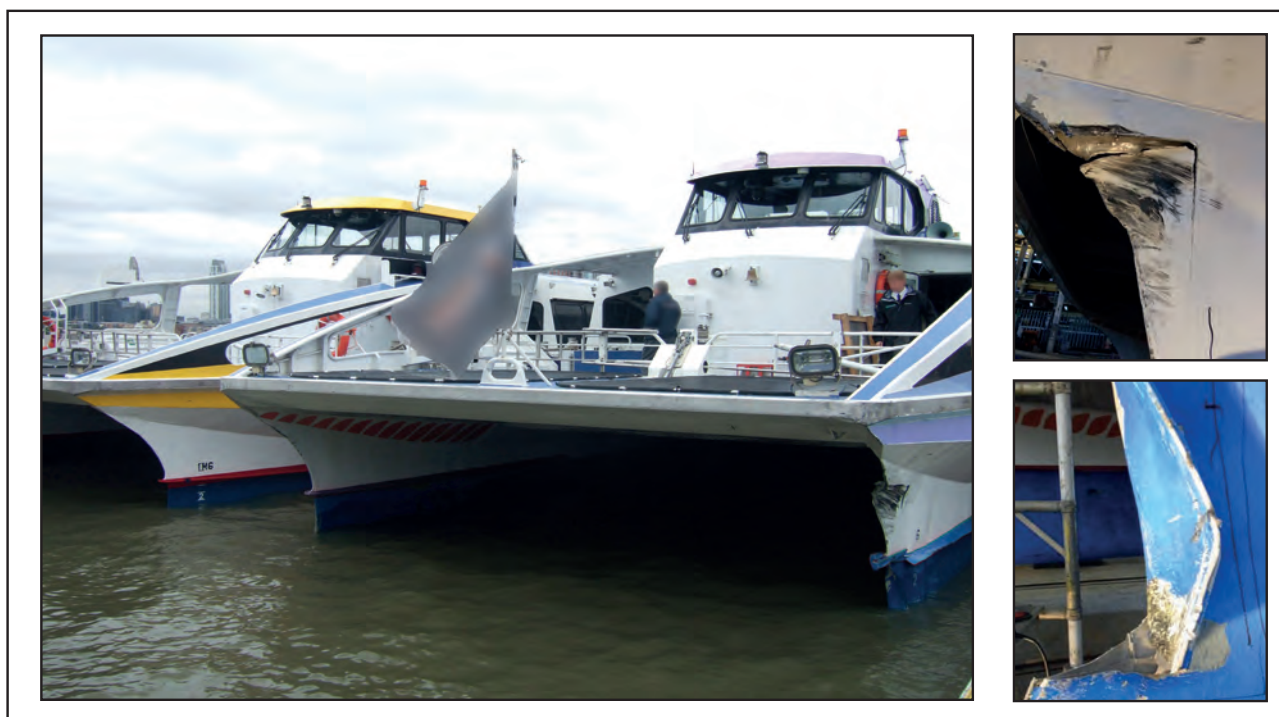
Figure 1: Hull damage caused by contact
