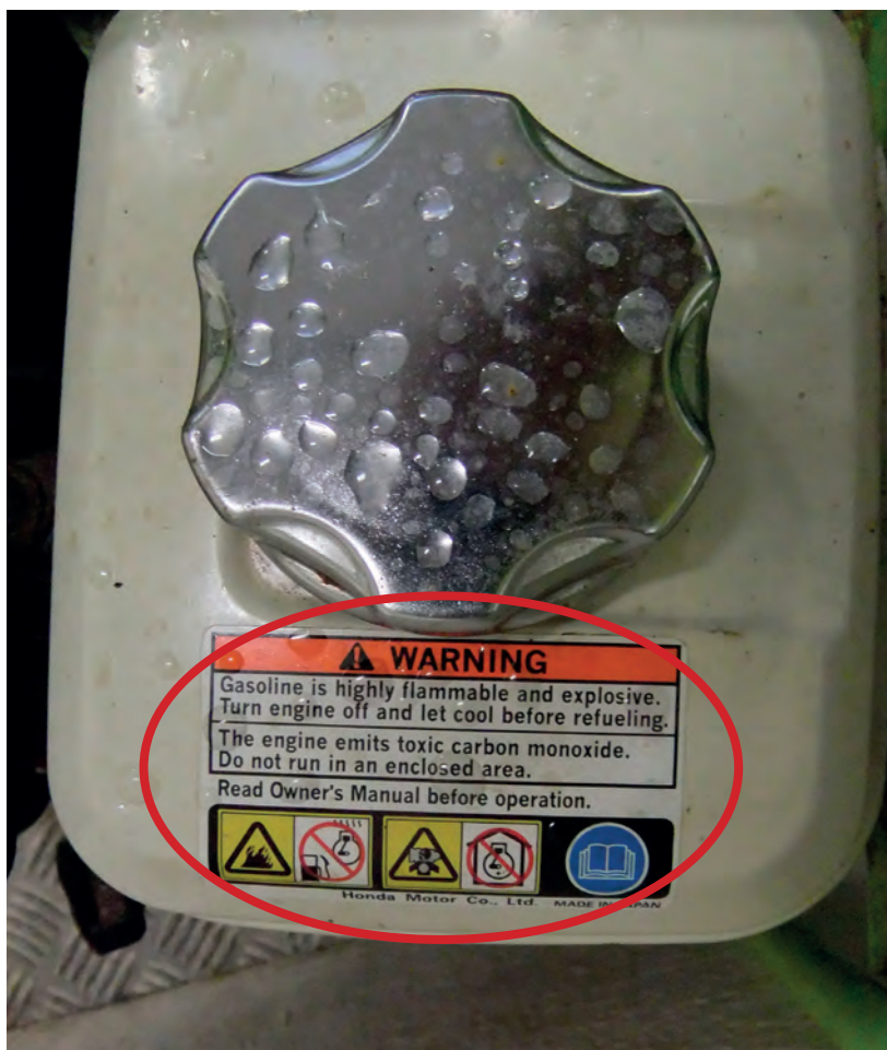
Figure 2: Warning notice on the petrol tank
