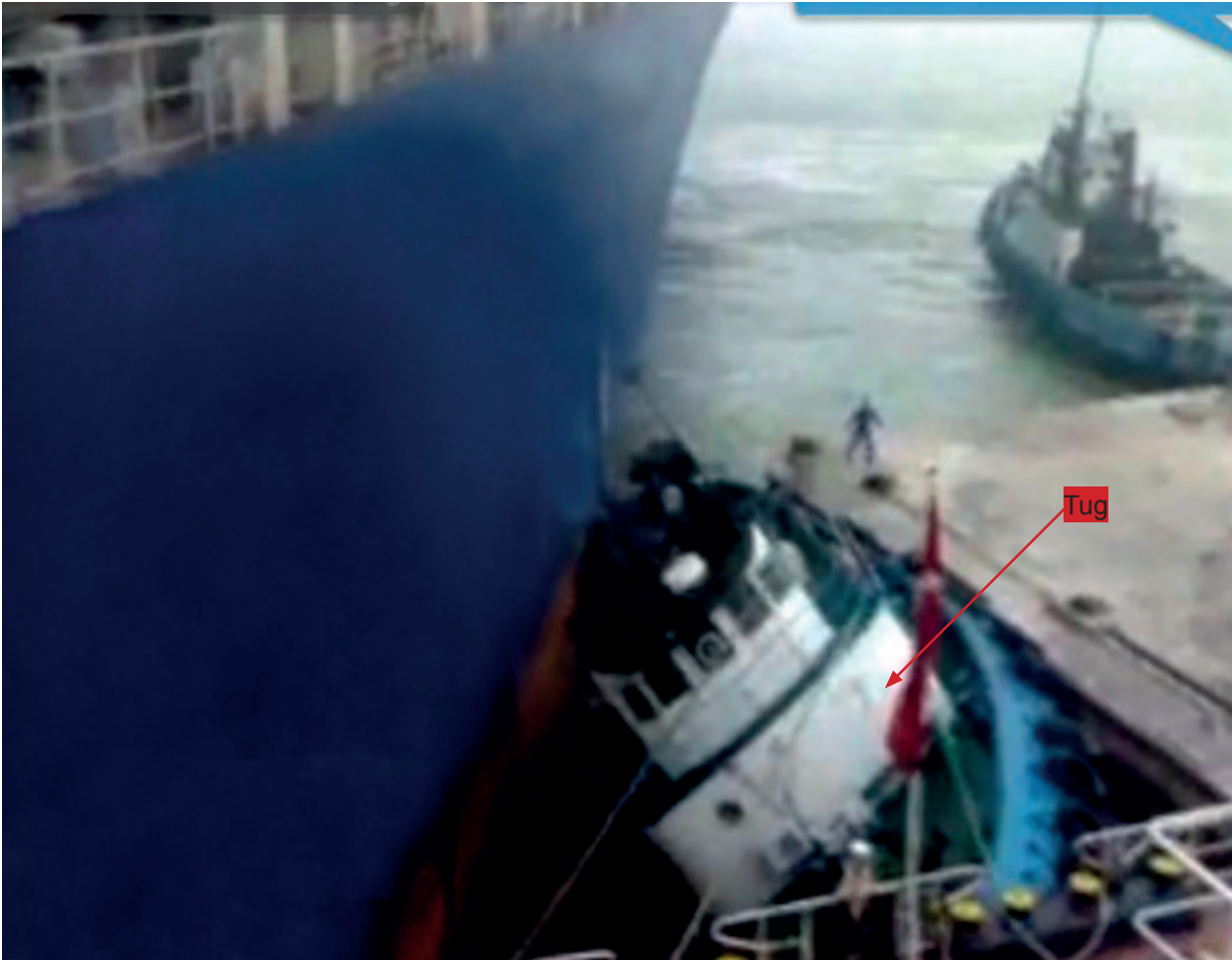
Figure 5: Tug trapped between vessel and quayside
