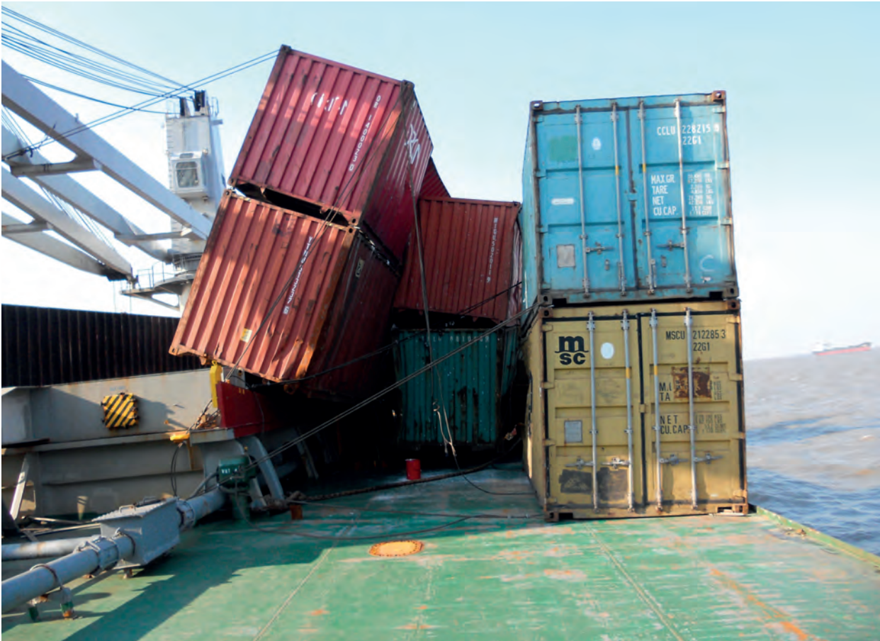
Figure 3: Some of the loose containers that remained on deck
