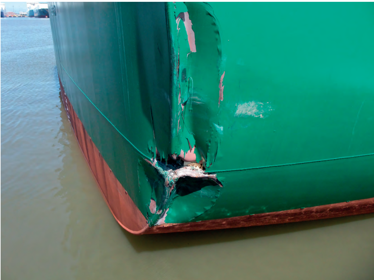
Figure 2: Damage to the vessel's stern
