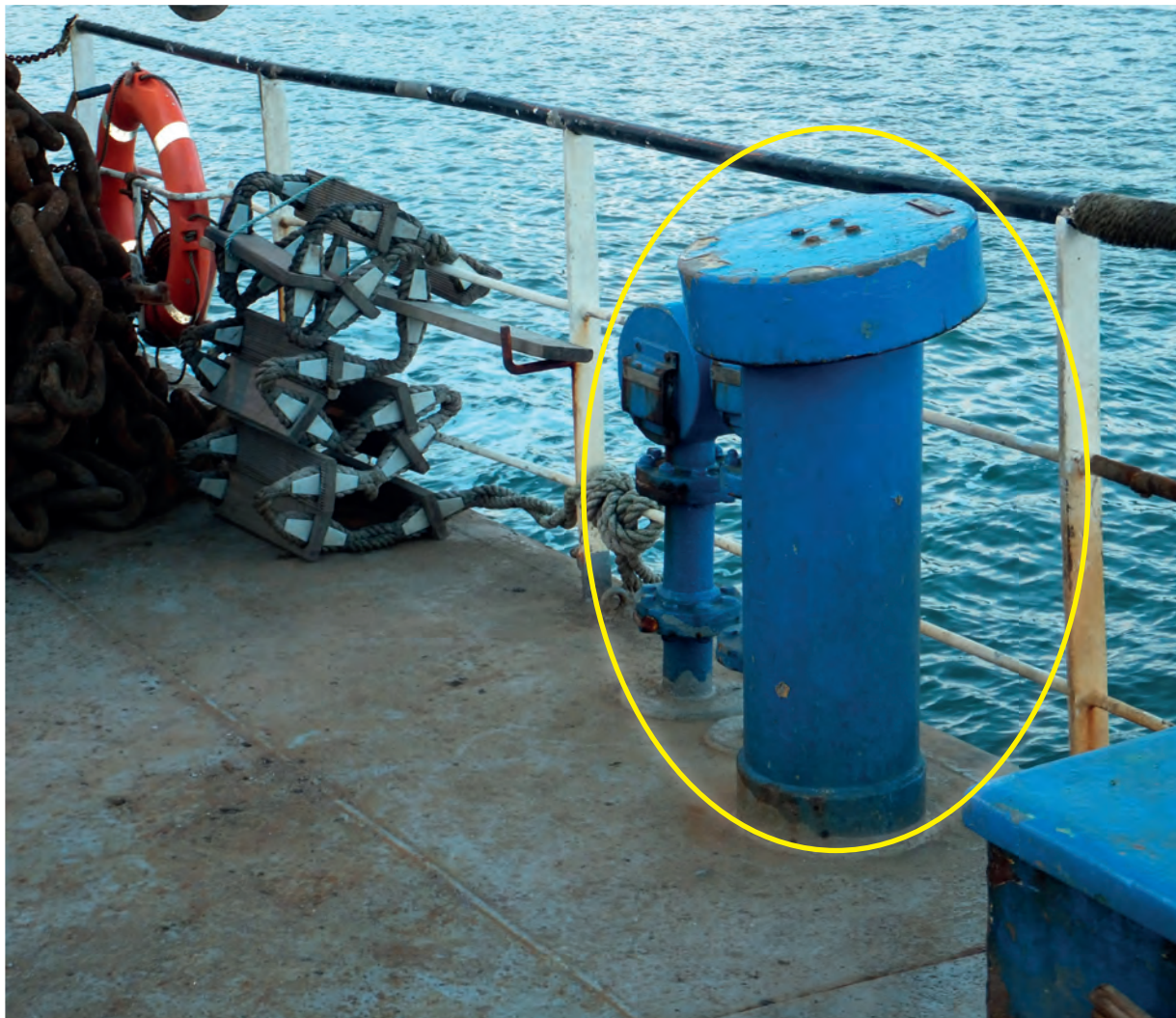
Figure 1: The mushroom vent and mooring chain
