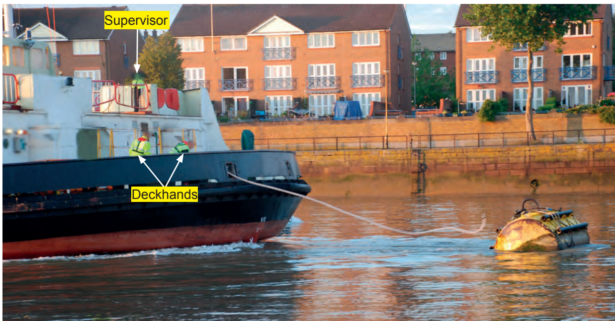
Figure 1: Typical slip rope recovery from the mooring buoy
