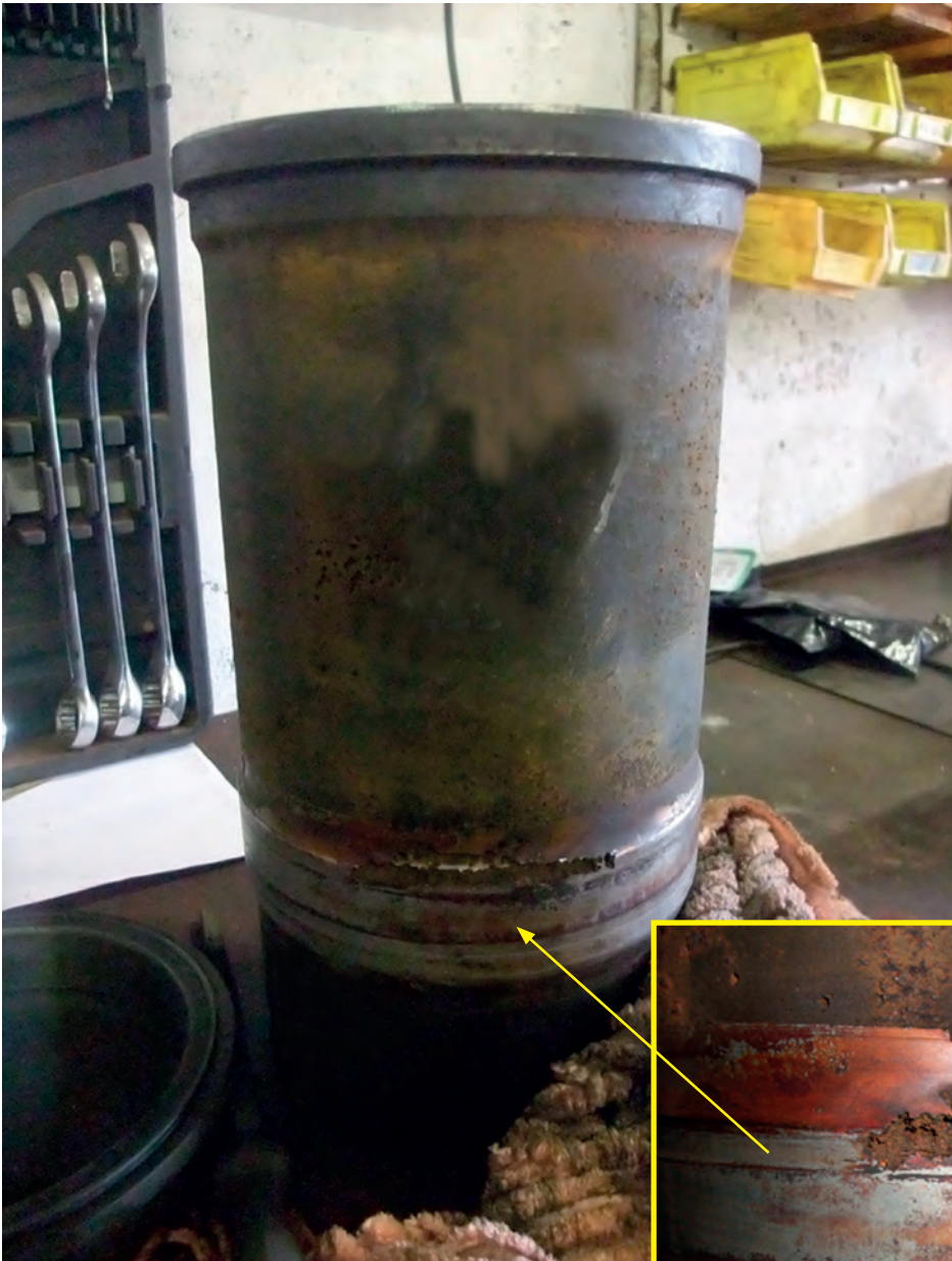
Electrolytic corrosion on vessel's cylinder liner
