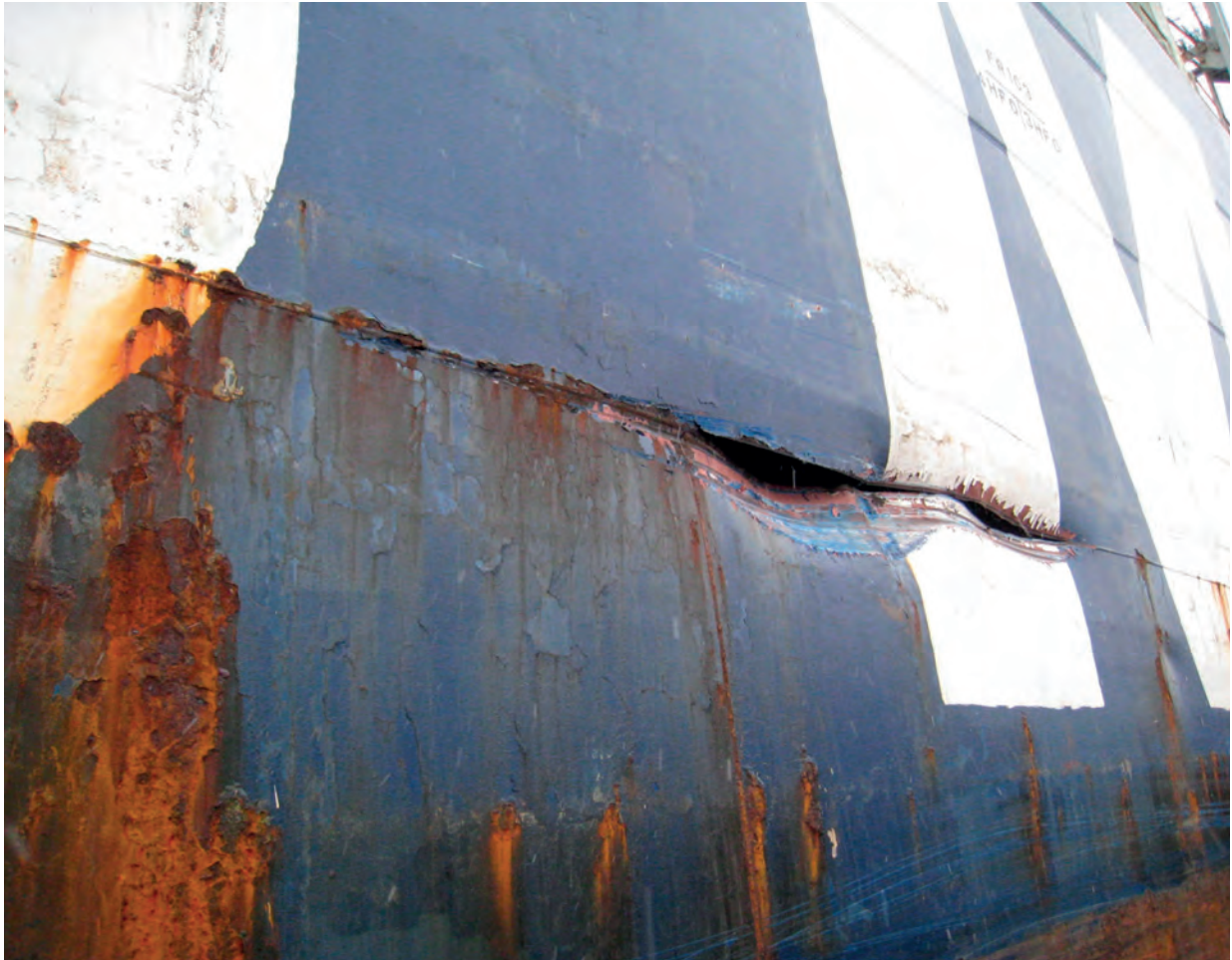
Figure 4: Hull damage to container vessel
