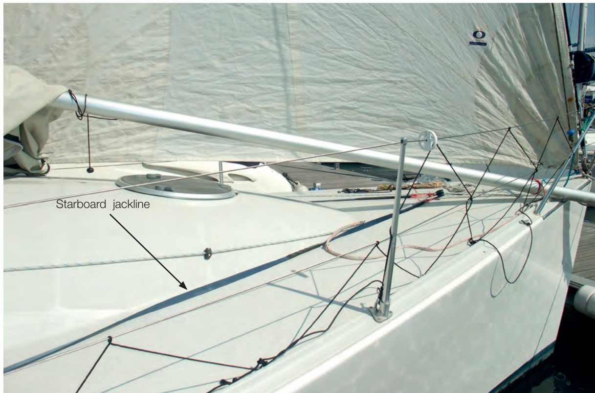
Figure 2: Tether connected to the starboard jackline
