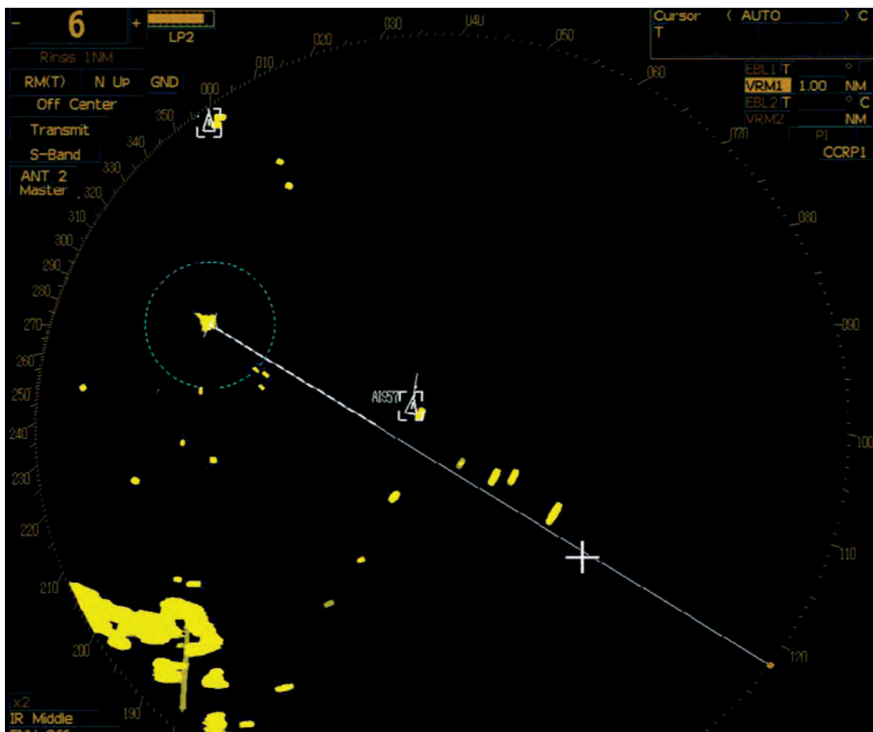
Radar display showing three fishing vessels on the starboard bow at 1 mile range
