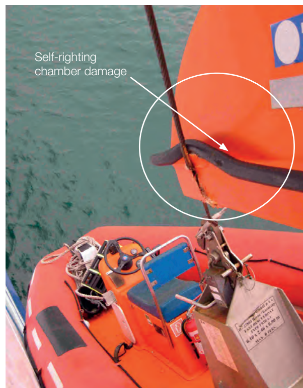
Figure 2: Winch wire snagging self-righting chamber
