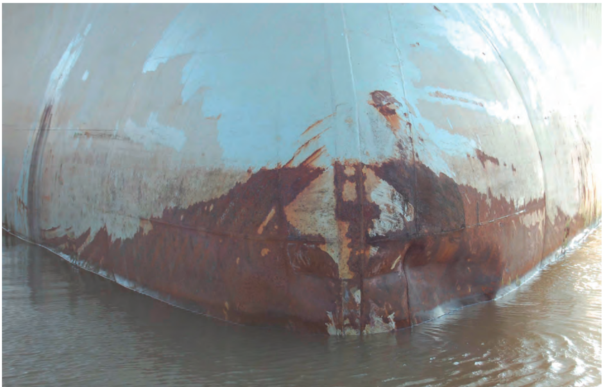
Figure 2: Damage to vessel's bulbous bow
