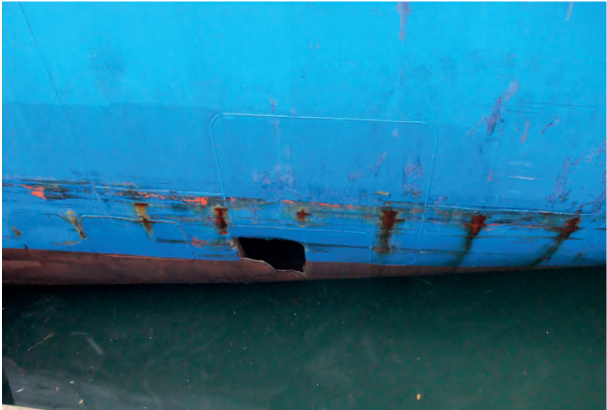
Figure 2: Hull penetration damage to the ship
