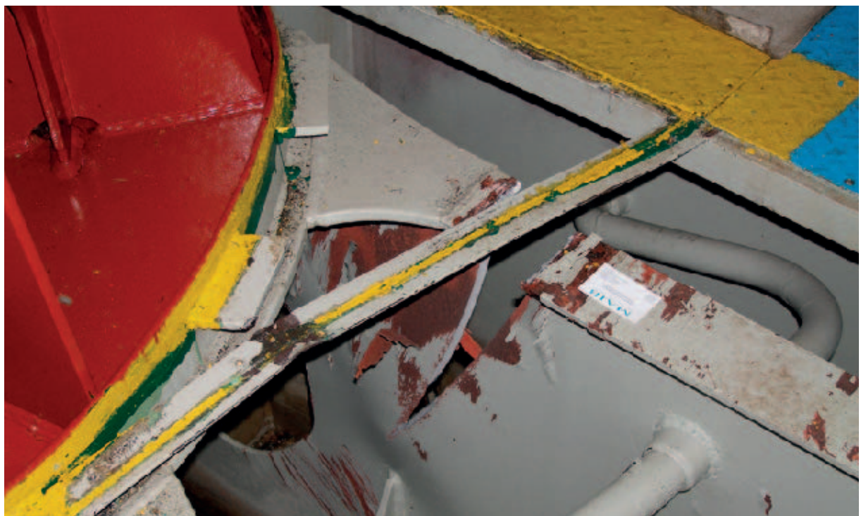
Figure 2: Damage to steering compartment
