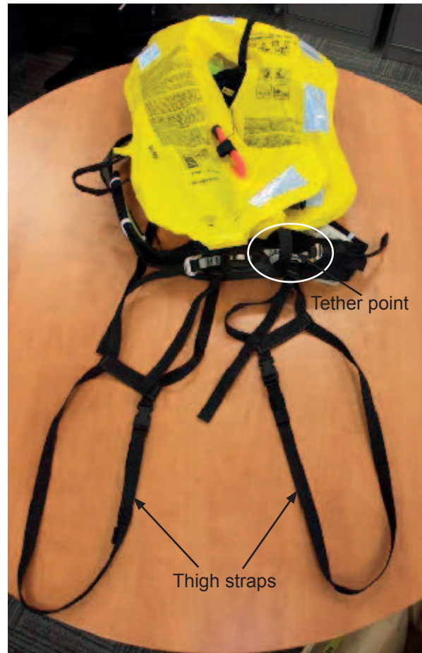
Figure 1: Lifejacket showing harness and thigh straps
