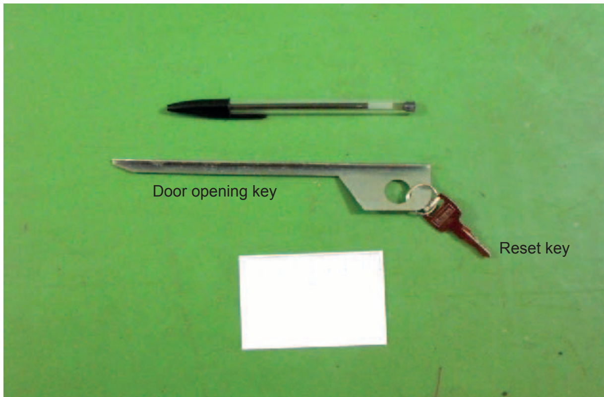
Figure 3: Lift door opening key and lift reset key
