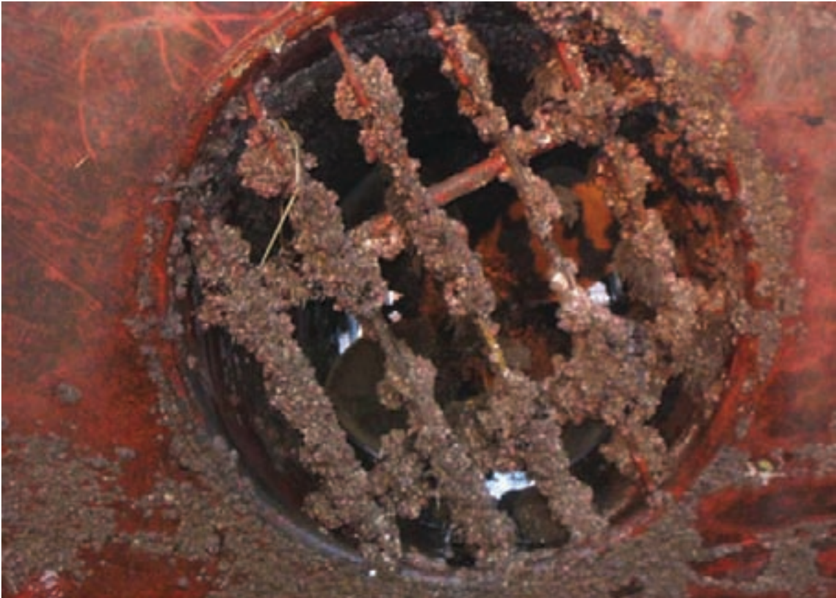
Figure 3: Mussel and barnacle fouling of an inlet grid
