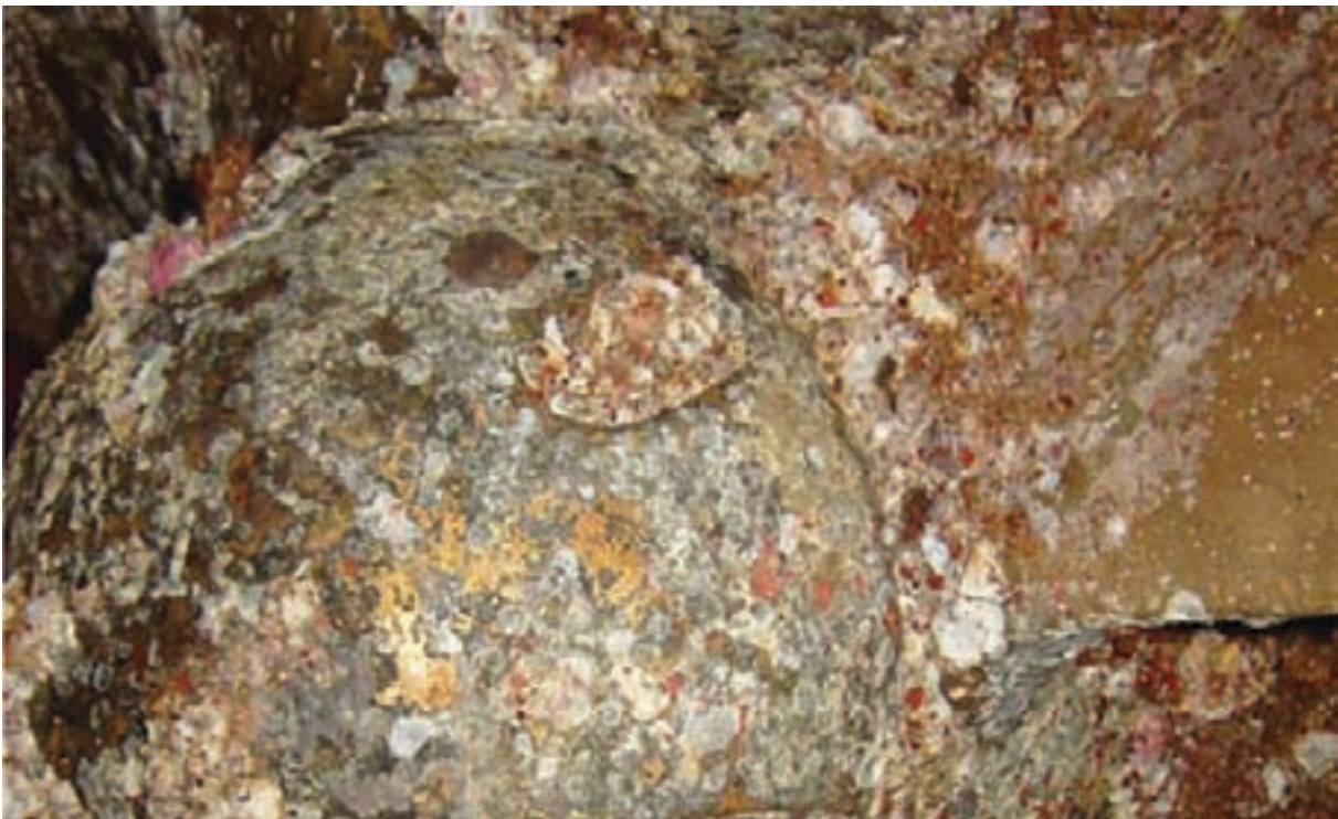
Figure 4: Fouling of the propeller blade
