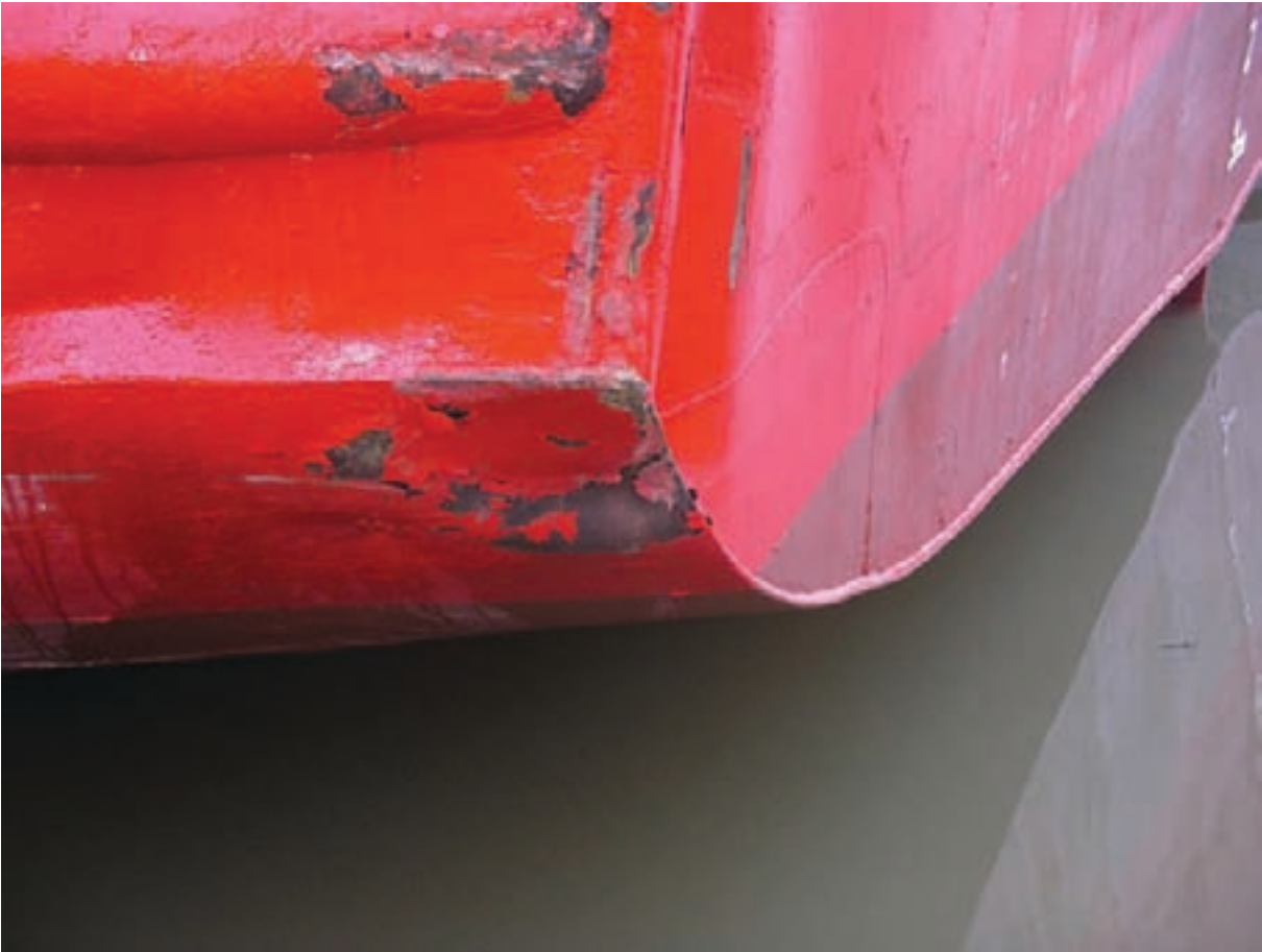
Figure 2: Damage to the coaster's port quarter
