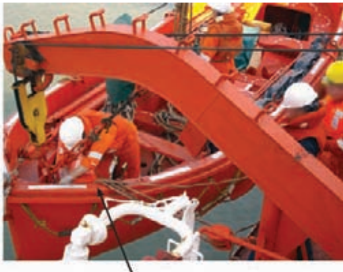
CORRECT Bowsing-in gear fitted before releasing tricing pennant
