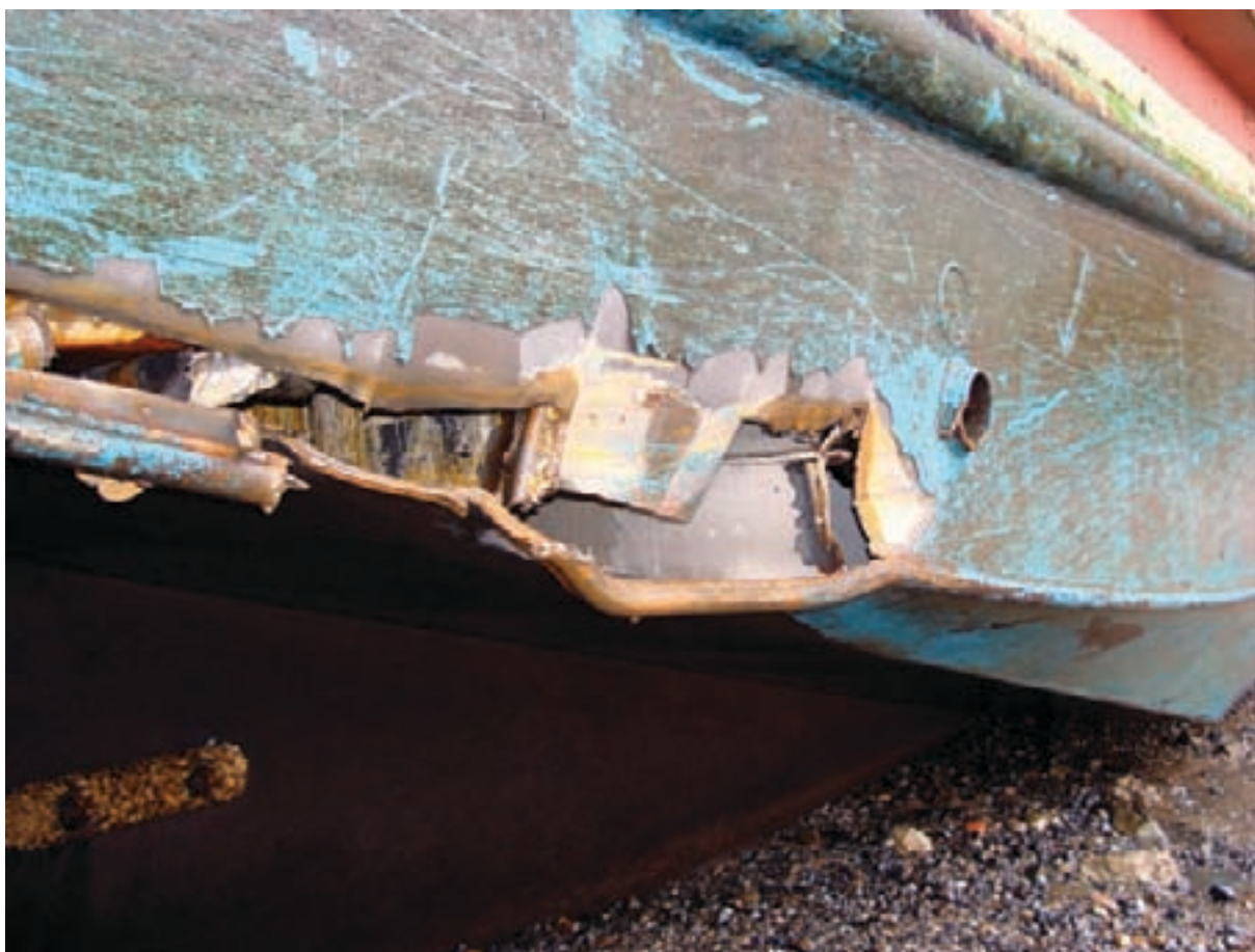
Figure 1: Damage to vessel's starboard pontoon
