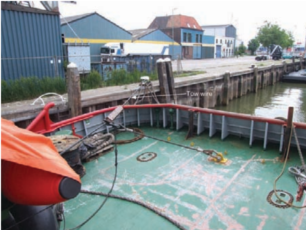
Figure 3: View of tow wire in approximate position after shackle jumped
