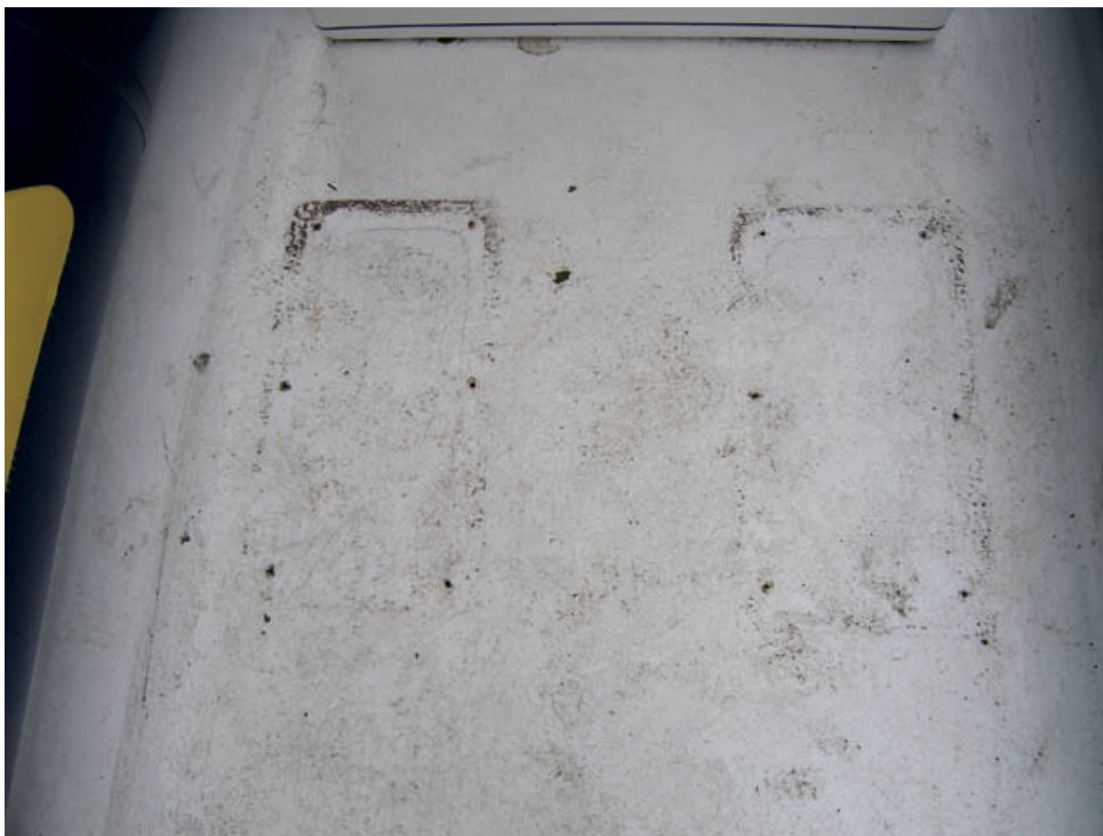
Vessel's deck showing outline of consoles – note lack of deck preparation and adhesive
