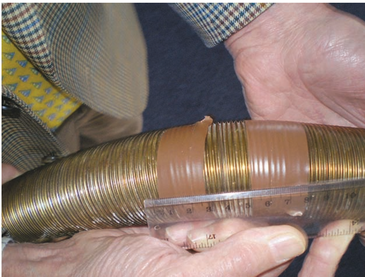
Heater exhaust pipe with crack indicated at the 4cm mark on the ruler
