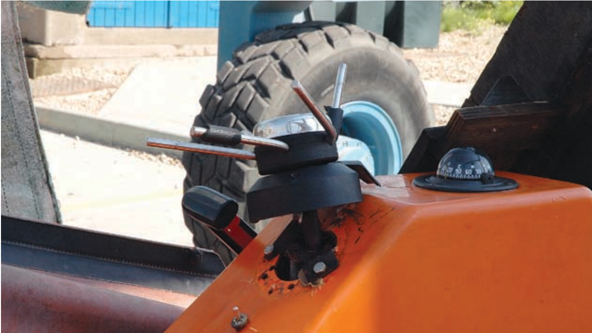
Damage to steering wheel following impact of the skipper
