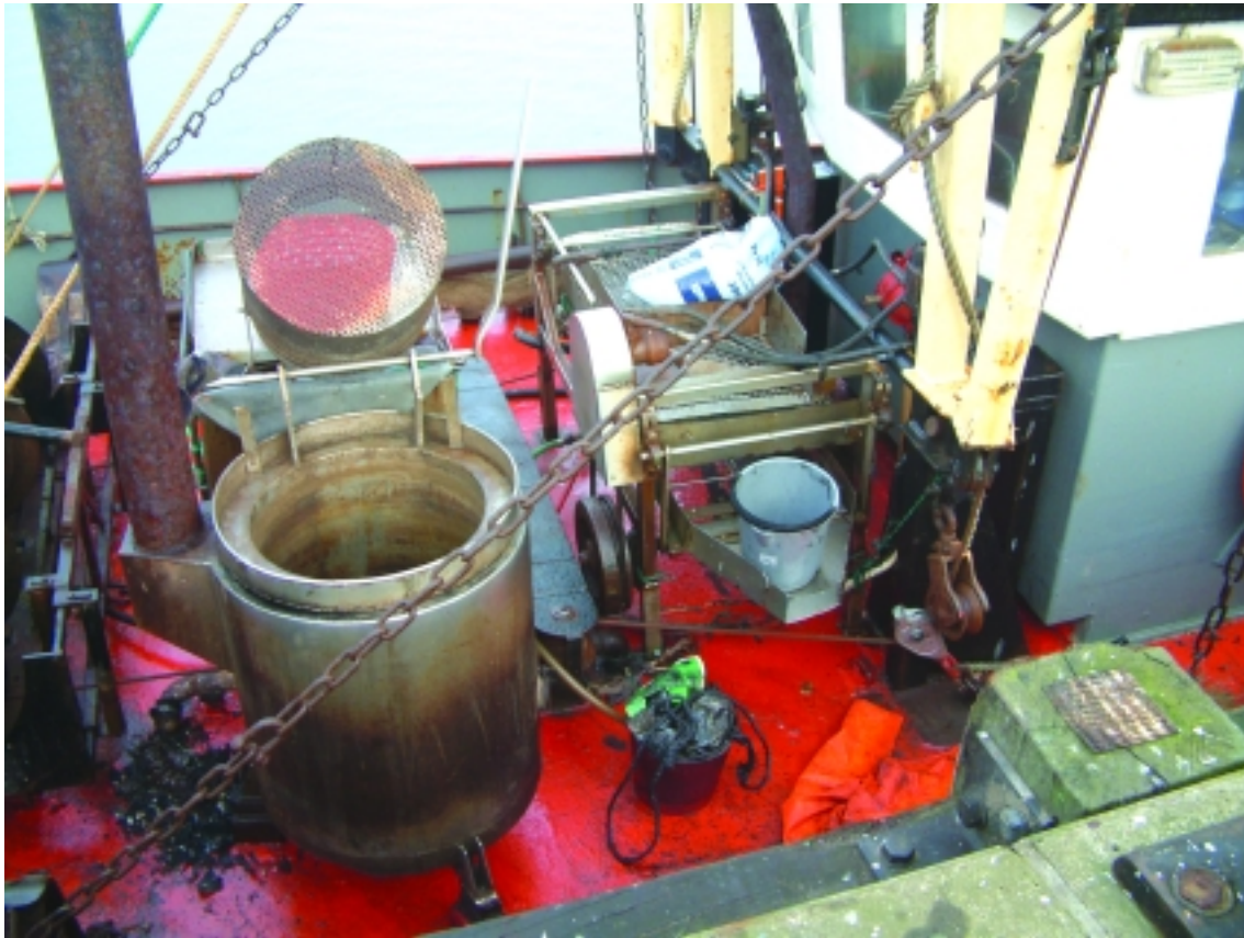
Figure 2: Shrimp boiler after the fire, with melted air supply pipe
