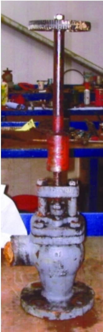
Vessel's eductor system valve
