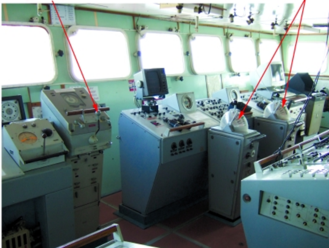
The bridge showing the telegraph and steering positions
