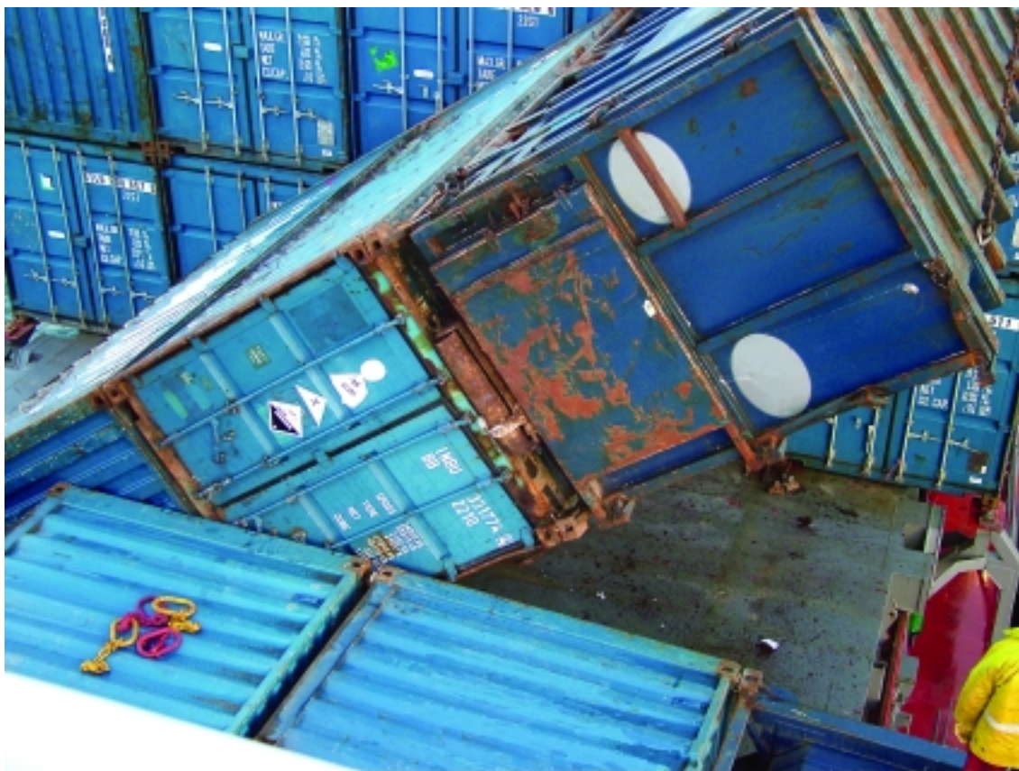
Remaining containers being lifted by crane after collapsing on deck
