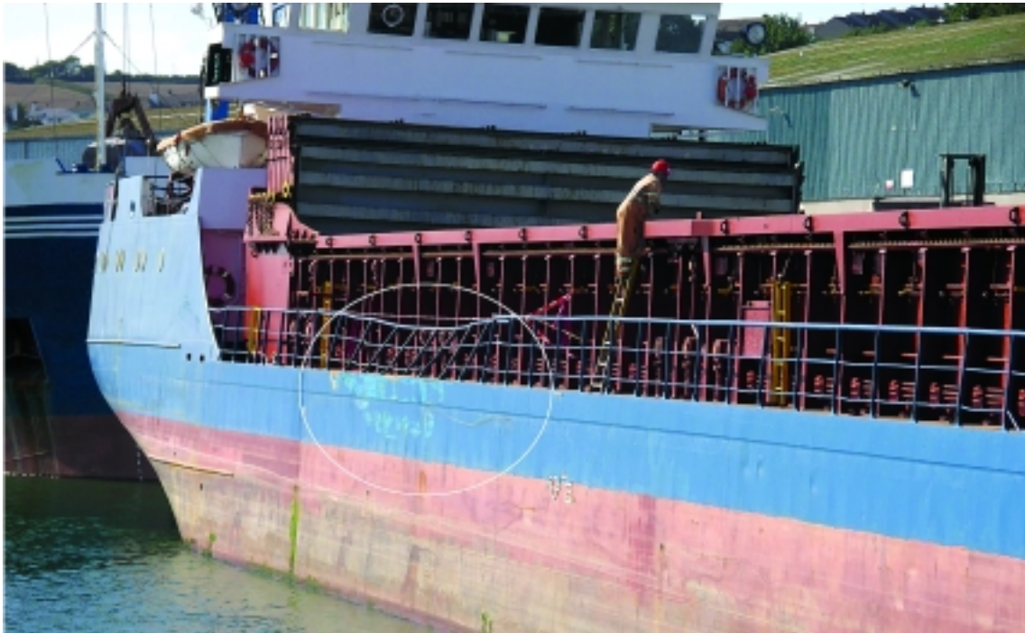
Damage to the starboard side of the ship
