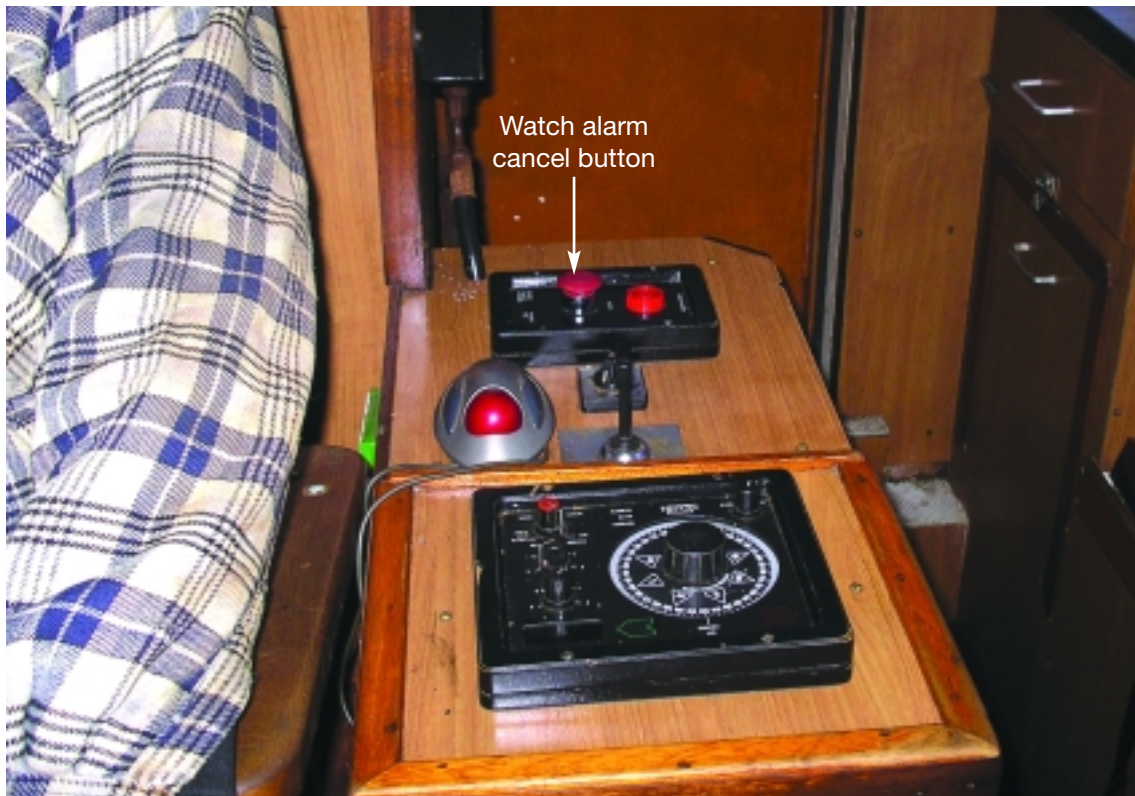
Figure 1: Vessel's watch alarm cancel button, next to the crewman on watch
