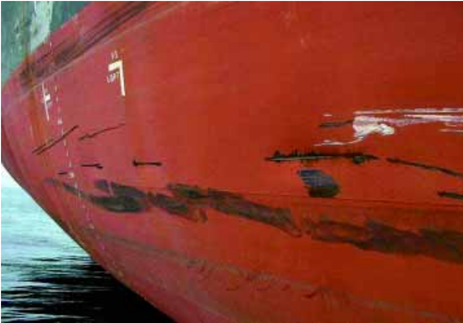
Shell plating damage on ore carrier
