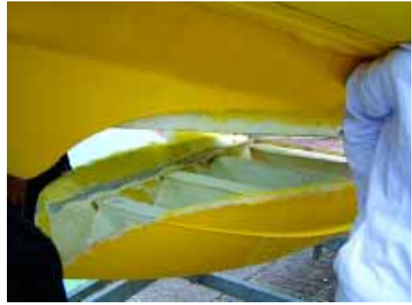
Figure 3: Hull lifted to expose split
