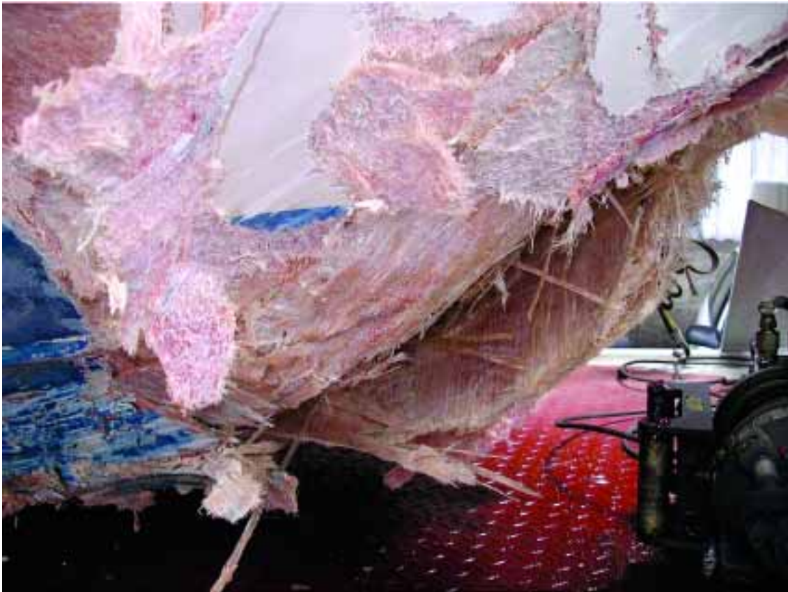
Damage to starboard forefoot and bow forward
