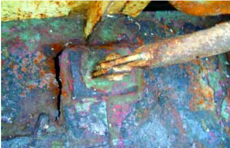
Figure 2: A frame supporting frame to deck split
