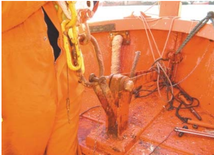
Figure 3 Full blocks chain ring incorrectly positioned over safety pin
