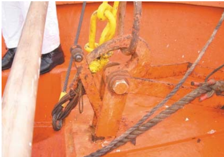
Figure 4 Forward hook assembly showing damage
