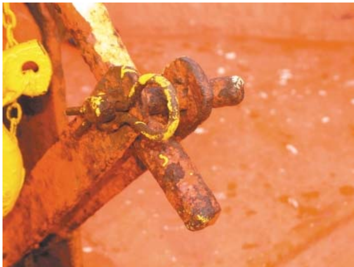
Figure 2 Detail showing hook in the secure position with the safety pin and 'R' clip in place
