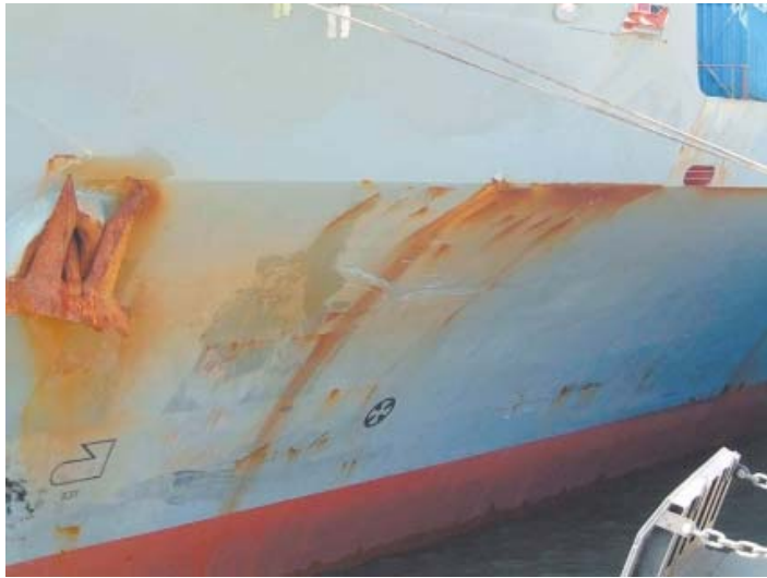
Damage caused by impact
