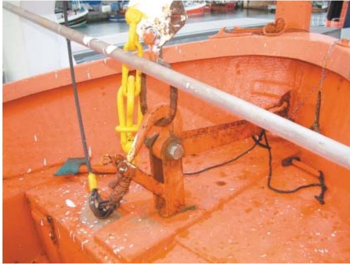
Figure 1 Lifting hook showing fall block chain ring correctly secured
