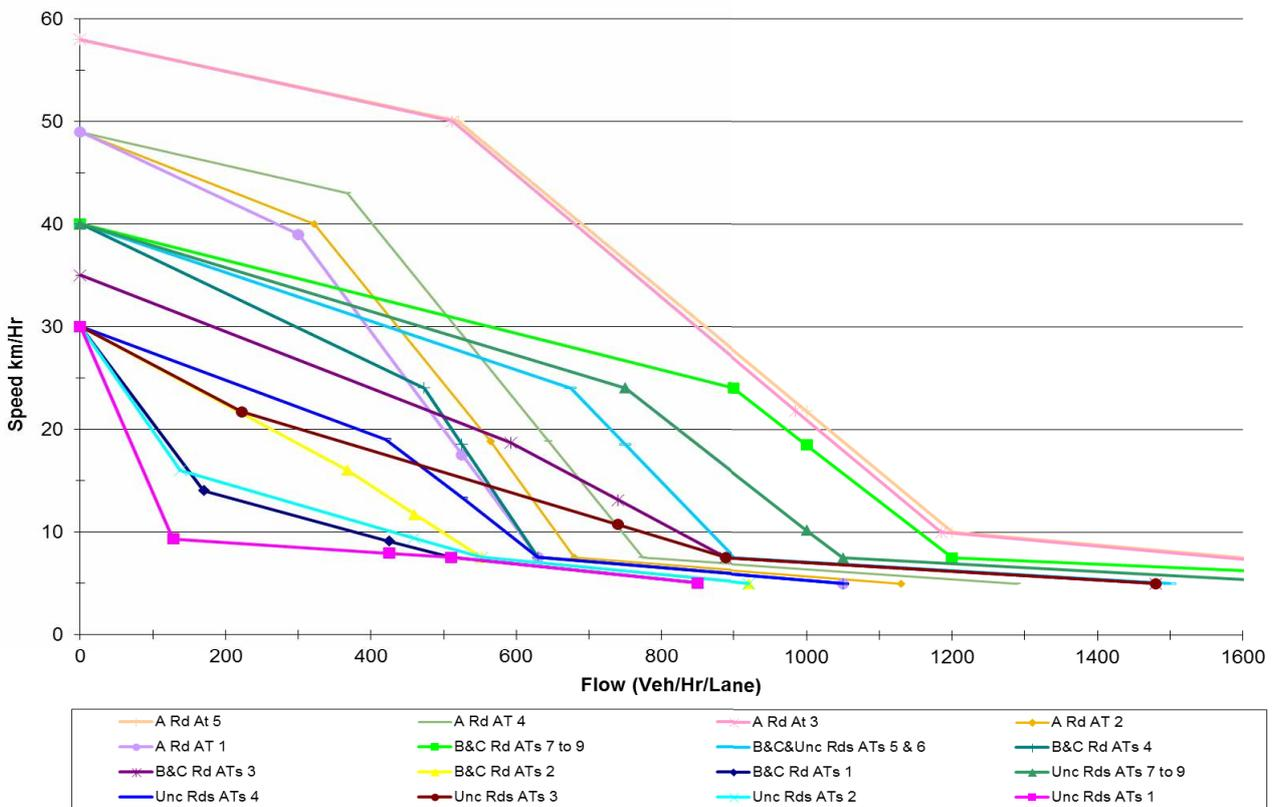
Figure 49: Urban Minor Road Speed Flow Curve
