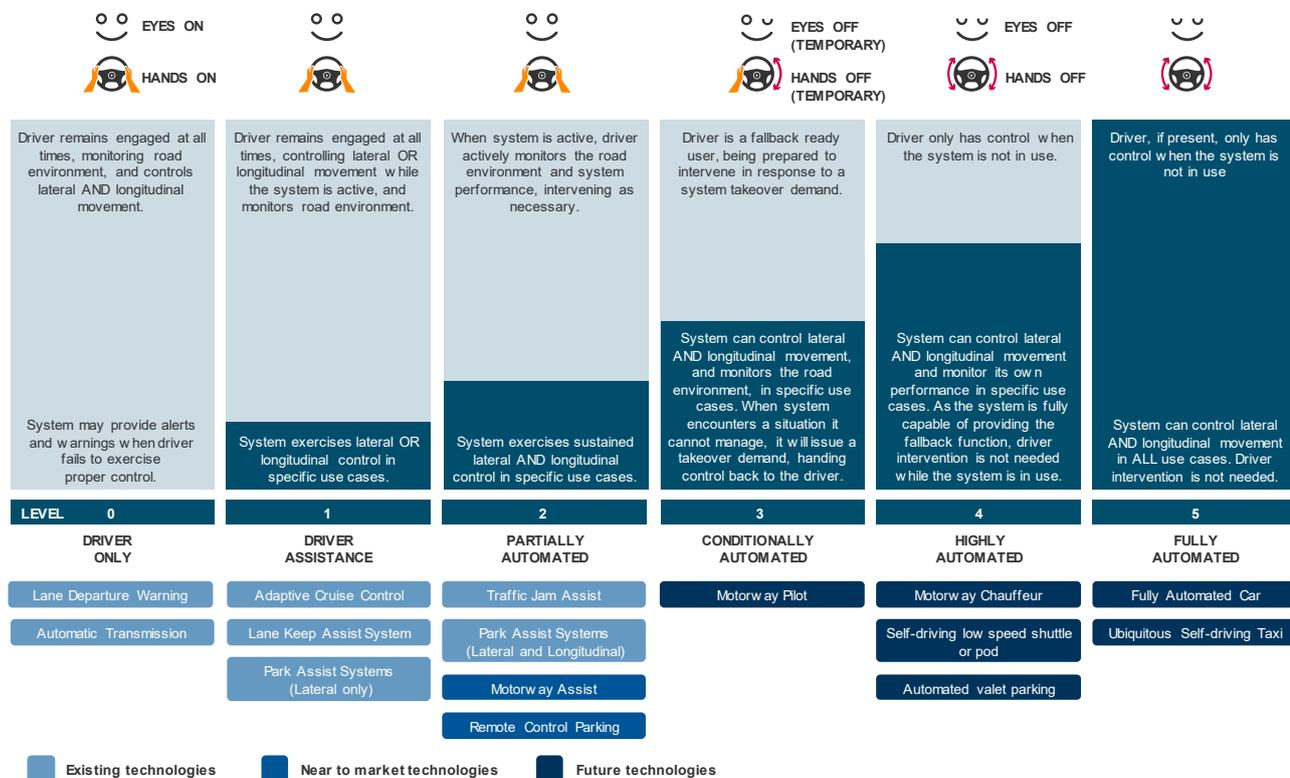
Figure 43: Society of Automotive Engineer (SAE) Levels
