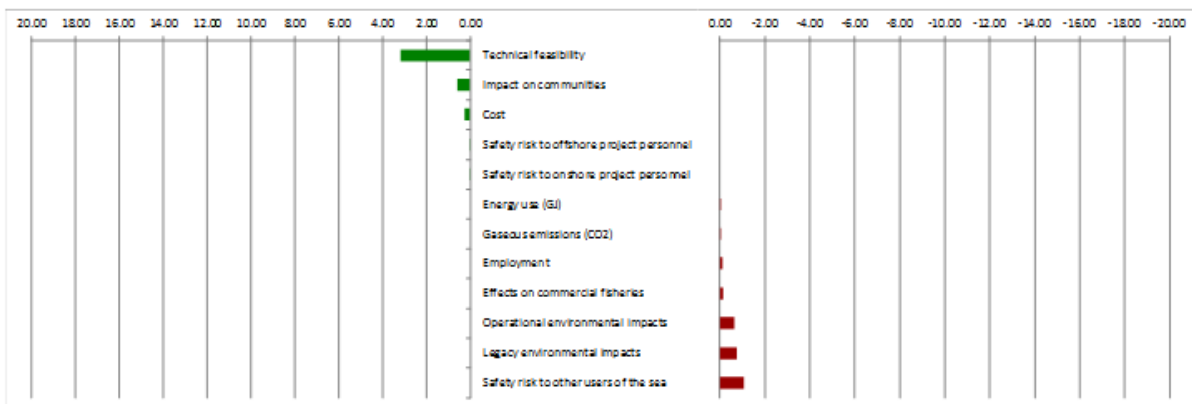
Figure 13 Difference Chart Comparing the Weighted Scores for Each Sub-criterion of Option 5 'Rock-dump Whole Length' with Option 6 'Recover Whole Length by Cut and Lift', under the Standard Weighting, for Pipeline PL050/N0401.
