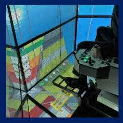
A state of the art training and technology suite at the Port of Tilbury includes two training simulators provide a full, 360-degree experience, of major crane and straddle operational equipment. This provides operators with an enhanced learning environment featuring industrial controls and realistic working terminal scenarios.
