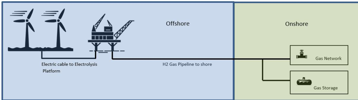
The centralised offshore electrolysis design option provides an intermediate cost option across all distances.
