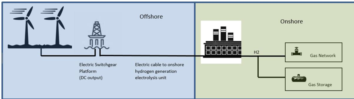
Centralised onshore electrolysis provides the highest cost option for the development of hydrogen at all distances, with costs increasing with distance from shore.
