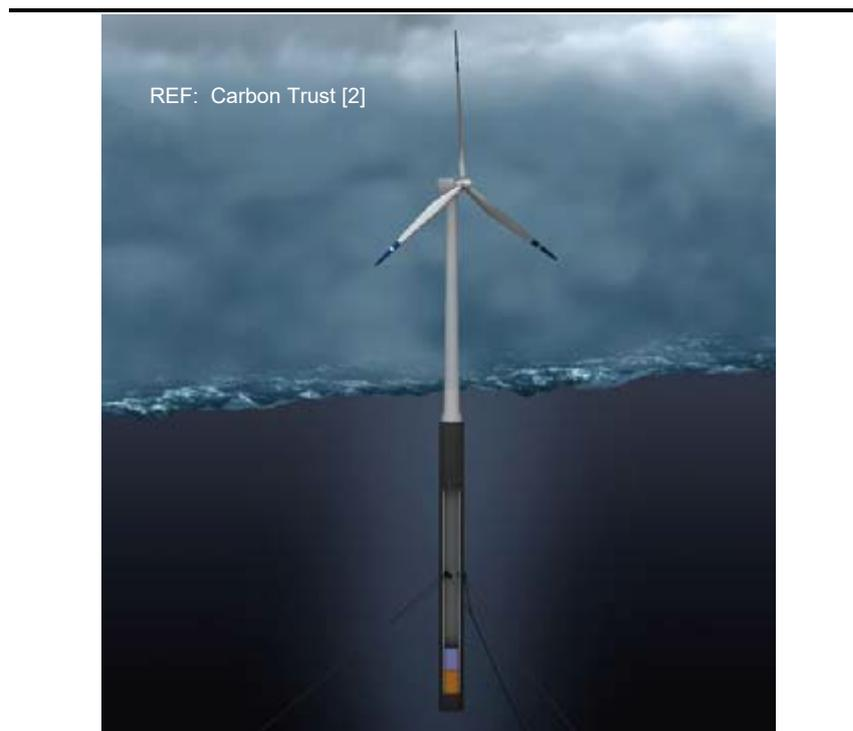
The design comprises an extension on the main turbine tower vertically oriented downwards with ballasting in the sub-structure to provide stability. The design has been proven to work at a 2.3 MW scale in Norway, and at 6 MW scale in the UK North Sea (5 x 6MW units deployed on the Hywind project offshore Aberdeen).
