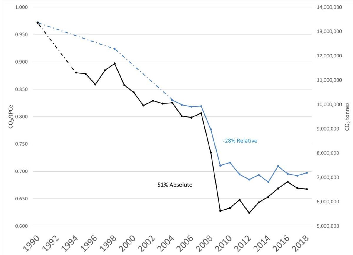
Figure 2.5: Reduction in Absolute and Relative Emissions from UK Cement Manufacture 1990 - 2018
