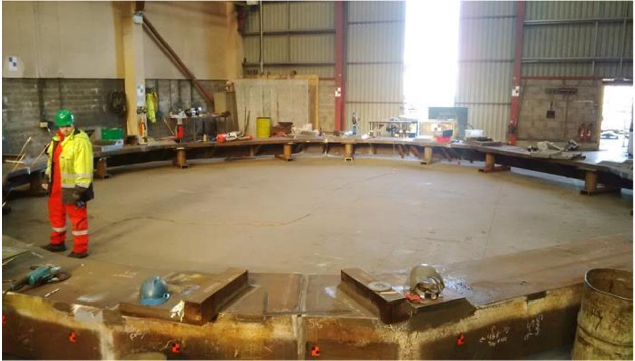
Figure 11. Shear Restraint Fitted inside a Leg on Brent Delta.
