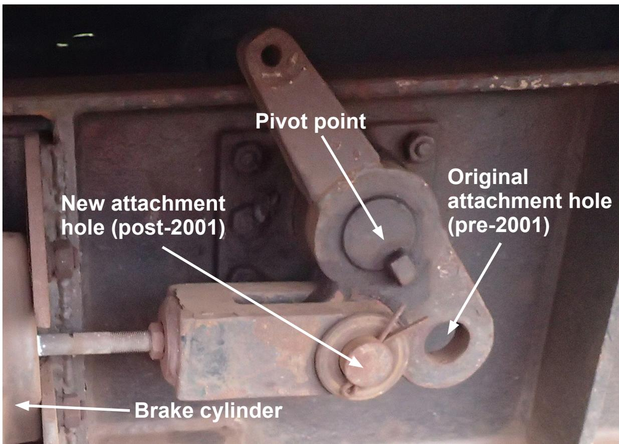
Figure 8: The original and new (2001) brake cylinder attachment positions
