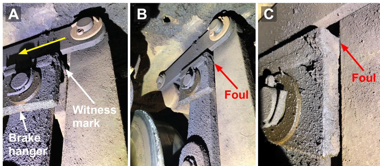
Figure 7: Photographs showing the location of the foul in the brake linkage (red arrows), (a) with brakes off; (b) with brakes on and (c) close-up view with brakes on. The yellow arrow in (a) indicates the movement of the link when the brakes apply.
