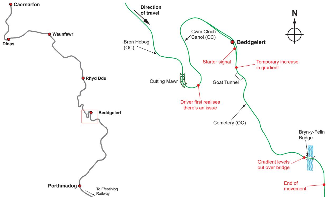
Figure 2: Geographical overview of the Welsh Highland Railway route, and (right) detail of the area in which the runaway occurred.
