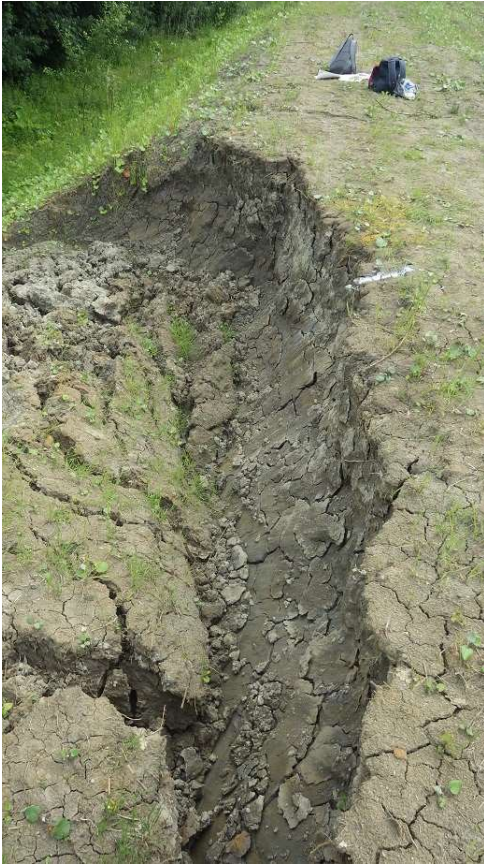
Photo 1: One of 3 slip failures in the outer shoulder of the embankment
