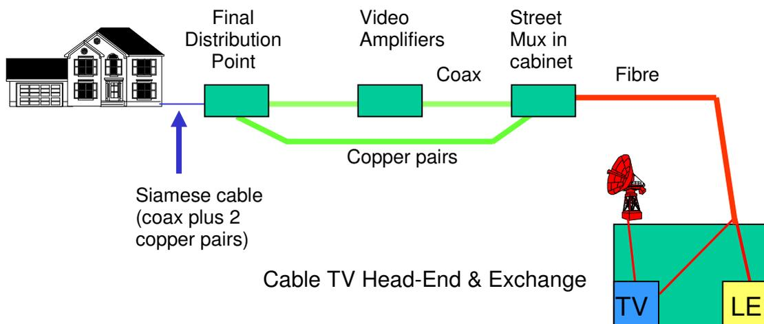
How a telephone call is connected
