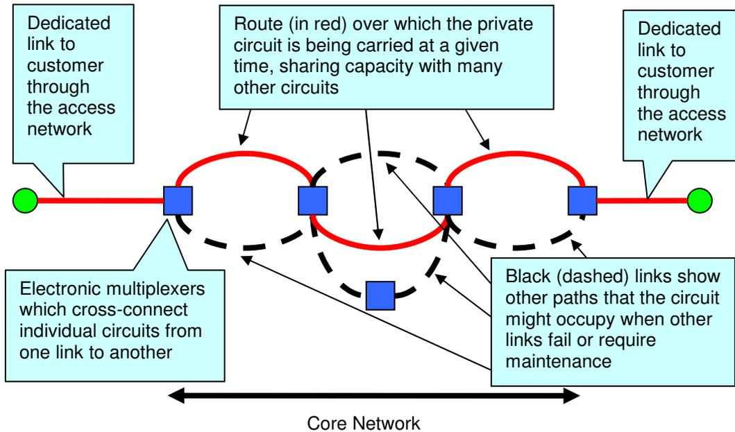
Figure 6: Typical arrangement and routing of a Private Circuit
