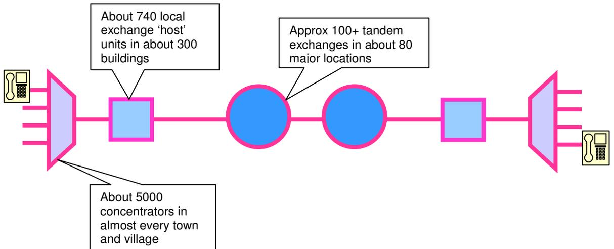
Figure 5: Telephone network architecture
