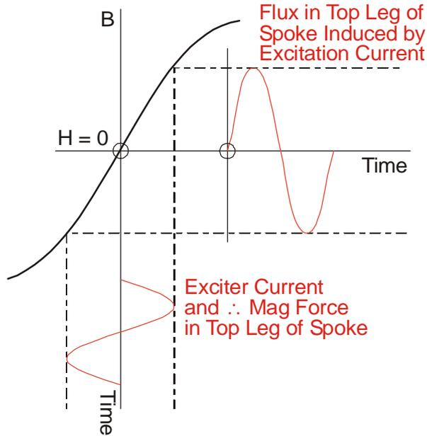
18. Now considering the bottom leg only; the flux induced in this leg by the excitation current will at any instant be in the opposite direction to that induced in the top leg, i.e. the flux in the bottom leg is 180° out of phase with the flux in the top leg as shown in Fig 8.
