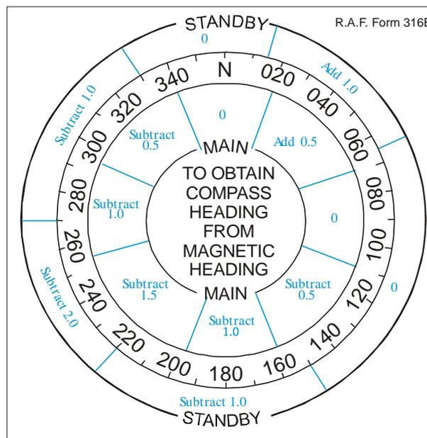
20. **Documentation.** It is important to remember that the compass swinging process is part of an engineering procedure and, as such, must be documented and recorded in accordance with relevant orders. The compass swing is not complete until the paperwork is done and the relevant sections of the aircraft documentation signed.
