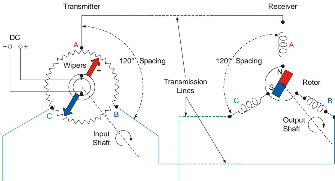
8. **The Receiver.** The receiver (see Fig 2) consists of three high resistance coils whose axes are spaced  $120^\circ$  apart, with a permanent magnet rotor pivoted at their centre carrying a pointer. The three coils are connected to the tapping points A, B, and C in the transmitter.
