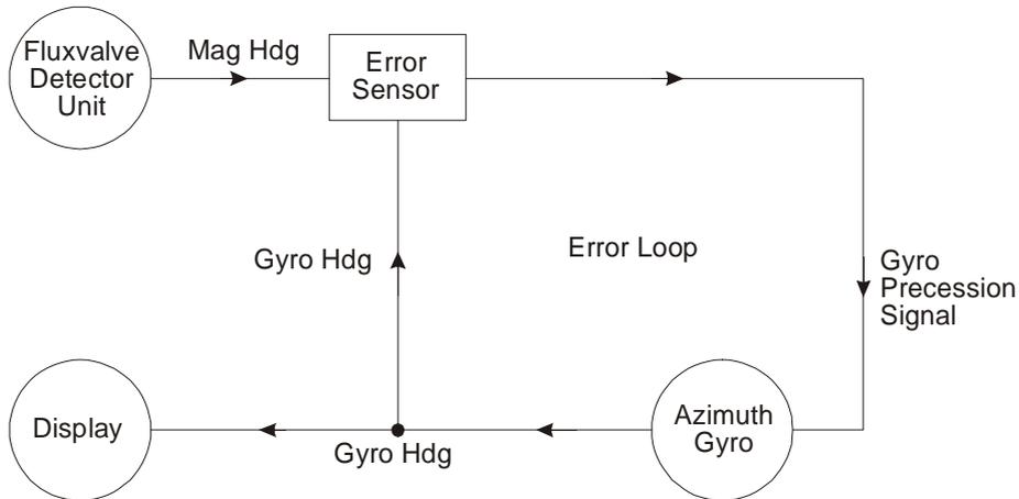
**5-12 Fig 25 Typical Gyro Slaving Mechanization (Simplified Schematic)**
