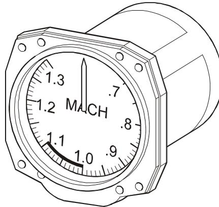
6. The airspeed capsule measures the pressure difference between pitot and static pressure and therefore expands or contracts as airspeed increases or decreases. The movement of the capsule is transferred by the airspeed link to the main shaft, causing it to rotate and move a pivoted arm (the ratio arm) in the direction A-B (see Fig 2).
