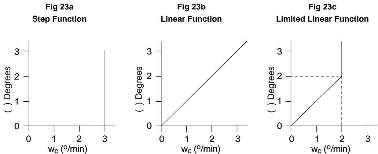
38. The linear correction technique (Fig 23b) appears to be ideal since the correction rate ( $W_c$ ) is proportional to the error signal ( $\epsilon$ ), i.e. for small errors, small torques are applied and vice versa. A problem exists when very large errors occur. For example, modern gyro-magnetic compasses commonly use the random gyro azimuth technique in which the gyro spin axis can point in any
