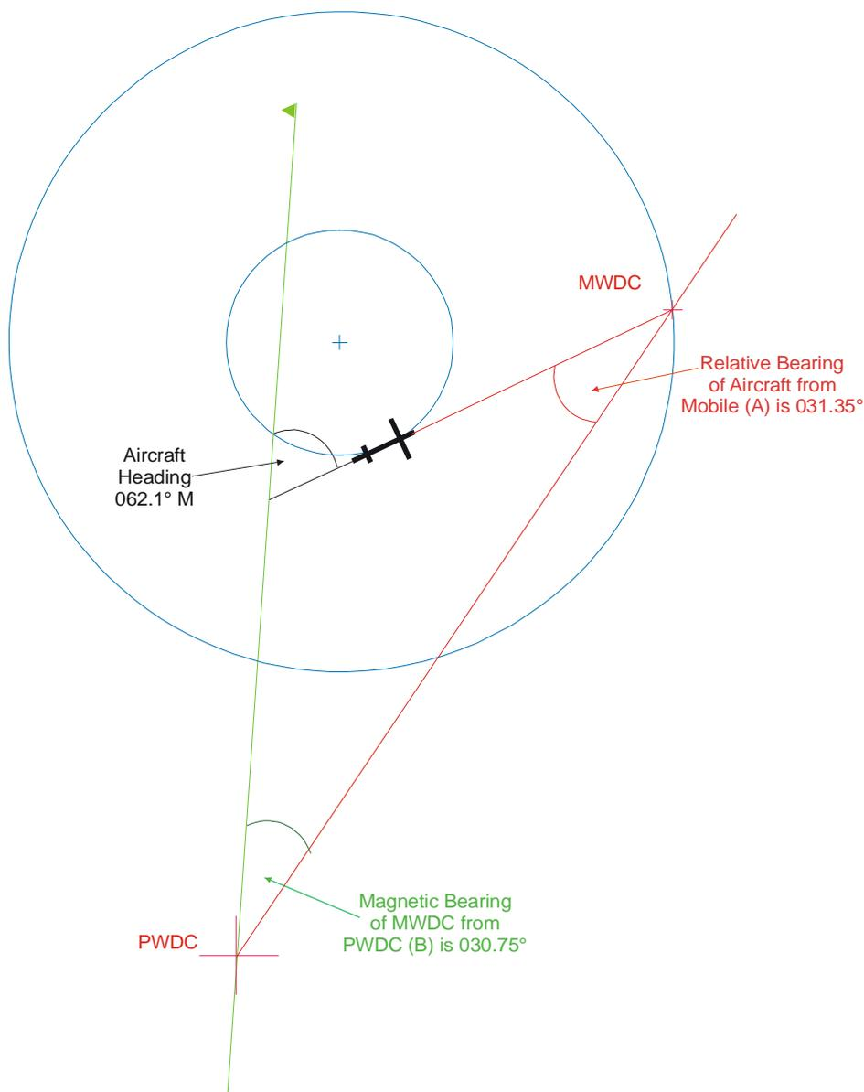
5-18 Fig 4 Observed Bearings from Watts Datum Compasses with Aircraft Heading 270°
