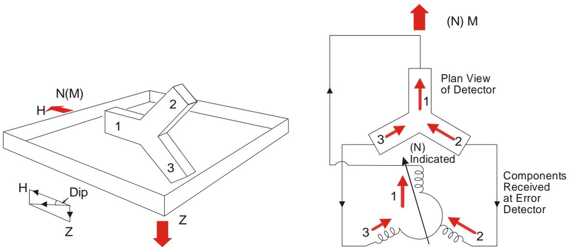
30. The error also depends on magnetic dip for, if the case at Fig 17 is repeated with a different dip, the components threading the spokes will alter. In Fig 18, the dip is increased, thereby increasing the error and reversing one component in this particular case.
