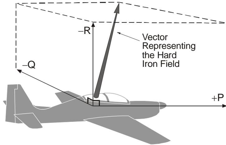
9. The fore-and-aft vector, P, will have the greatest deviating effect on H when the aircraft is on an East or West heading; on North or South the vector merely changes the magnitude of the directive force (Fig 4). The variation of the deviation due to P is in the form of a sine function as shown in Fig 5, i.e.:
