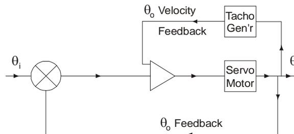
47. Varying degrees of damping can be achieved by adjustment of the feedback and much greater precision is possible than with viscous friction. Once again, optimum damping is sought.
