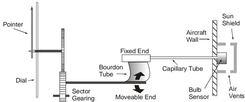
6. To minimize errors due to variations in the temperature of components other than the bulb, the volumes of the capillary tube and the Bourdon tube are kept small relative to the volume of the bulb. To compensate for changes of temperature at the indicator, a bi-metallic strip, which reacts in opposition to the motion of the Bourdon tube, is incorporated between the free end of the Bourdon tube and the pointer spindle.
