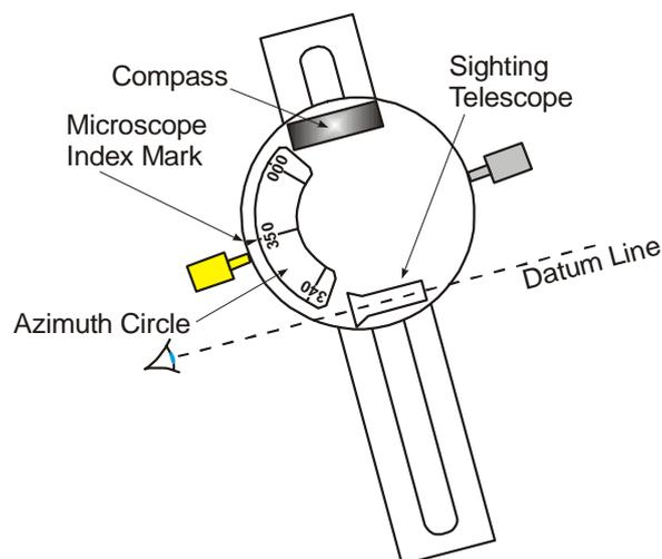
14. **Taking a Bearing.** Taking a bearing consists of three separate stages:
