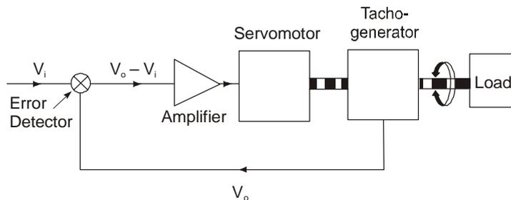
21. The input voltage ( $V_i$ ) is applied through a power amplifier to turn a servomotor, which accelerates the load towards the required speed. Comparison between the load speed and the input voltage is made possible by converting the speed into a voltage. The conversion is effected by a tachogenerator coupled to the output shaft. This is a special type of generator which gives a voltage proportional to its
