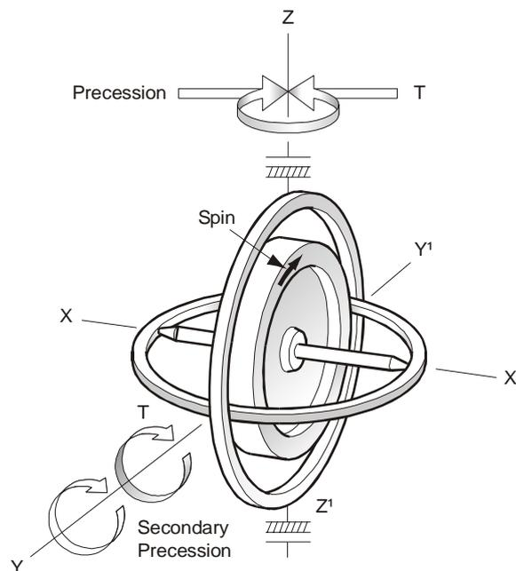
24. Secondary precession can only take place when the gyro is already precessing, thus its name. Note also that secondary precession acts in the same direction as the originally applied torque.
