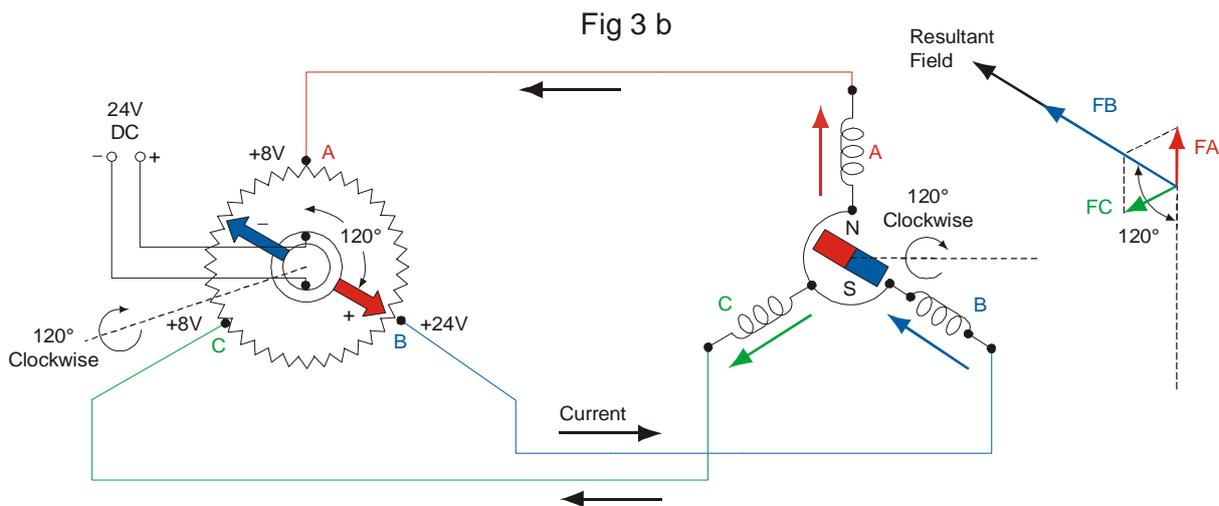
Thus, if the wipers in the transmitter are placed in any position by the input shaft, the resultant field at the receiver and hence the rotor magnet take up corresponding positions. If a pointer, moving over a calibrated scale, is attached to the rotor, remote indication of the position of the input shaft is immediately available.
