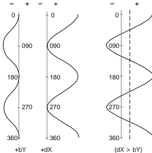
**5-15 Fig 15 Combination of Deviations due to Unequal Components of +bY and -dX**
