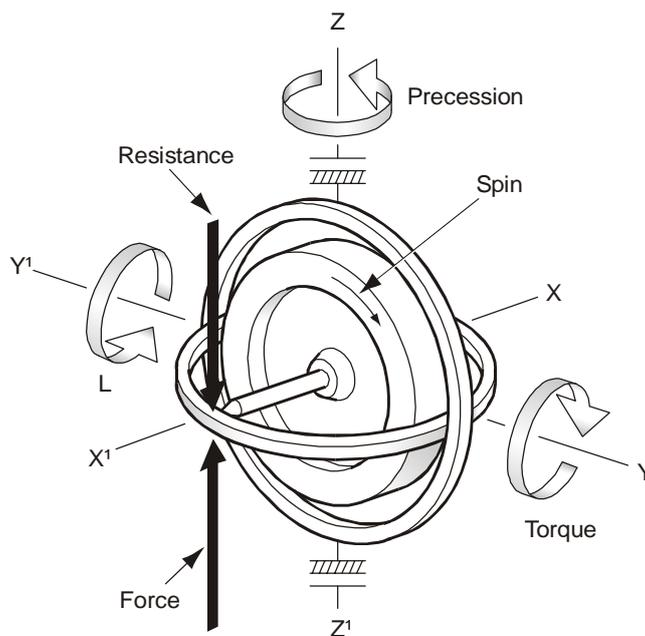
20. Gyroscopic Resistance is always accompanied by precession, and it is of interest to note that, if precession is prevented, gyroscopic torque cannot form, and it is as easy to move the spin axis when it is spinning as when it is at rest. This can be demonstrated by applying a torque to the inner gimbal
