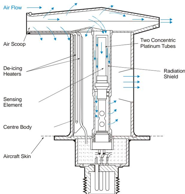
23. **De-icing.** The de-icing heater, embedded in the material of the probe, is a tube containing an axial wire element, which operates continuously throughout flight. The heating is not thermostatically controlled but is self-compensating in that, as temperature rises, the resistance rises and so reduces the power consumption. The de-icing element heats the exterior of the probe. A cylindrical radiation shield protects the sensor from the heating effects of the element.
