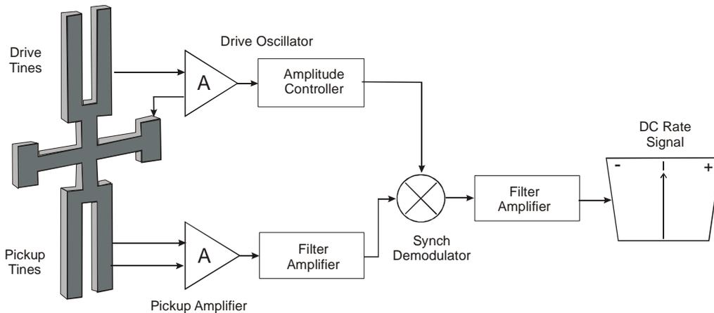
62. Vibration of the drive tines causes them to act like the arms of a spinning ice skater, where moving them in causes the skater's spin rate to increase and moving them out causes a decrease in rate. An applied rotation rate causes a sine wave of torque to be produced, resulting from 'Coriolis Acceleration', in turn causing the tines of the Pickup Fork to move up and down (not toward and away from one another) out of the plane of the fork assembly.
