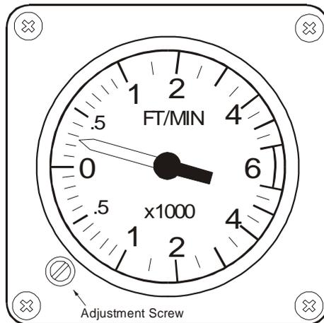
3. It is important that any given pressure difference between the inside and outside of the capsule should represent the same rate of climb or descent, regardless of the ambient atmospheric pressure and temperature variations with altitude. The function of the metering unit, in the manner in which it restricts the flow into the case, is to compensate for these changes in ambient conditions.
