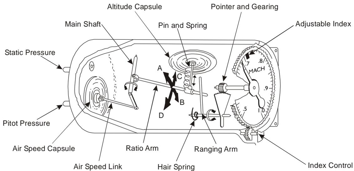
7. The altitude capsule responds to changes of static pressure, expanding or contracting with variation of altitude. The movement of the capsule is transferred to the ratio arm, via a spring and pin, causing it to move in the direction C-D. The pin is pointed at both ends and rests in cups on the altitude capsule and ratio arm (the spring providing the tension necessary to retain the pin in position).
