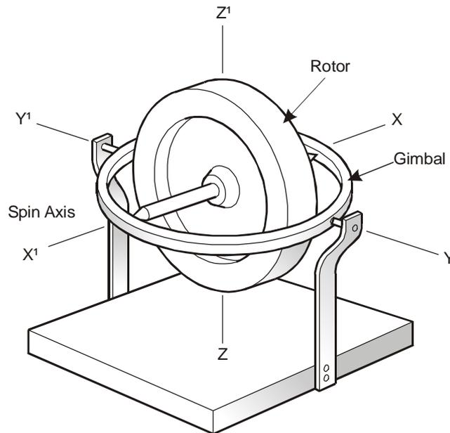
**5-11 Fig 2 Two-degrees-of-freedom Gyroscope**
