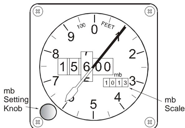
8. The servo drive can also be used to transmit altitude information to remote displays and to other systems, e.g. IFF/SSR. In current servo altimeters, the multiple needle display is replaced by a digital display, with an auxiliary pointer moving over a scale graduated in 50 ft increments from 0 to 1,000 ft (Fig 2).
