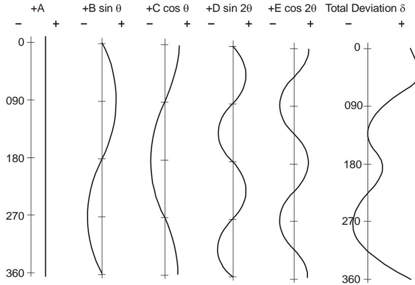
24. Although the previous discussion has considered the components of total deviation separately, they cannot in practice be measured individually as they act simultaneously. However, if the total deviation is measured on the eight headings at which the individual maxima occur, the values of all of the coefficients can be obtained by analysis of the total deviation equation.
