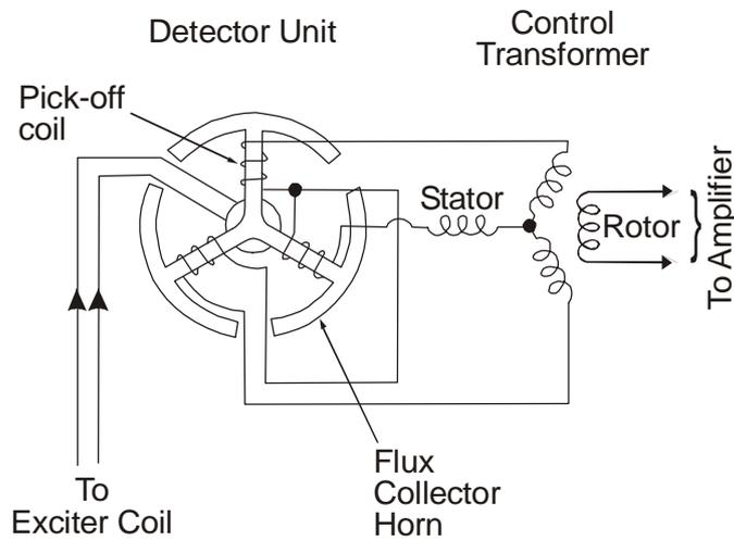
5-12 Fig 12 Operation of the Three-spoke Fluxvalve
