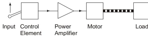
4. The control element, perhaps a variable resistor, applies the input to a power amplifier, which drives the motor in the required direction. The motor, in turn, moves the load.
