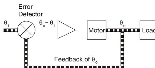
11. The automatic control system described operates by continuous cycling of the load position through the loop formed by the feedback, error detector, amplifier, and motor. Control mechanisms in which this loop can be identified are known as closed loop systems, while those which do not have feedback are known as open loop systems (e.g. Fig 1).
