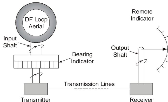
4. There are, however, many occasions when the accurate remote control of the position of a heavy load is required (eg remote rotation of a radar scanner). To provide the necessary torque servomechanisms (i.e. amplifiers and servomotors) are normally employed.
