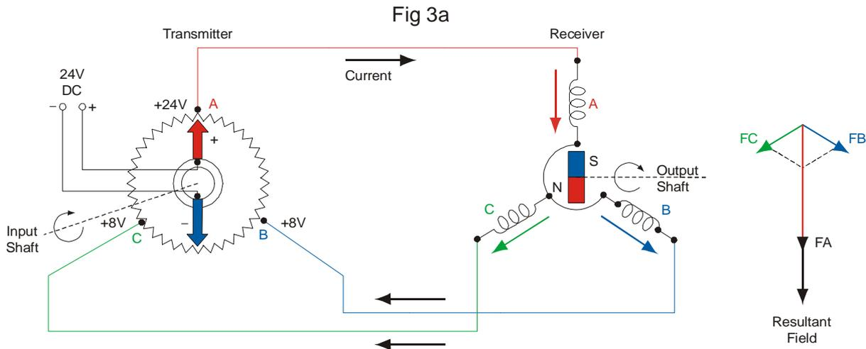
b. If the input shaft is rotated through  $120^\circ$  in a clockwise direction as shown in Fig 3b, the voltage distribution around the potentiometer is such that current flows from B through coil B in the receiver then divides equally to flow through coils A and C back to the transmitter. The vectors show that the resultant magnetic field also rotates through  $120^\circ$  clockwise and the rotor shaft aligns itself along this new axis.
