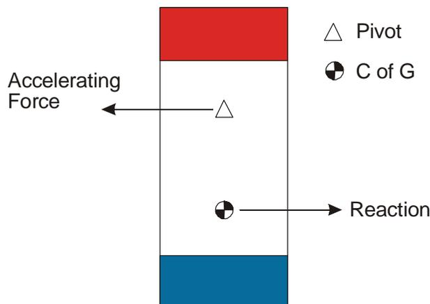
5-10 Fig 4 Acceleration Causing Tilt
