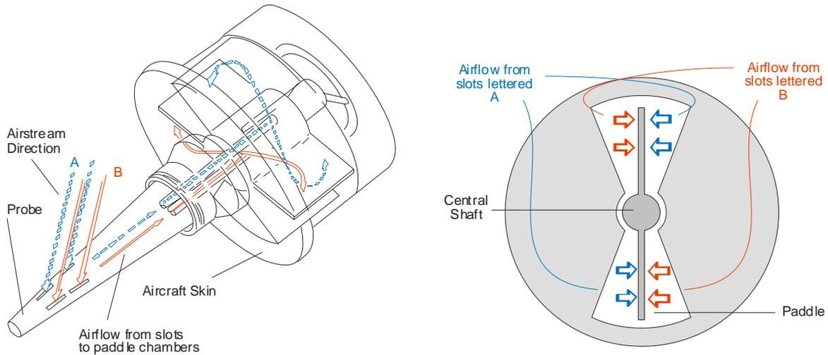
7. The position of the central shaft relative to the casing, and therefore to the aircraft, is transmitted to potentiometer assemblies by means of wiper arms, and the output voltage, which is related to AOA, may be used to operate the particular aircraft indicators or warning devices. In some installations two ADDs are provided to add a measure of redundancy, and so that the output voltage from the two can be compared, and the higher taken, to provide an additional margin of safety.
