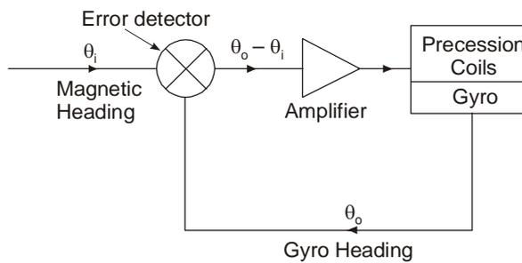
19. The GM compass is therefore essentially a servomechanism, and the fact that a second servo (see Fig 4) is used to provide the load position feedback is a matter of design convenience. Indeed some systems use a direct mechanical link for the feedback. Whatever the feedback method, the servo principle can be identified in all GM compasses.
