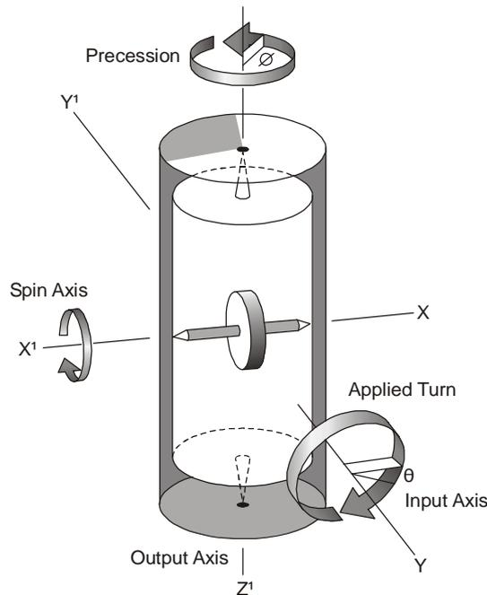
32. A gyro mounted so that it senses rotations about a horizontal input axis is known as a levelling gyro. Two levelling gyros are required to define a level plane. Most inertial platforms using conventional gyros align the input axis of their levelling gyros with True North and East.
