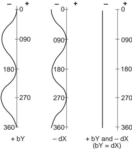
5-15 Fig 13 Combination of Deviation due to Equal Components of  $+bY$  and  $+dX$
