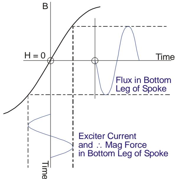
19. Since the top and bottom legs are identical, the amplitudes of the flux of the two legs are equal but 180° out of phase with each other relative to the pick-off coil, which is wound round both legs. Therefore, the resultant flux cutting the pick-off coil, which is the algebraic sum of the flux in the top and bottom legs is zero as shown in Fig 9.
