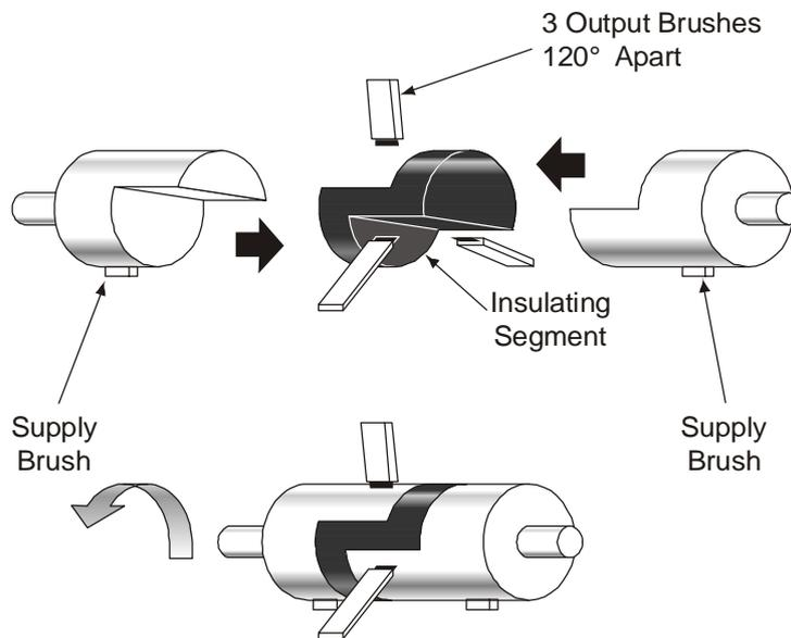
12. The receiver unit is similar to that in the Desynn system, although the rotor may be either a permanent magnet or a laminated soft-iron core. The outer end of each coil in the receiver is connected to one of the three pick-off brushes in the transmitter. More than one receiver may be operated from a single transmitter.
