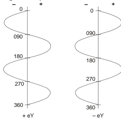
19. **Coefficients E and A.** Coefficients E and A are due to components  $bY$  and  $dX$ . Each component produces a deviation which varies with heading in the form shown in Fig 11; this function is the cosine of twice the heading, displaced to one side or the other of the zero axis.
