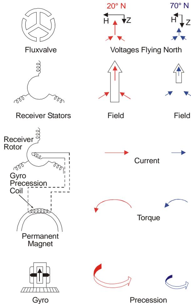
**GYRO-MAGNETIC COMPASS SYSTEM ERRORS**
