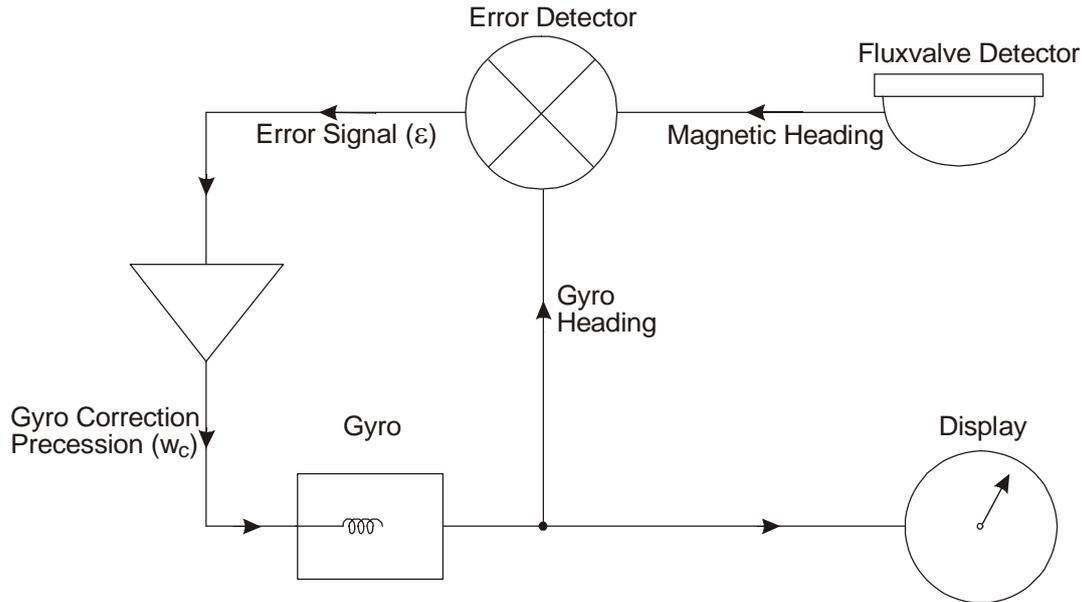
36. The method of mechanizing the gyro precession loop is of extreme importance. Three methods of accomplishing the task are as follows:
