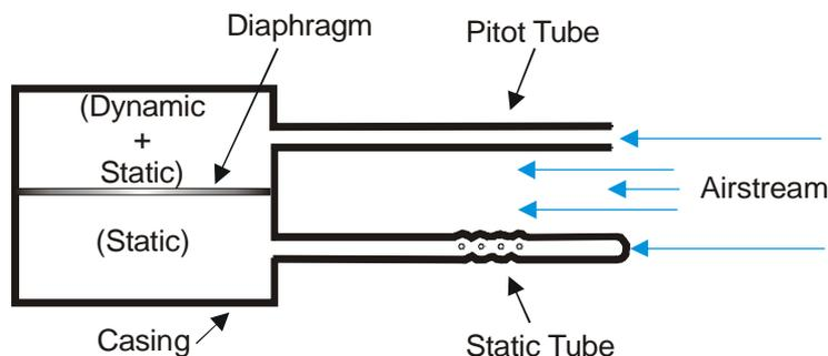
4. When moved through the air, the pitot tube will pick up pitot pressure made up of static pressure and dynamic pressure. The pitot pressure is led through a pipeline to one side of a sealed chamber, divided by a thin flexible diaphragm. The static tube is unaffected by dynamic pressure as its end is closed, however, the small holes will pick up local static pressure. The static pressure is led through a second pipeline to the other side of the diaphragm.
