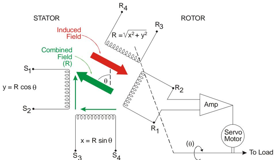
32. **Resolver Synchro (Differential).** It is often necessary to produce the sine and cosine of the sum of two angles multiplied by a given value, eg northings and eastings relative to true North represented by R (ground speed), multiplied by cosine and sine  $\theta$  (true track) may be required as
