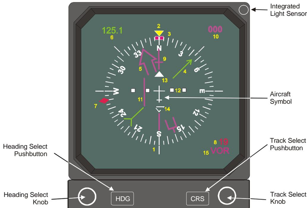
1. **Compass Card.** The compass card indicates gyrocompass heading in conjunction with the lubber line (2). The card rotates clockwise as the aircraft turns left. If the compass fails, the card freezes and a red HDG FAIL caption is superimposed.
