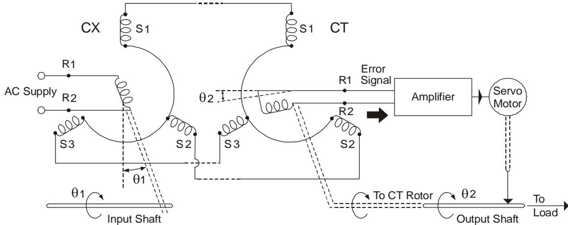
24. **Control Synchro Accuracy.** Using a suitably powered motor, the control synchro accuracy is independent of load. Typical accuracy figures are 16 minutes of arc.
