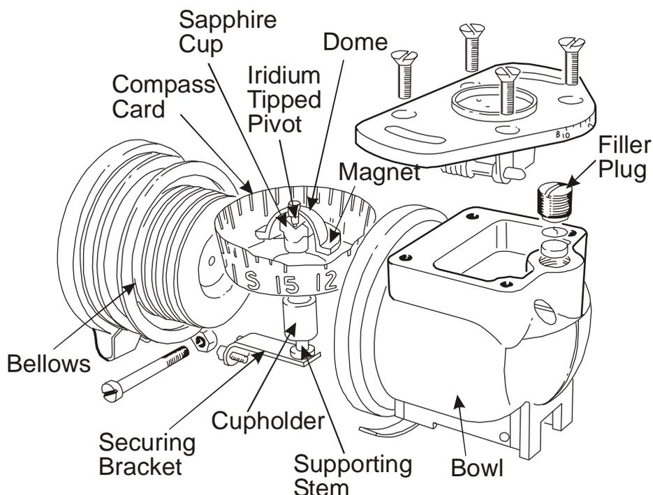
19. **Serviceability Checks.** Before use the compass should be checked to ensure that the bowl is not cracked or damaged and is completely filled with fluid that is free from excessive discolouration, bubbles and sediment.
