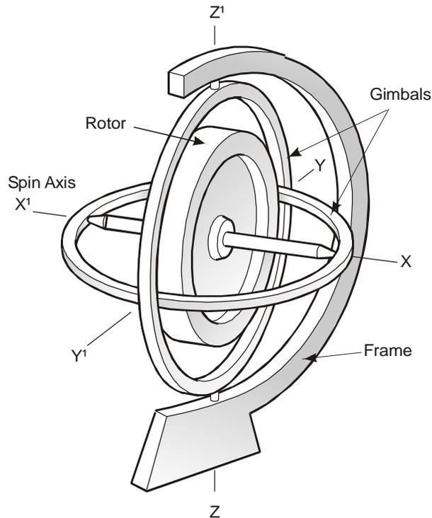
3. The physical laws which govern the behaviour of a conventional gyroscope are identical to those which account for the behaviour of the Earth itself. The two principal properties of a gyro are rigidity in inertial space and precession. These properties, which are explained later, are exploited in some heading reference and inertial navigation systems (INS) and other aircraft instruments.
