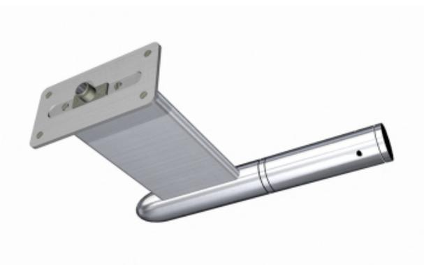
18. The housing is designed such that air entering the probe head proceeds into a venturi. Inside, most of the air that comes into contact with the venturi walls is expelled through ports in the housing. However, a small central flow of air is passed over the tube containing the element at a very reduced speed, and then discharged through holes in the outlet ring.
