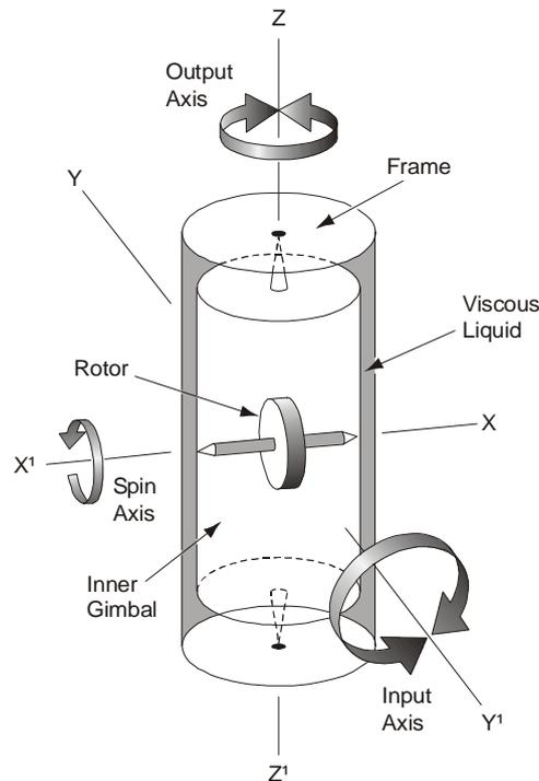
29. The rate-integrating gyro was designed for use on inertial navigation stable platforms, where the requirement was for immediate and accurate detection of movement about three mutually perpendicular axes. Three rate-integrating gyros are used, each performing its functions about one of the required axes. These functions could be carried out by displacement gyros, but the rate-integrating gyro has certain advantages over the displacement type. These are:
