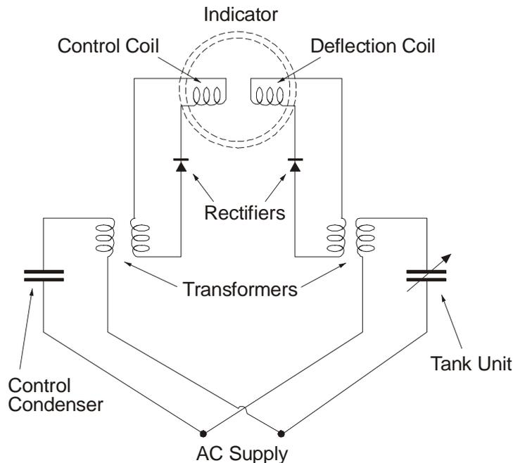
4. Normally, at least two units are fitted in each tank, connected in parallel. This ensures that accuracy is maintained despite aircraft attitude changes (within specified limits) as the fall in fuel level at one end of the tank is compensated for by the rise at the other end (Fig 2).
