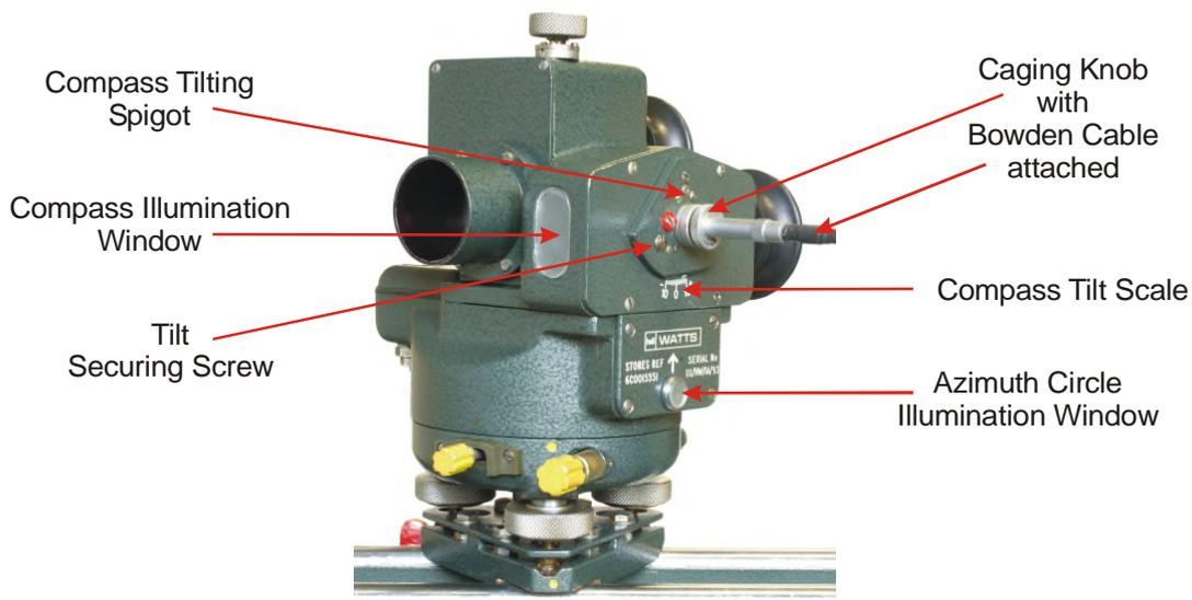
8. **The Compass Box.** The compass box (Fig 4) is closed at its North end by a ground glass window and at its South end by a convex lens. A mirror above the magnet pivot faces the lens and can, for collimation purposes, be moved about its vertical axis by a small adjustment screw. The compass box is mounted on a horizontal spigot so that it may be tilted to allow for dip. It can be tilted up to  $10^\circ$  either side of the horizontal and locked in position by two screws (see Fig 3).
