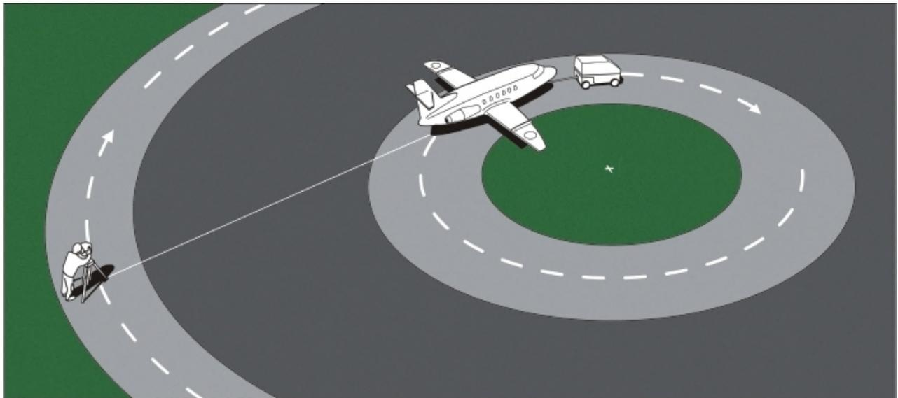
2. A full compass swing usually consists of a 'correcting swing' followed by a 'calibration swing'.
