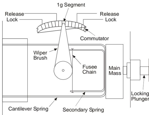
5-27 Fig 6 Basic Fatigue Meter Mechanism
