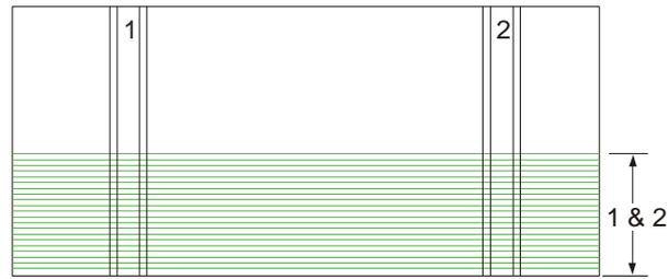
Tank Level (Capacitance of 1 and 2 Equal)
