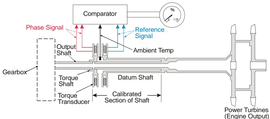
**5-26 Fig 7 Torquemeter Transmitter**
