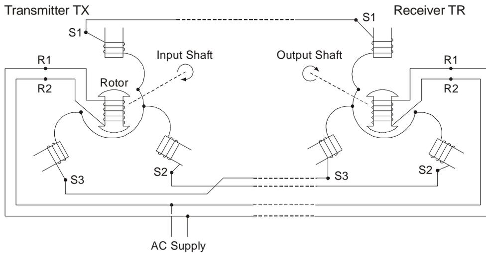
**5-24 Fig 8 Construction of Torque Synchro**
