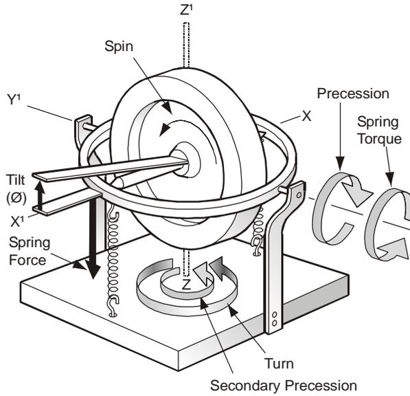
27. The relationship between the deflection angle and rate of turn is derived as follows:
