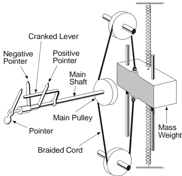
6. A cranked lever is attached to the shaft, and the horizontal arm of this lever is interposed between positive and negative pointers so that they will be moved when the shaft rotates, and will remain in their new positions on the return of the shaft to the neutral position. The recording pointers may be reset to the neutral position when desired. A device is fitted to damp out vibrations and prevent violent pointer fluctuations under short period accelerations.
