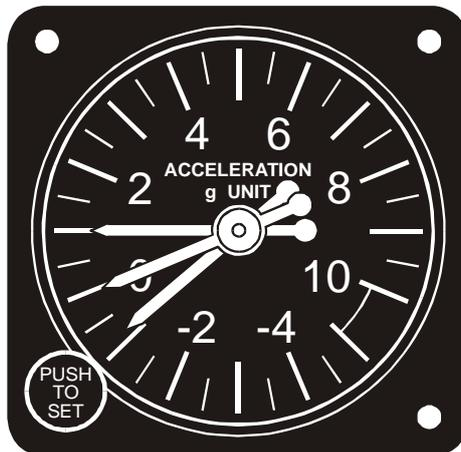
8. The cockpit accelerometer should not be confused with the aircraft fatigue meter. This instrument will normally be installed outside the cockpit (often in the undercarriage bay) to monitor cumulative acceleration forces on the airframe. Details of the fatigue meter may be found in Volume 5, Chapter 27, Para 15 and in Volume 1, Chapter 19, Para 12.
