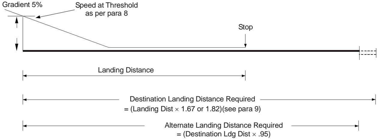
**10. Reference Landing Distance.** This is the gross horizontal distance required to land on a reference wet hard surface from a height of 30 ft and come to a complete stop. The speed at a height of 30 ft is the maximum threshold speed ( $VAT_0 + 15$  kt); touch down is at the Reference Touch Down Speed, after a steady gradient of descent to the 30 ft point of not greater than 5% ( $3^\circ$  glide path) under limiting operational conditions of ceiling and visibility.
