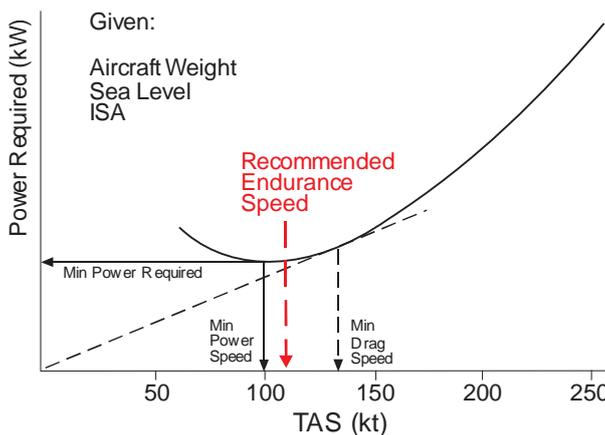
30. It should be recognized that the recommended IAS for endurance is considerably higher than the minimum possible flight IAS. There is a large rate of drag increase at the lower speeds as shown in Fig 4. To overcome this drag, flight at very low airspeeds entails the use of power much higher than that required for maximum endurance. Indeed, level flight is possible on some aircraft at speeds well below the power-off stalling speed.
