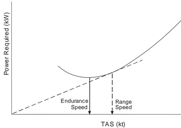
37. It should be remembered that the recommended speeds for an aircraft are unlikely to match the ideal because they take account of individual aircraft characteristics, manoeuvrability requirements, altitude considerations and the like. That said, in general, the endurance speed is about 80% of the range speed.
