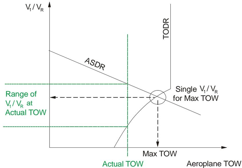
21. When field lengths are unbalanced it is necessary to consider individually take-off run, accelerate stop distance and take-off distance available. If, however, ASDA and TODA are of the same length, or assumed to be so, then the field is said to be 'balanced' and compliance with these 2 distance requirements can be achieved simultaneously for the case of power unit failure at  $V_1$ . From a balanced field chart it is possible, in one step, to determine:
