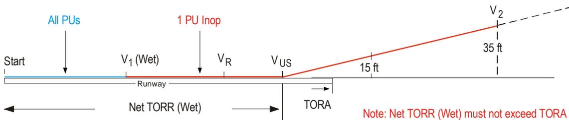
10. **TORR Compliance.** In order to comply with Air Navigation (General) Regulation 7(2) therefore, TORR should be the greatest of sub-para 9a, b or c and must not exceed TORA.
