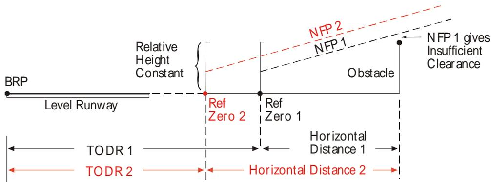
13. **Runways with a Slope.** When a slope exists in the take-off distance, either up or down, not only will the horizontal distance vary, but also the relative heights of the obstacles and reference zero will need careful consideration (see Figs 5 and 6)
