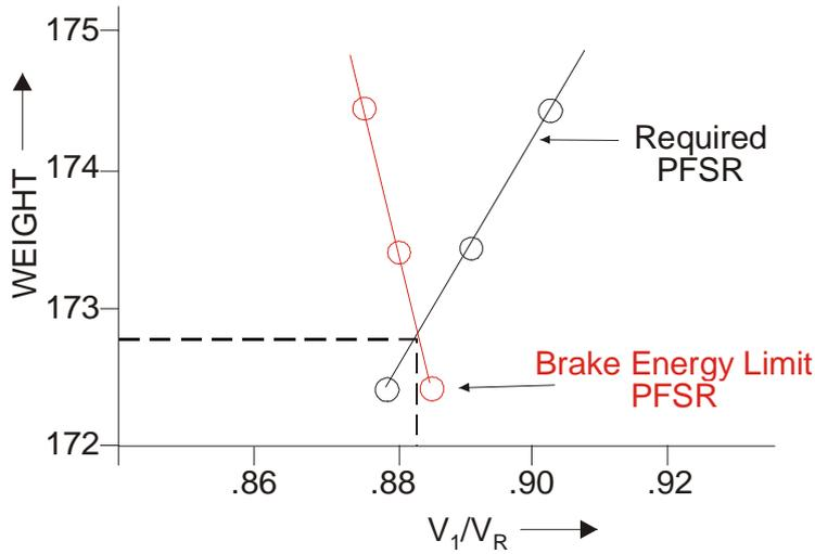
7. The intersection of the two lines (in Fig 3) gives the take-off weight and the corresponding PFSR. From this the take-off distance (all engines) operating requirement must again be checked.
