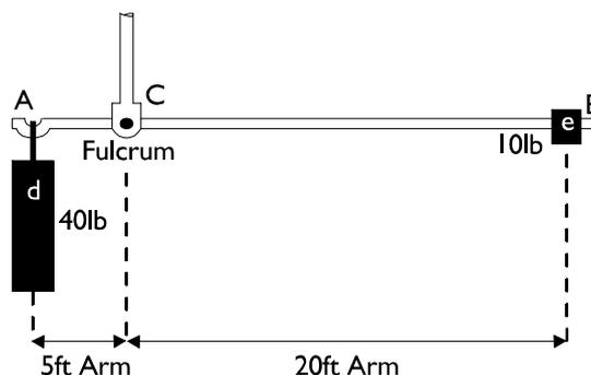
16. **Practical Application of the Principle.** In practice, the formula  $\text{weight} \times \text{arm} = \text{moment}$  is used to determine the position of the CG of any aircraft by using the weights and arms of the various loads
