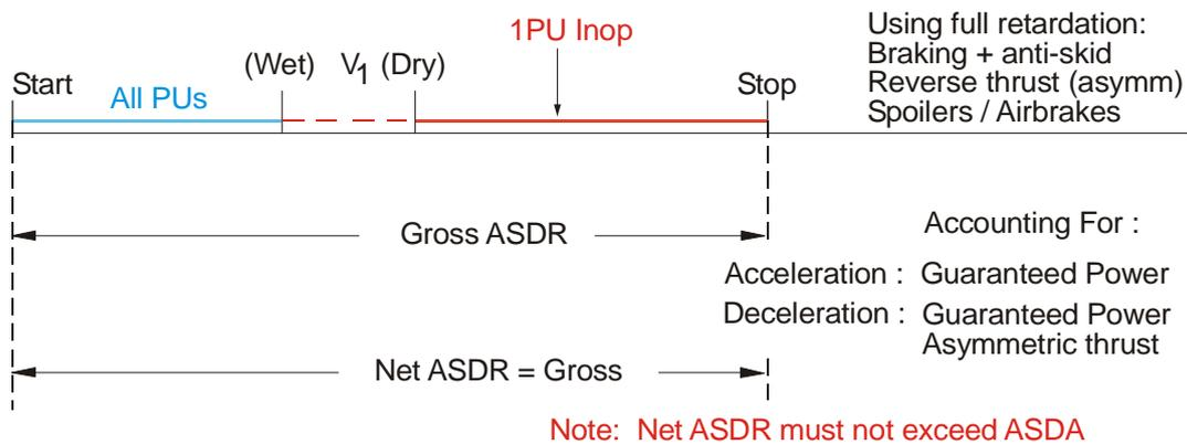
b. The sum of the gross distance to accelerate with all power units operating from the starting point to the decision point ( $V_1$ ) appropriate to a wet runway and the gross distance to stop with the critical power unit inoperative from the decision point on the reference wet hard surface using all available means of retardation (see Fig 5).
