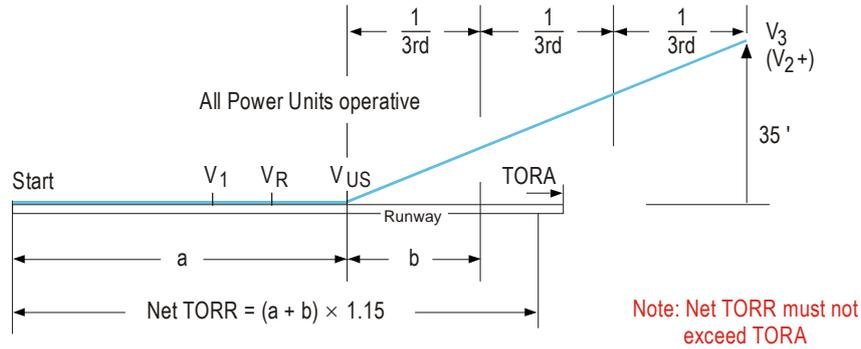
b. **One Power Unit Inoperative.** This is the gross distance from the starting point to the point where the aeroplane becomes airborne ( $V_{US}$ ) plus  $1/3$  the gross distance between  $V_{US}$  and the point at which it attains a screen height of 35 ft. The power unit fail point shall be such that failure would be recognized at the decision point ( $V_1$ ) appropriate to a dry runway (see Fig 2).
