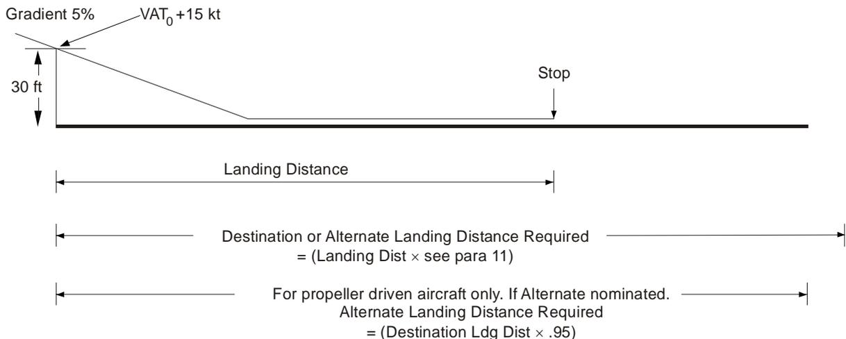
12. **Limiting Landing Weight.** Paras 8 to 11 covered the landing distance requirements for the destination and alternate aerodrome. Each must be considered separately and the most limiting will govern the maximum permissible landing weight (C of A and WAT limits apart). When comparing the destination and alternate to obtain the limiting landing weight, allowance must be made for fuel burn-off between destination and alternate.
