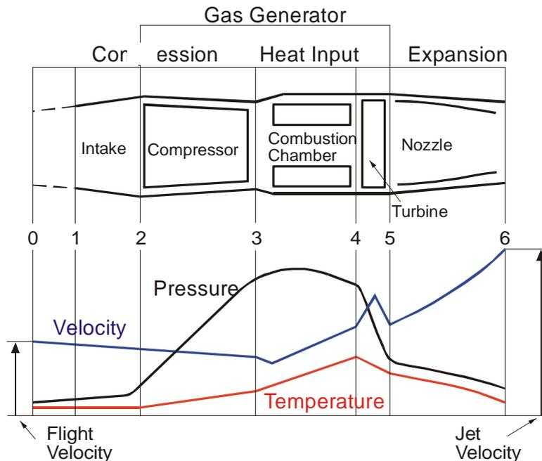
2. The thrust produced by a turbojet engine can be expressed thus:
