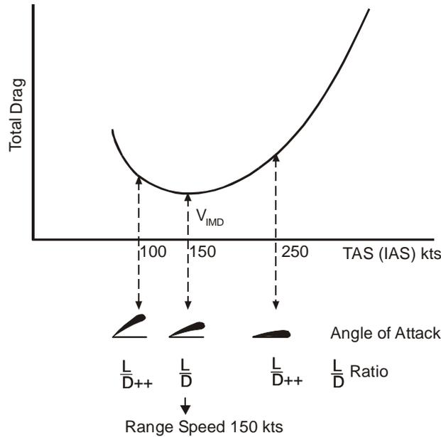
7.  **$\frac{\text{Lift}}{\text{Drag}}$  Ratio.** Assuming that the AUW remains constant, the lift in level flight follows suit.
