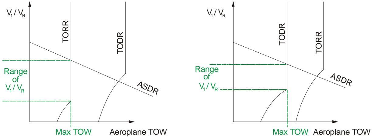
There will also be a range when the actual take-off weight is less than the maximum permissible (see Fig 13). The decision to use high or low  $V_1$  depends upon the aeroplane type and operating techniques.
