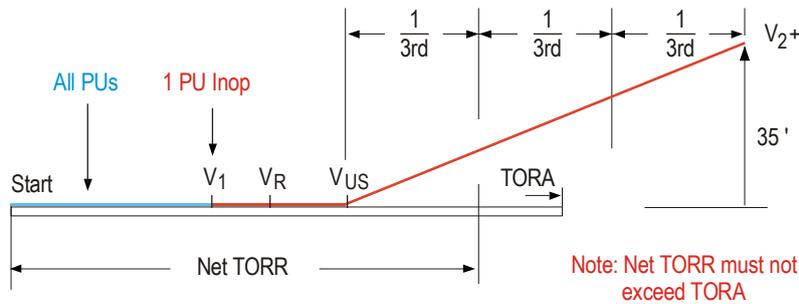
c. **One Power Unit Inoperative - Wet Runway.** This is the gross distance from the starting point to the point where the aeroplane becomes airborne ( $V_{US}$ ) to effect a transition to climbing flight to attain a screen height of 15 ft at the end of TODA, in a manner consistent with the achievement of a speed not less than  $V_2$  at 35 ft. The power unit failure point shall be such that failure would be recognized at the decision point ( $V_1$ ) appropriate to a wet runway (see Fig 3).
