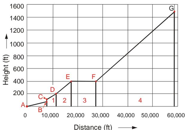
4. Plot the TODR (A-B) using the runway slope to calculate the height gained/lost by the end of TODR in relation to the 'brakes-off' point.
