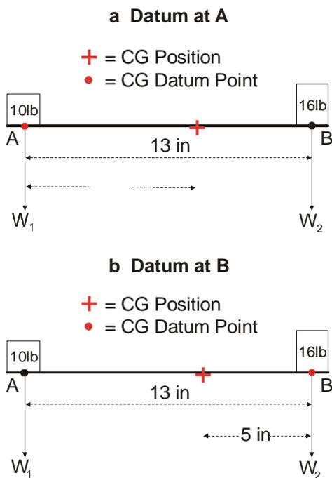
18. The distance of this point from a stated reference point, ie a CG datum point, can be calculated by dividing the algebraic sum of the moments of the weight about the reference point by the sum of the weights. For example, Fig 2a assumes that the CG datum point is at A and, following the accepted conventions regarding positive and negative load arms and moments, the algebraic sum of the moments of the weights is:
