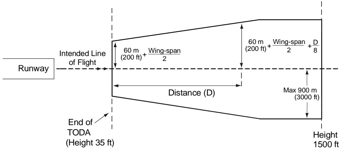
7. The domain within which an object can be considered a legal obstacle can therefore be plotted for a straight take-off as in Fig 1. If the aeroplane changes its direction of flight by more than 15°, the obstacle domain maintains the same dimensions but curves with the curved intended line of flight.
