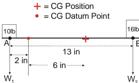
22. Summarizing, in the examples in paras 17 – 20, the data given consisted of the two weights and their corresponding load arms. From this, the algebraic sum of the longitudinal moments is calculated. The sum of the moments (remembering that sign is important) is then divided by the sum of the weights to give the longitudinal distance and the fore-and-aft direction of the new CG position from the CG datum point.
