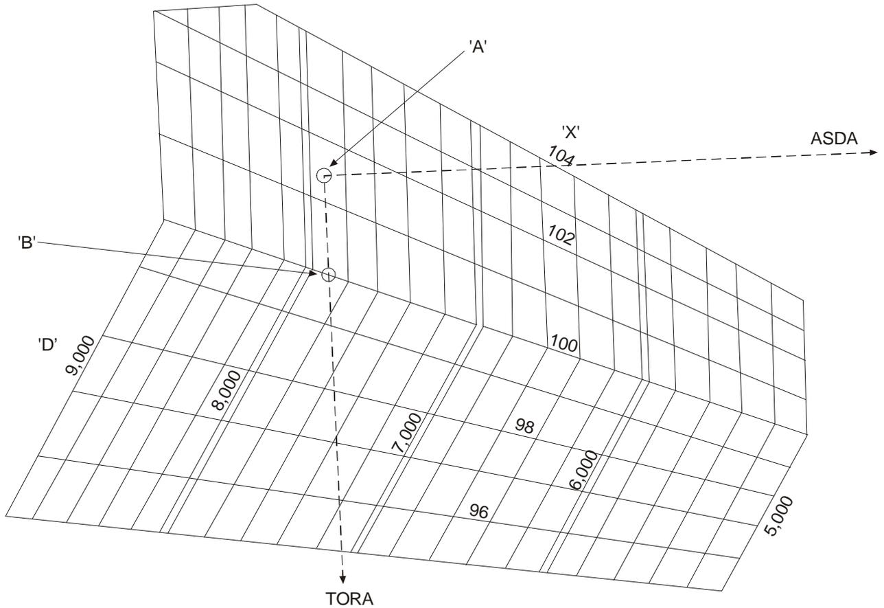
b. **Take-off Weight Less Than Maximum Take-off Weight.** There will always be a range of  $V_1$  when the take-off weight is less than the maximum take-off weight. The usable range will be governed by take-off run or take-off distance whichever is limiting in determining maximum take-off weight (see Fig 6).
