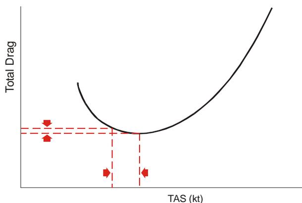
28. Although the theory is sound, flight at the speed for minimum power is less than practicable since all ability to manoeuvre disappears and engine handling problems arise. For these reasons a margin of speed is added to improve manoeuvrability, resulting in a slightly higher recommended endurance speed which should be maintained within plus or minus five knots. Endurance speed may be defined as:
