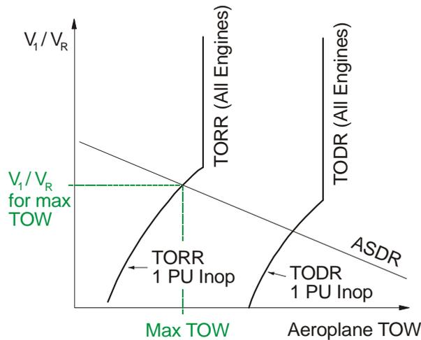
19. The disposition of the 3 graphs depends entirely on the airfield dimensions and, although in Fig 11 maximum permissible take-off weight and  $V_1/V_R$  ratio were determined by the take-off run 'one power unit inoperative' case, they might equally well have been determined by either of the take-off distance limitations.
