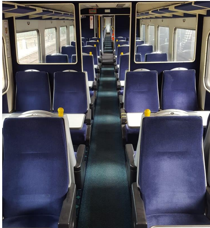
Mark 2 saloon showing narrow clearway
