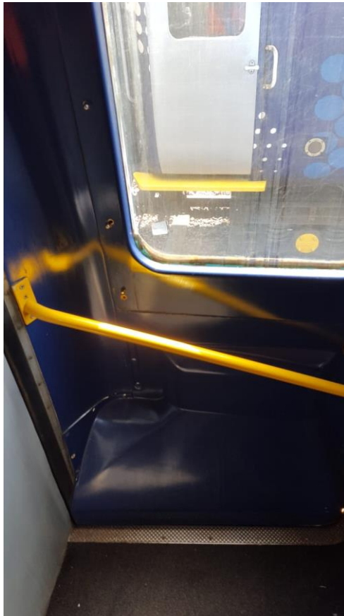
Mark 2 coach slam door with integral grab rail
