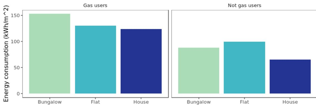
Figure 4: Mean electricity consumption in 2017, by gas use status and property type
