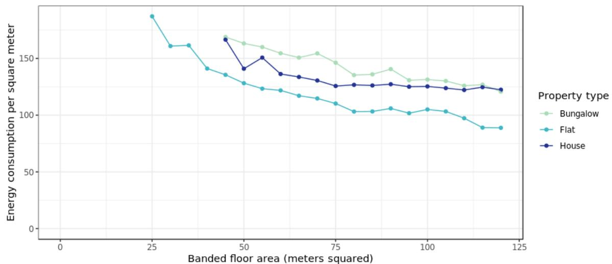
Figure 6: Relationship between banded floor area and mean energy consumption per m<sup>2</sup> (houses only)
