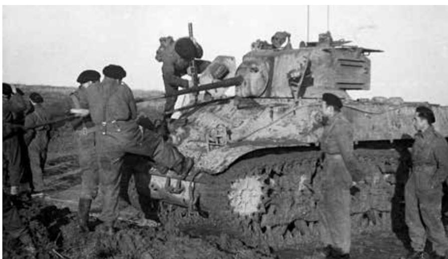
A long barrel rod is used by Polish tank crewmen to clean the gun barrel, preventing the build-up of dirt
