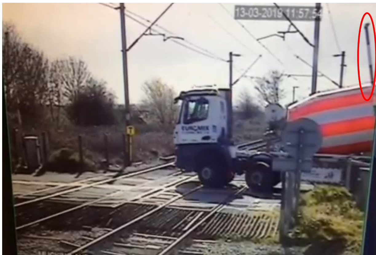
Figure 9: Level crossing camera view showing lorry stopped and about to start reversing manoeuvre. The crossing barrier (highlighted) has started to lower (courtesy of Network Rail)
