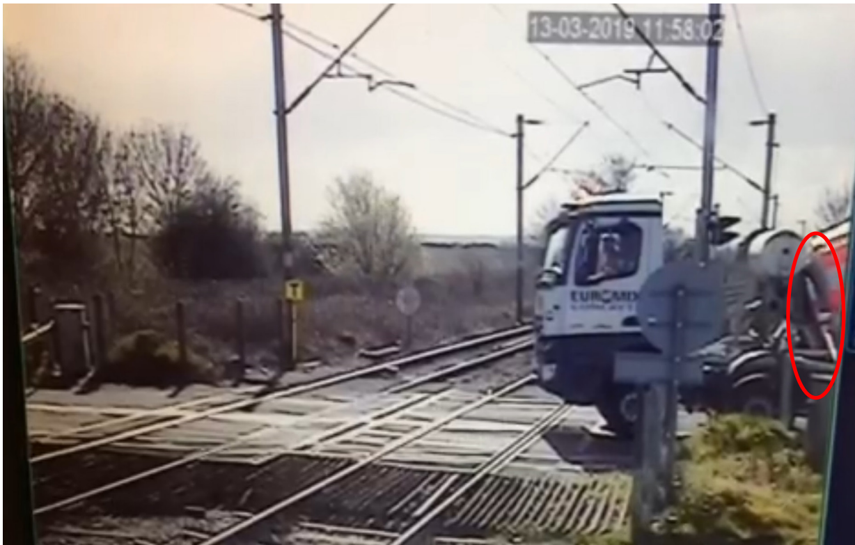
Figure 10: Level crossing camera view of the stationary lorry and partly lowered level crossing barrier (highlighted) caught by equipment on the back of the lorry. The approaching train is hidden by the lorry (courtesy of Network Rail)
