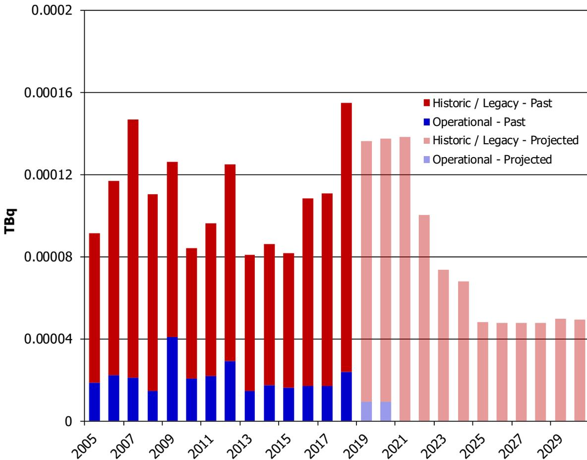
Figure 5. Past and projected total beta discharges associated with particulates from gaseous effluents
