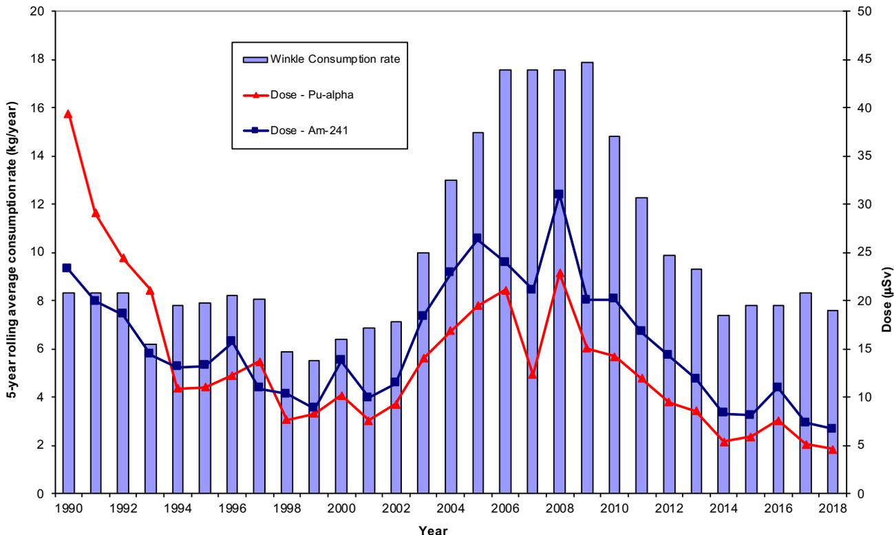
Figure 2. Dose to marine critical group from Pu-alpha and Am-241 in mussels and consumption rate
