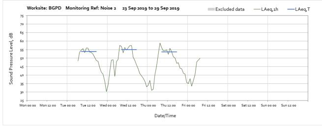
Note: Missing data between 17:00 on Sunday 22<sup>nd</sup> and 05:00 on Tuesday 24<sup>th</sup> of September was due to a technical fault with the monitoring station. Following completion of the works the monitor was removed at 08:00 on Friday 27<sup>th</sup>.
