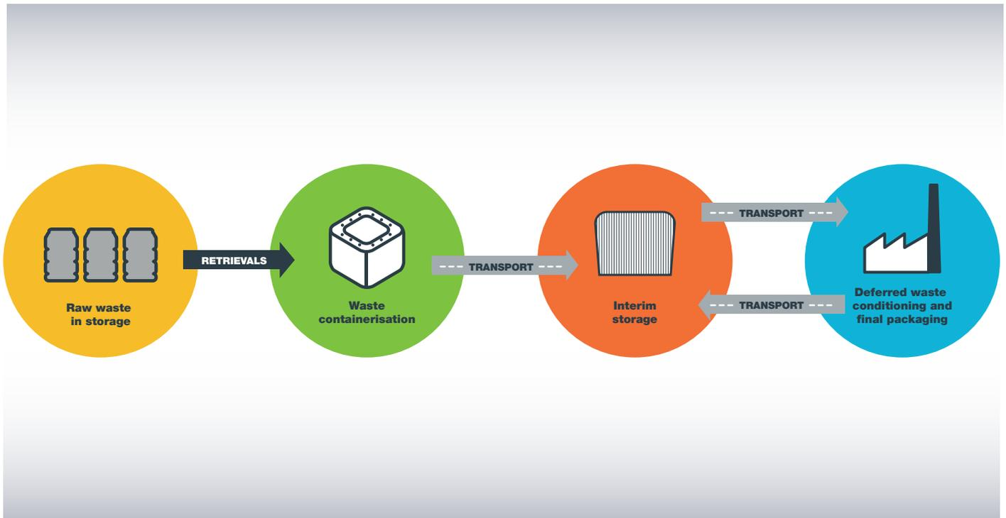
**FIGURE 6 - EXAMPLE OF A CONTAINERISATION WITH DEFERRED FINAL WASTE CONDITIONING**
