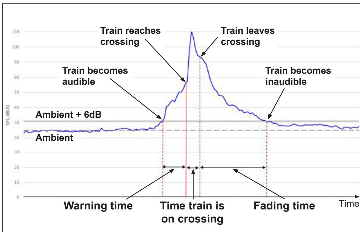
Figure 10: Typical sound trace recorded at Tibberton No. 8 footpath crossing
