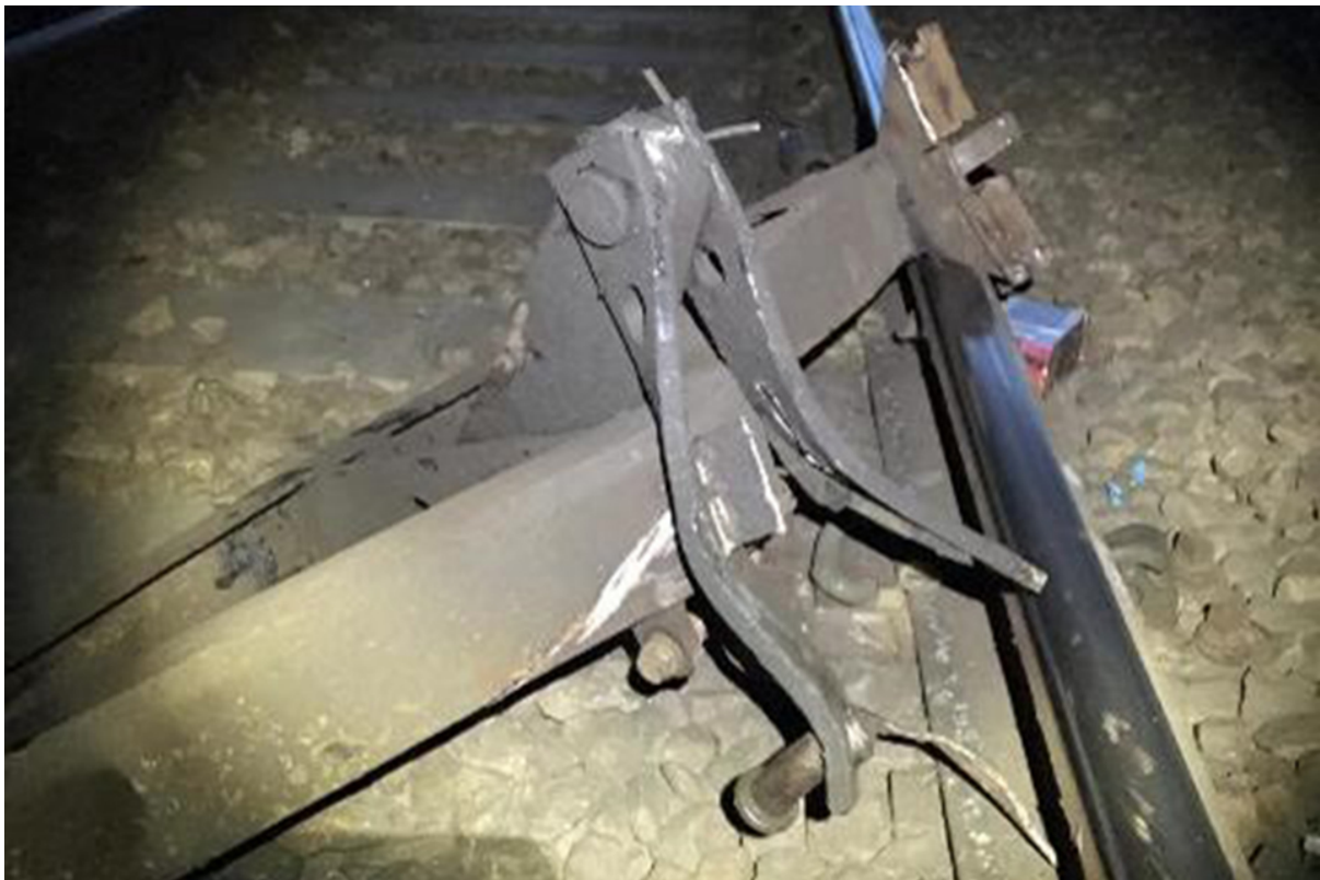
Figure 2: Detached brake gear found after the accident (courtesy Network Rail)
