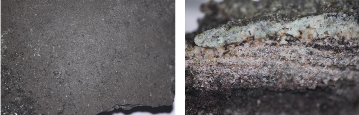
Figure 33 Example of deposit form combustion chamber floor
