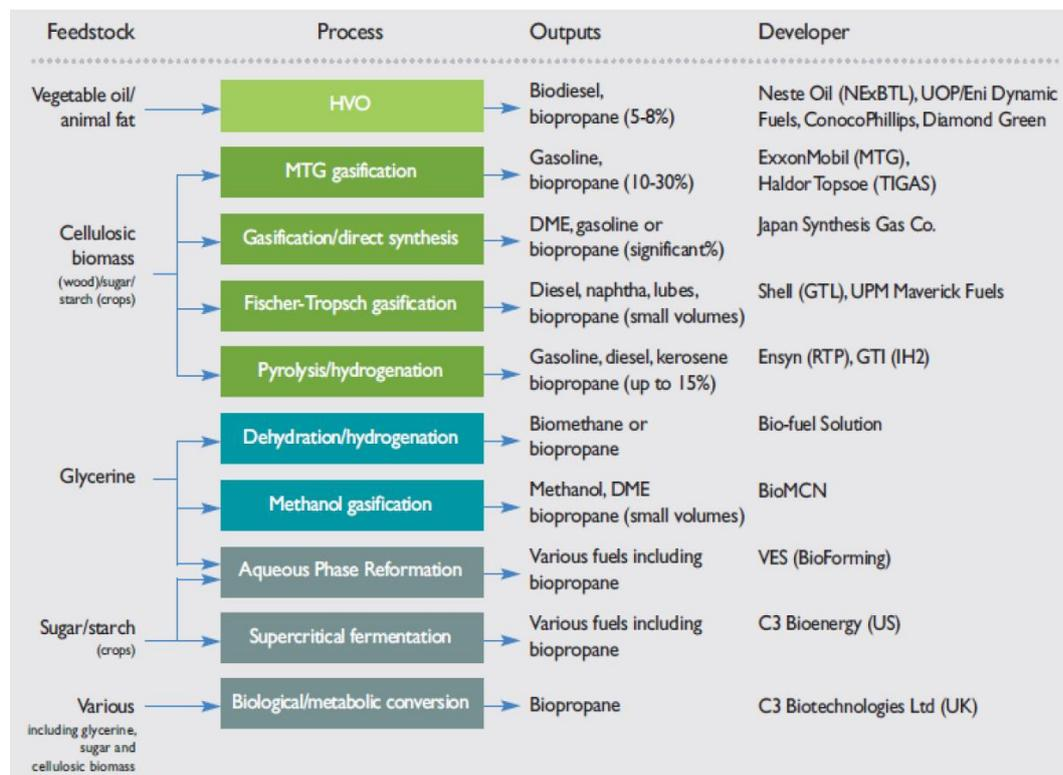
Figure 18: Main technologies being used or developed to produce BioLPG. Source: UKLPG.
