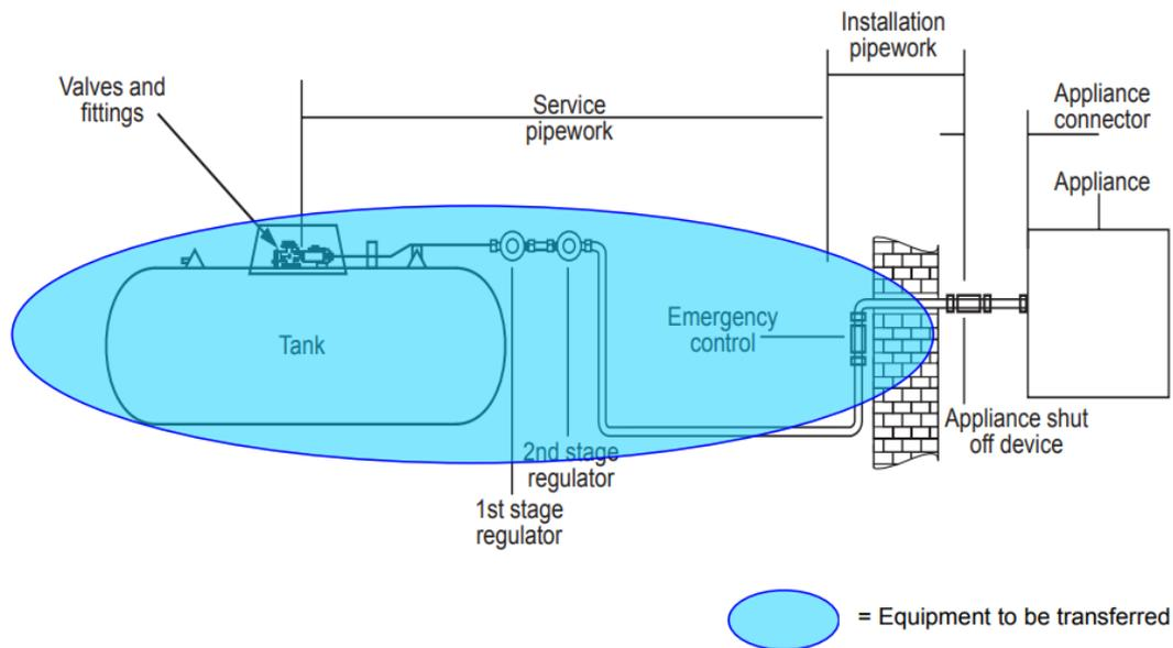
Figure 7. Typical domestic LPG installation showing equipment owned by the supplier [13]
