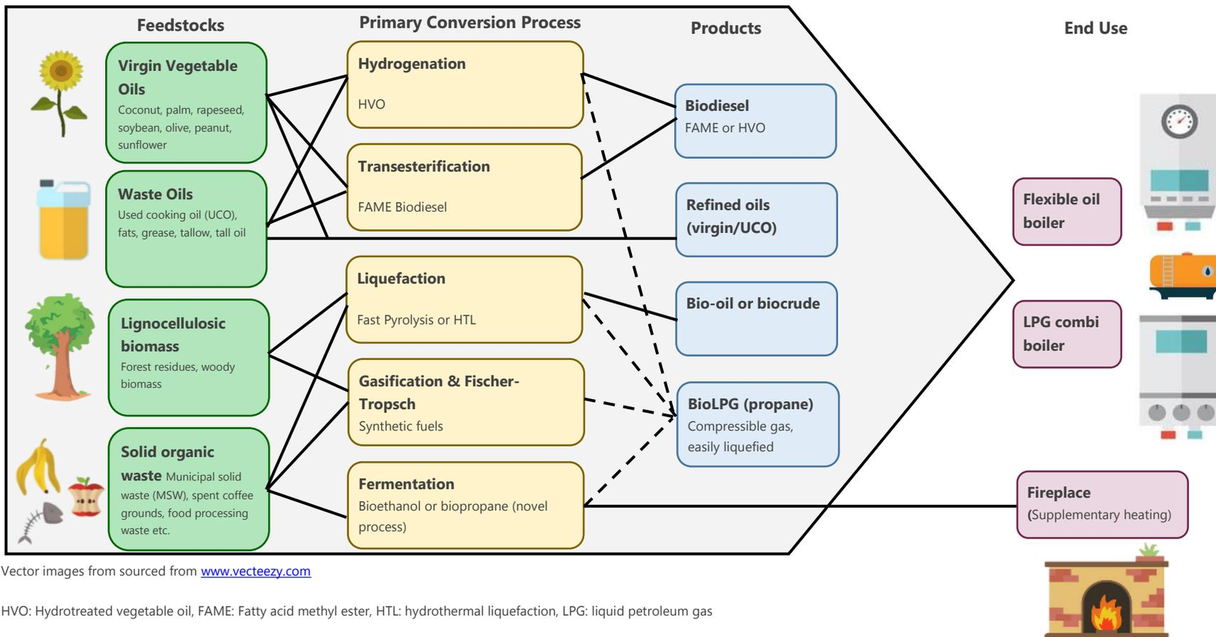
Figure 2. Flow chart for the production of bioliquids for domestic heating
