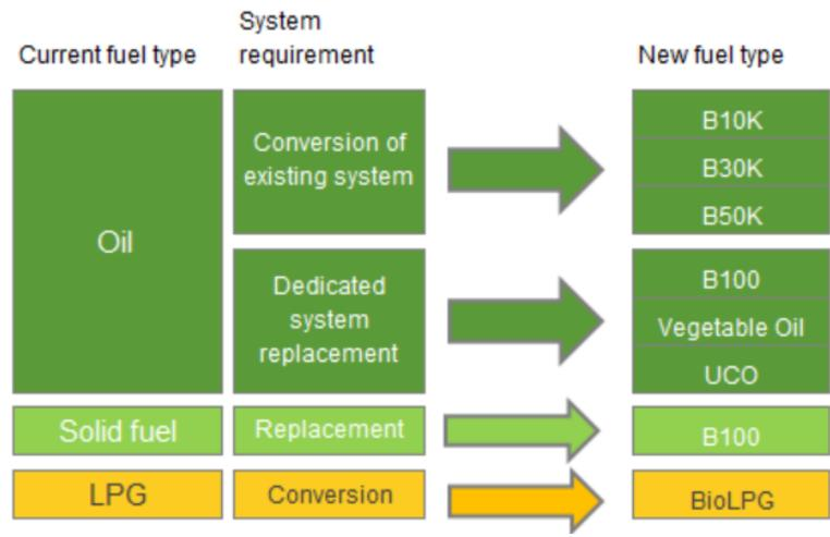
Figure 4: Illustration of technologies and fuel types covered in the deployment model.
