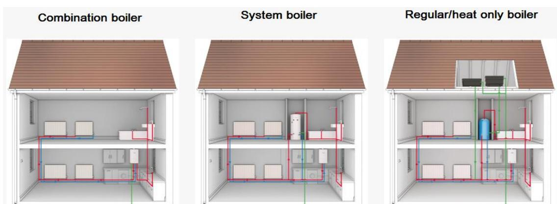
Figure 5. Key boiler types. Image source: Worcester-Bosch<sup>2</sup>
