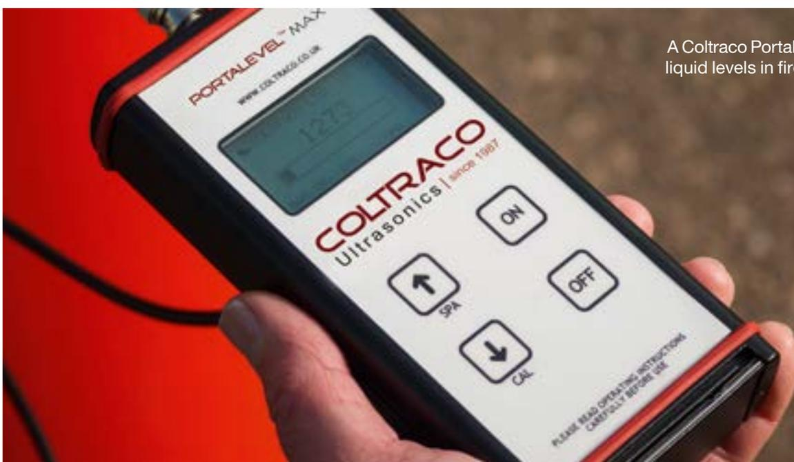
A Coltraco Portalevel MAX for inspecting liquid levels in fire suppression systems
