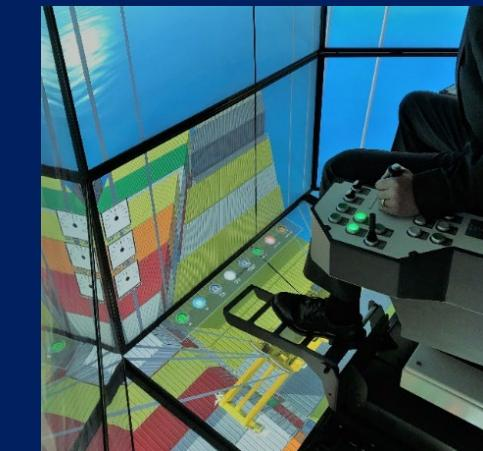
A state of the art training and technology suite at the Port of Tilbury includes two training simulators provide a full, 360-degree experience, of major crane and straddle operational equipment. This provides operators with an enhanced learning environment featuring industrial controls and realistic working terminal scenarios.
