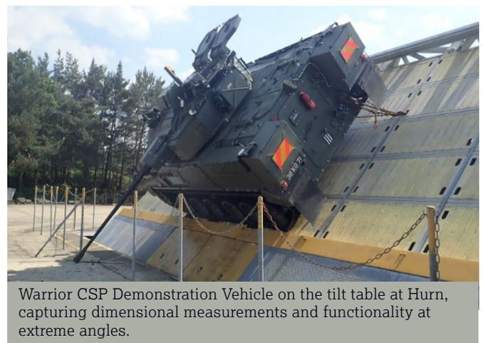
Warrior CSP Demonstration Vehicle on the tilt table at Hurn, capturing dimensional measurements and functionality at extreme angles.
