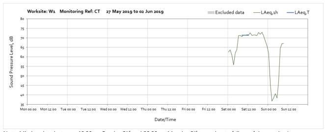
Note: Missing data between 10:00 on Sunday  $2^{nd}$  and 09:00 on Monday  $3^{rd}$  were due to failure of the monitor's battery. No works were undertaken during this period.
