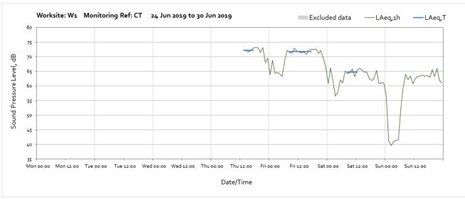
Note: Missing data between 12:00 on Friday 21st and 12:00 on Thursday 27th were due to failure of the monitor's battery. HS2 works were undertaken between 08:00 and 16:00 on Friday 21st.
