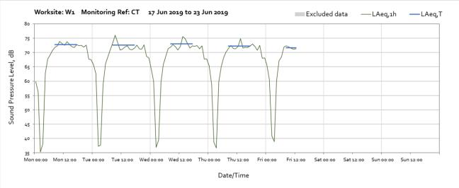
Note: Missing data between 13:00 on Friday 21st and 12:00 on Thursday 27th were due to failure of the monitor's battery. HS2 works were undertaken between 08:00 and 16:00 on Friday 21st.
