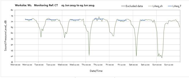
Note: Missing data between 10:00 on Sunday 2<sup>nd</sup> and 09:00 on Monday 3<sup>rd</sup> were due to failure of the monitor's battery. No HS2 works were undertaken during this period.
