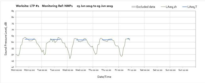
Note: The monitor was relocated from this position to a new monitoring location (NMP2) between 11:00 and 12:00 on the 6<sup>th</sup> of June.
