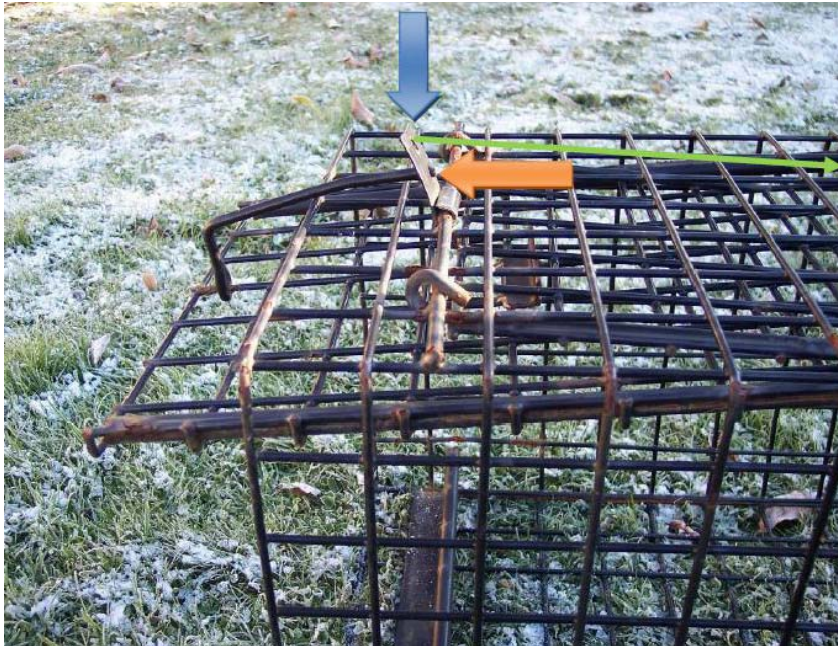
Plate 1: Trigger mechanism of trap showing hinge plate in roughly vertical position (blue arrow) and tip of trigger arm passed through lower hole of hinge plate (orange arrow) to hold trap door open. The green arrow indicates the line of twine, once set, from the upper hole of the hinge plate, running towards rear of trap.
