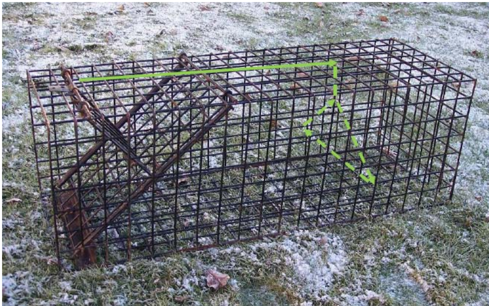
Plate 2: Setting the trap: the green line marks the line of twine from the hinge plate (which will be ~vertical when set) towards the rear of the trap, then through the roof into the trap 20-25cm from the rear, then out first through one side then the other, then back to join the central line of twine. This join should be made with a slip-knot that can be pushed down into the trap to form a triangular 'coat-hanger' shape, as shown. The other end of the string is then tied to the hinge plate with the door held open (as in Plate 1).
