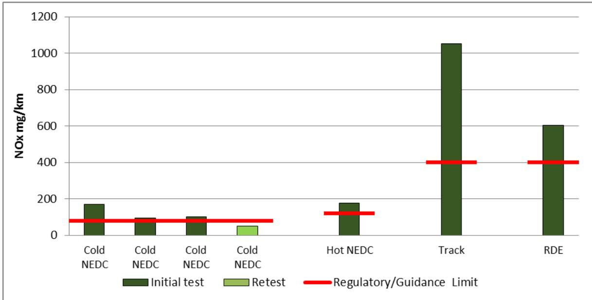
Figure 4-21: NO<sub>x</sub> emissions for the Vauxhall Astra SRI CDTi (1). Limit shown is the legislative limit for the NEDC (cold) test and the recommended guidance limits for the other tests
