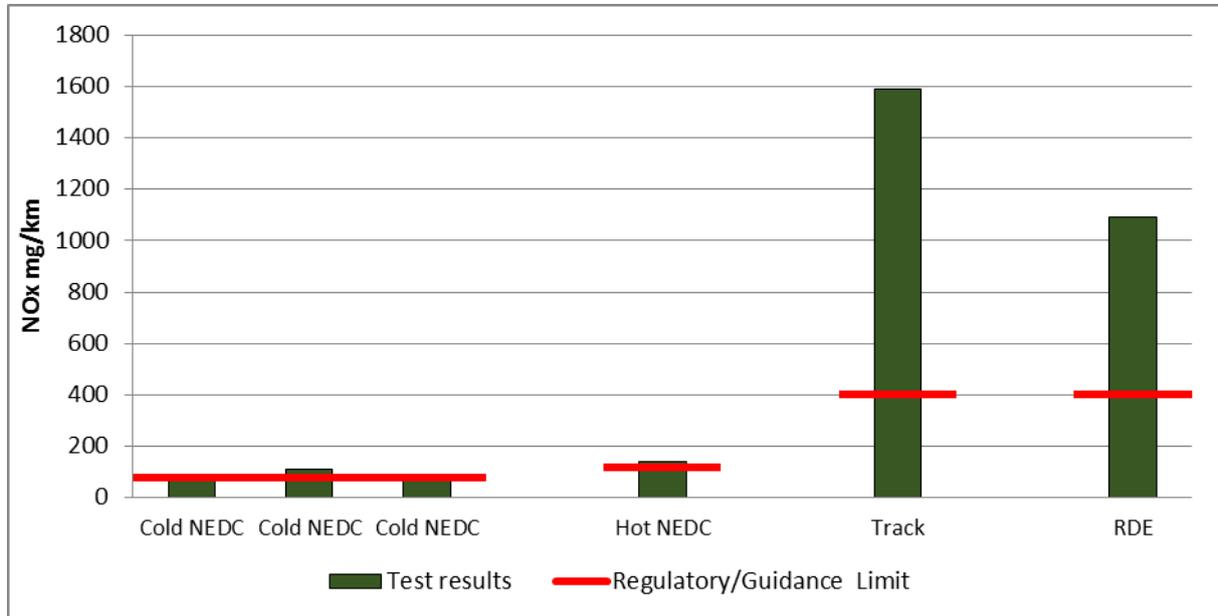
Figure 4-14: NO<sub>x</sub> emissions for the Renault Kadjar Dynamique DCI. Limit shown is the legislative limit for the NEDC (cold) test and the recommended guidance limits for the other tests
