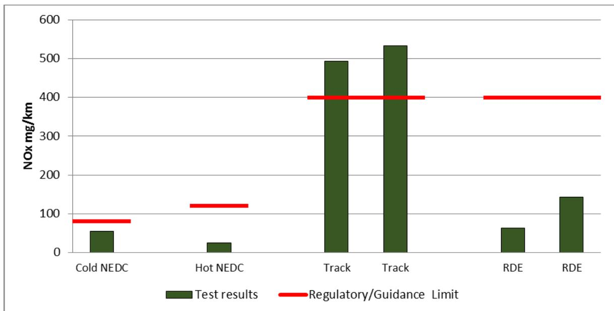
Figure 4-23: NO<sub>x</sub> emissions for the Jaguar F-Pace. Limit shown is the legislative limit for the NEDC (cold) test and the recommended guidance limits for the other tests
