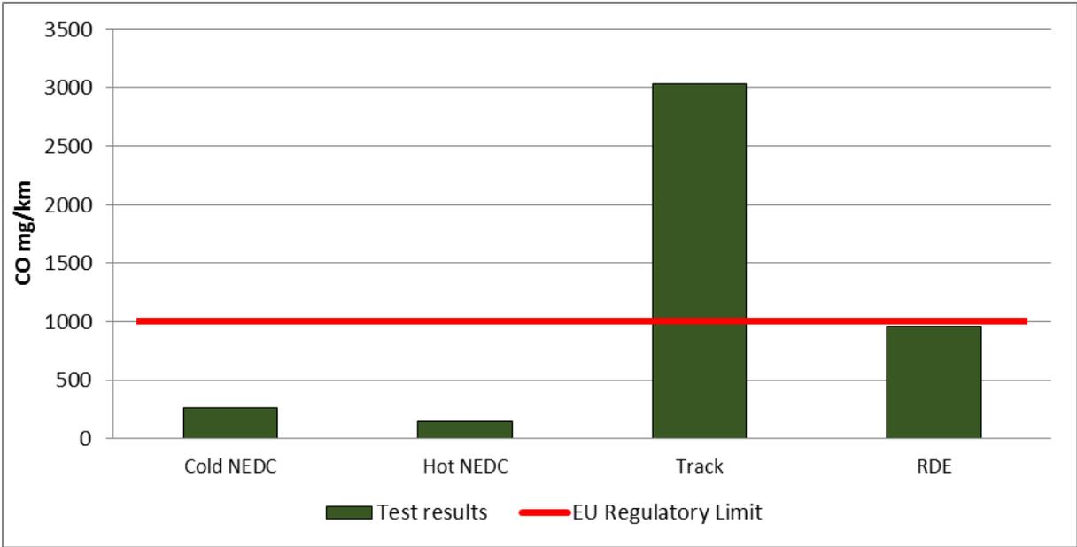
Figure 4-6: CO emissions for the Nissan Juke Tekna CVT. Limit shown is the regulatory limit for the NEDC (cold) test
