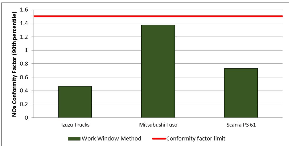
Figure 4-28: Results of the in-service, on-road emissions tests conducted on 3 HGVs. NO<sub>x</sub> results have been calculated in line with the relevant conformity factors described in section 3.13
