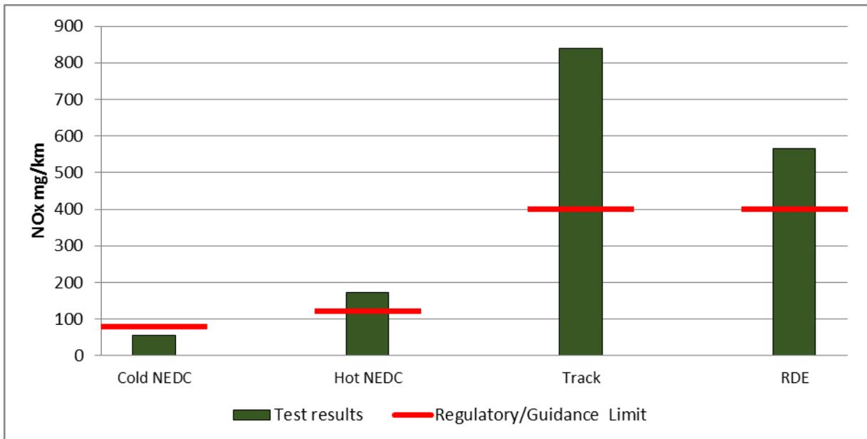
Figure 4.22: NO<sub>x</sub> emissions for the Vauxhall Astra SRI CDTi (2). Limit shown is the legislative limit for the NEDC (cold) test and the recommended guidance limits for the other tests
