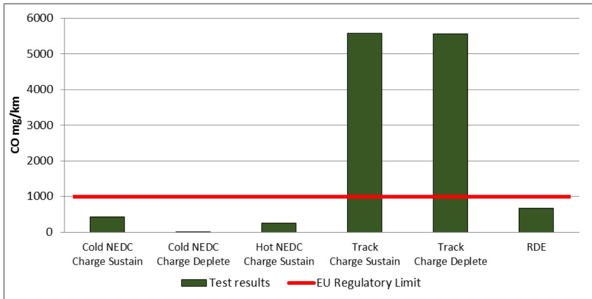
Figure 4-9 Laboratory NEDC (cold & hot), WLTP (track) and RDE CO emissions for PHEV car compared to the EU regulatory limits
