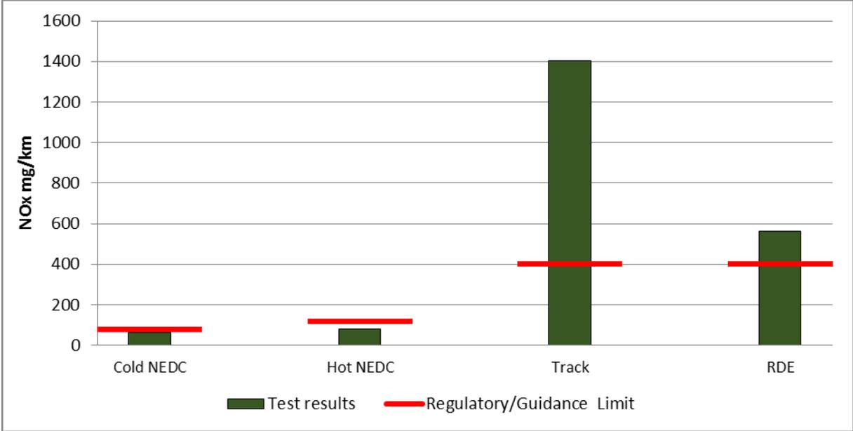
Figure 4-15: NO<sub>x</sub> emissions for the Nissan Qashqai N-Connecta DCI (vehicle 1). Limit shown is the legislative limit for the NEDC (cold) test and the recommended guidance limits for the other tests
