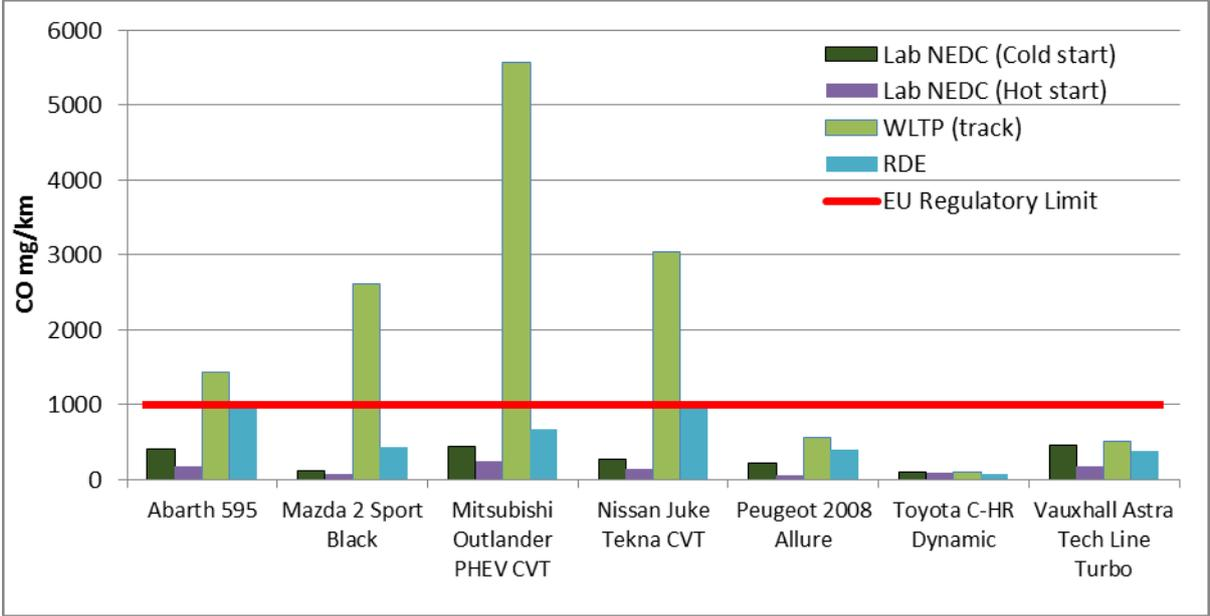
Figure 4-5: WLTP (track) results for petrol cars and PHEV compared to the EU recommended guidance limits
