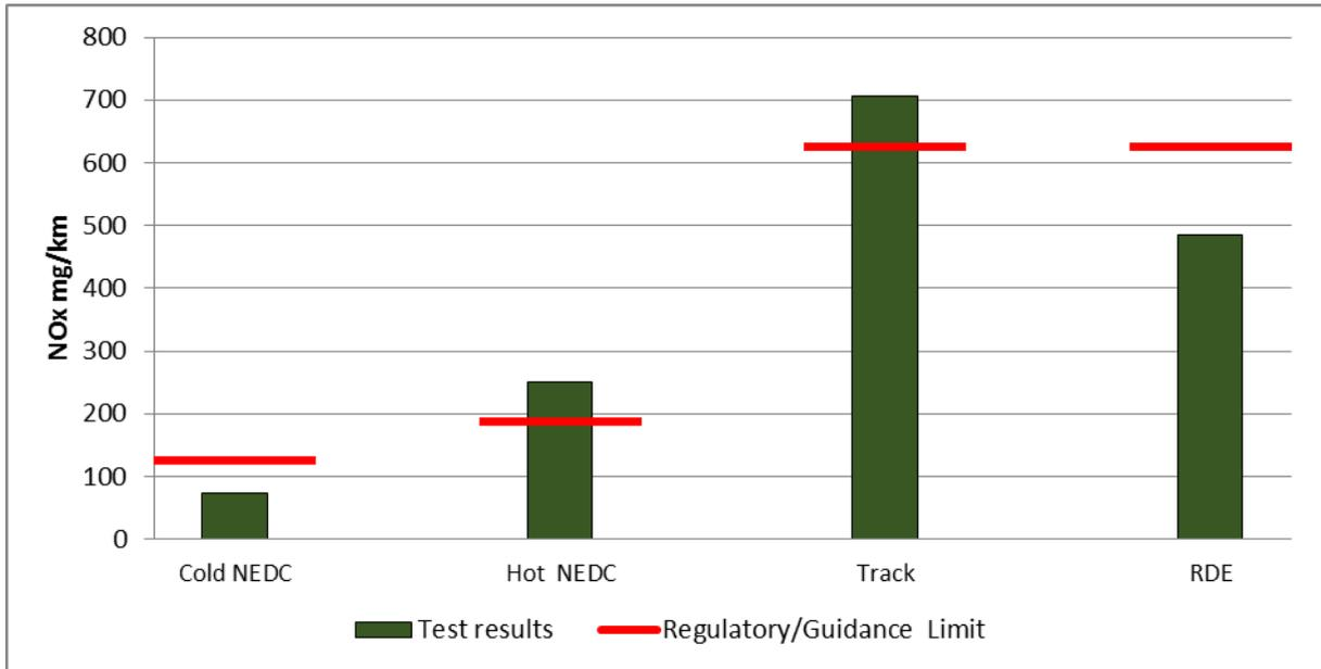
Figure 4.27 NO<sub>x</sub> emissions for the Mercedes Vito 114 Bluetec. Limit shown is the legislative limit for the NEDC (cold) test and the recommended guidance limits for the other tests
