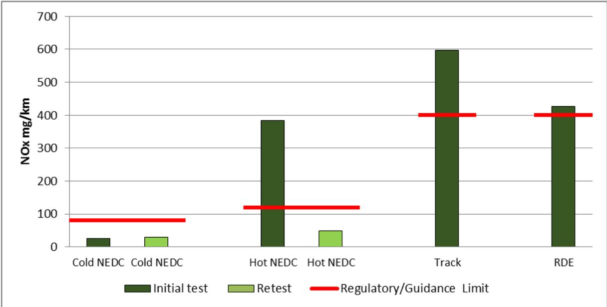
Figure 4-20: NO<sub>x</sub> emissions for the Hyundai Tucson SE B-Drive 2WD. Limit shown is the legislative limit for the NEDC (cold) test and the recommended guidance limits for the other tests
