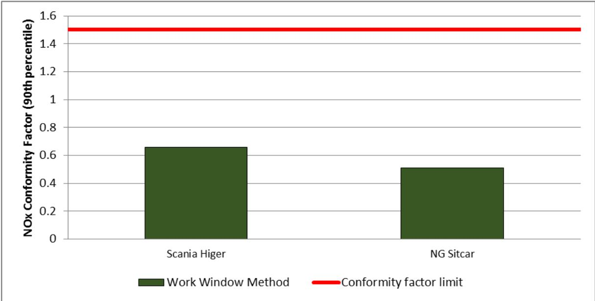
Figure 4-29: Results of the in-service, on-road emissions tests conducted on 2 PSVs. NO<sub>x</sub> results have been calculated in line with the relevant conformity factors described in section 3.16
