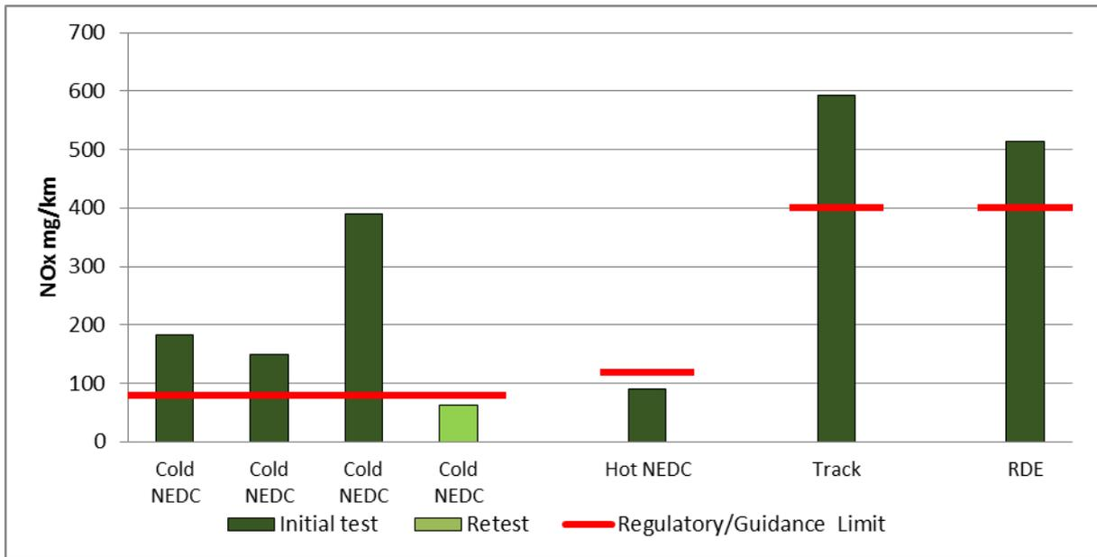
Figure 4.24: NO<sub>x</sub> emissions for the Volvo XC60 R-Design Lux D4 (1). Limit shown is the legislative limit for the NEDC (cold) test and the recommended guidance limits for the other tests
