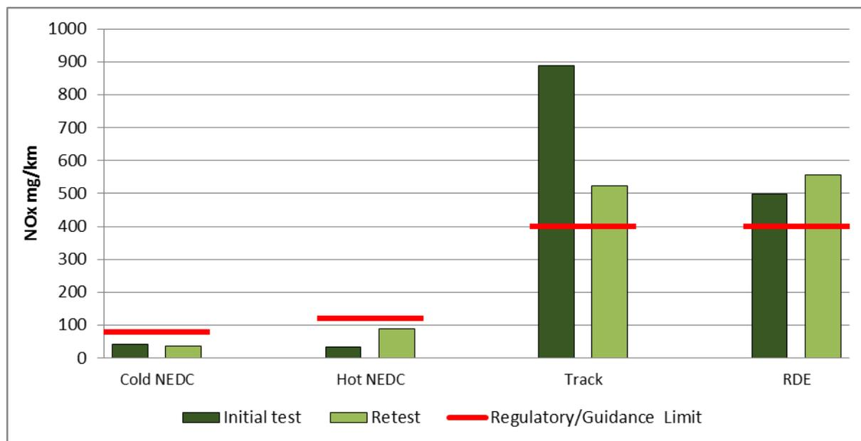
Figure 4-17: NO<sub>x</sub> emissions for the BMW 116D M Sport Shadow. Limit shown is the legislative limit for the NEDC (cold) test and the recommended guidance limits for the other tests
