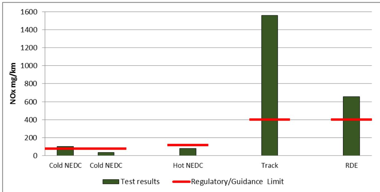
Figure 4-16: NO<sub>x</sub> emissions for the Nissan Qashqai N-Connecta DCI (vehicle 2). Limit shown is the legislative limit for the NEDC (cold) test and the recommended guidance limits for the other tests
