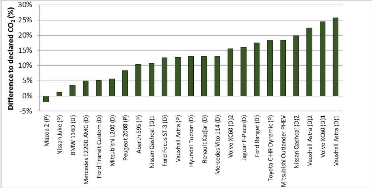
Figure 5-2: Percentage difference between the laboratory NEDC (cold) test CO<sub>2</sub> emissions and the type approval declared value
