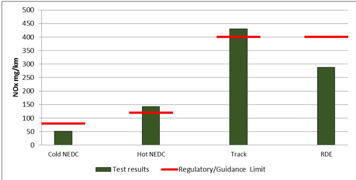
Figure 4-18: NO<sub>x</sub> emissions for the Ford Focus ST-3 TDCI Auto (initial). Limit shown is the legislative limit for the NEDC (cold) test and the recommended guidance limits for the other tests
