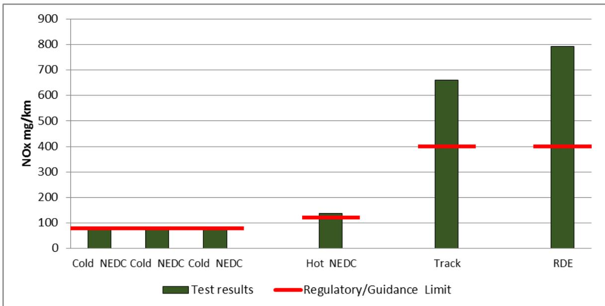
Figure 4-25: NO<sub>x</sub> emissions for the Volvo XC60 R-Design Lux D4 (2). Limit shown is the legislative limit for the NEDC (cold) test and the recommended guidance limits for the other tests
