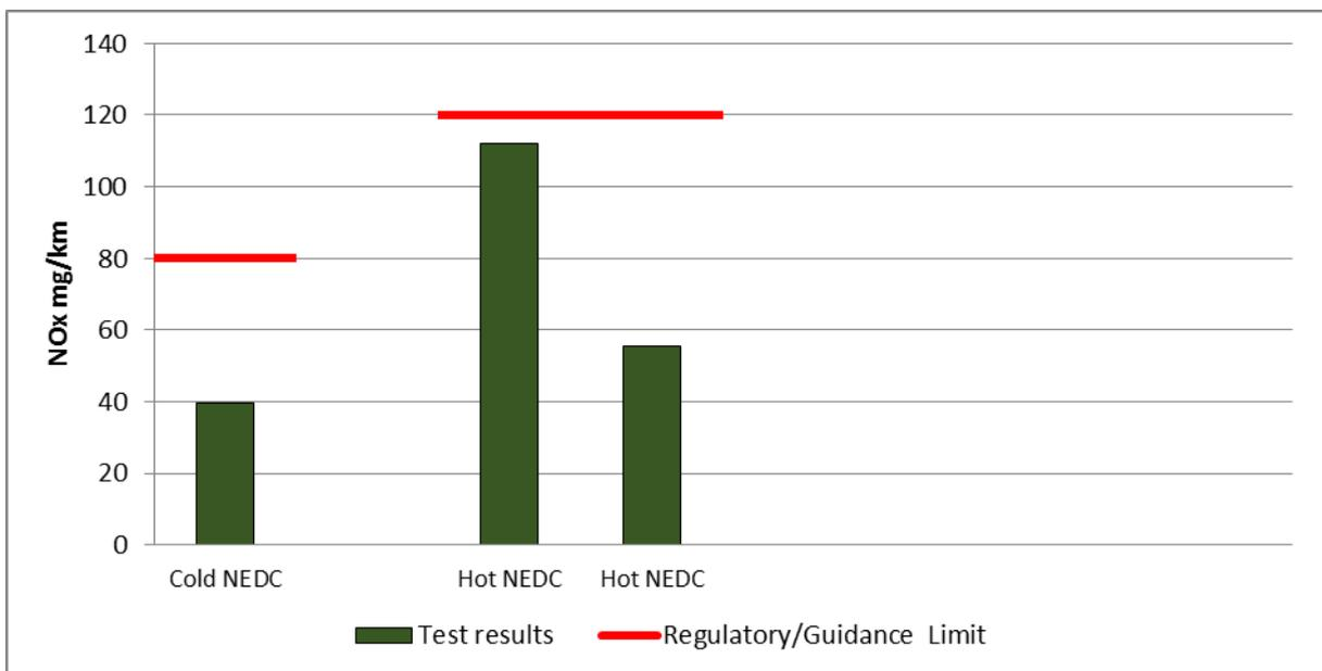
Figure 4-19: NO<sub>x</sub> emissions for the Ford Focus ST-3 TDCI Auto (retest). Limit shown is the legislative limit for the NEDC (cold) test and the recommended guidance limits for the other tests
