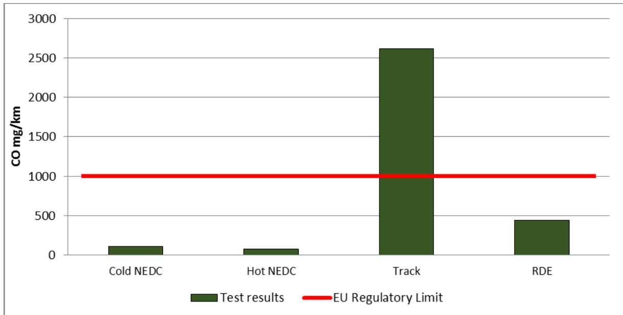
Figure 4-8: CO emissions for the Mazda 2. Limit shown is the legislative limit for the NEDC (cold) test
