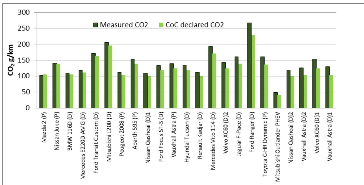
Figure 5-1: Type Approval and laboratory NEDC (cold) test CO<sub>2</sub> emissions
