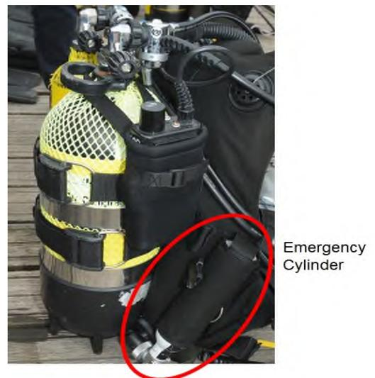
Figure 1.4.9 – Emergency Cylinder fitted to the lower right-hand side of the BCA jacket
