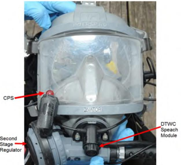
Figure. 1.4.7 – Full Face Mask with CPS, SSR and DTWC highlighted
