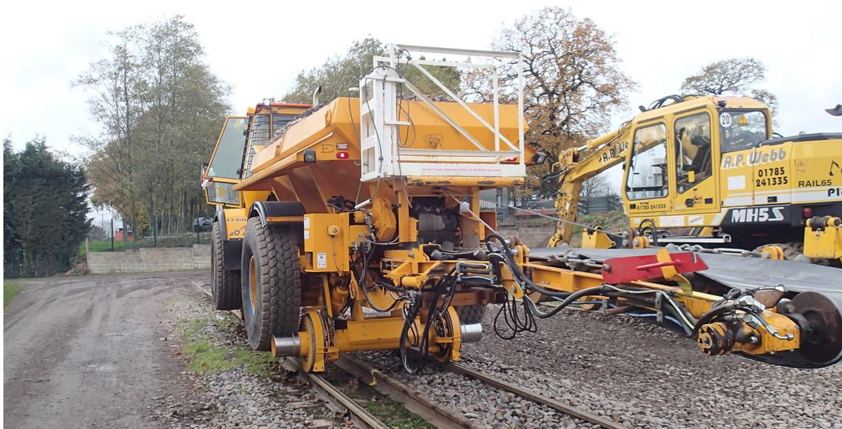
Figure 9: Rear platform on the ballast distributor
