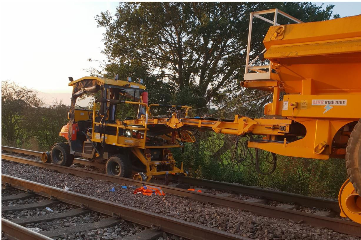
Figure 7: The position of the two vehicles after the collision
