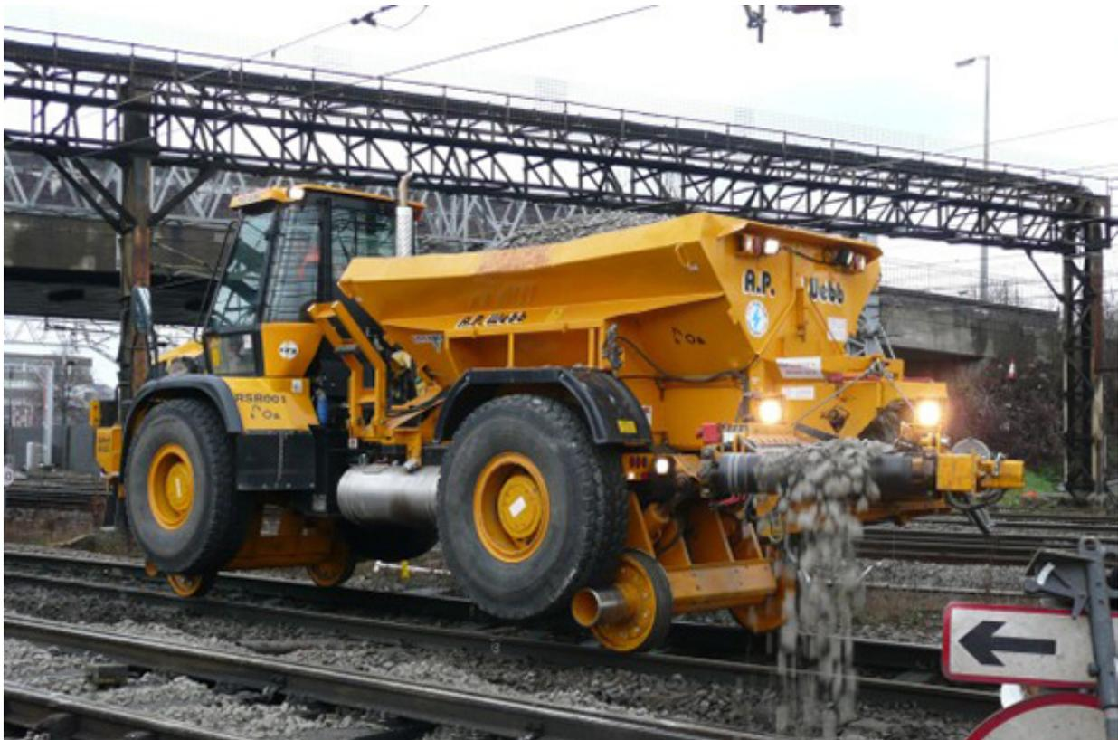
Figure 5: A ballast distributor dropping ballast (courtesy of AP Webb Plant Hire)
