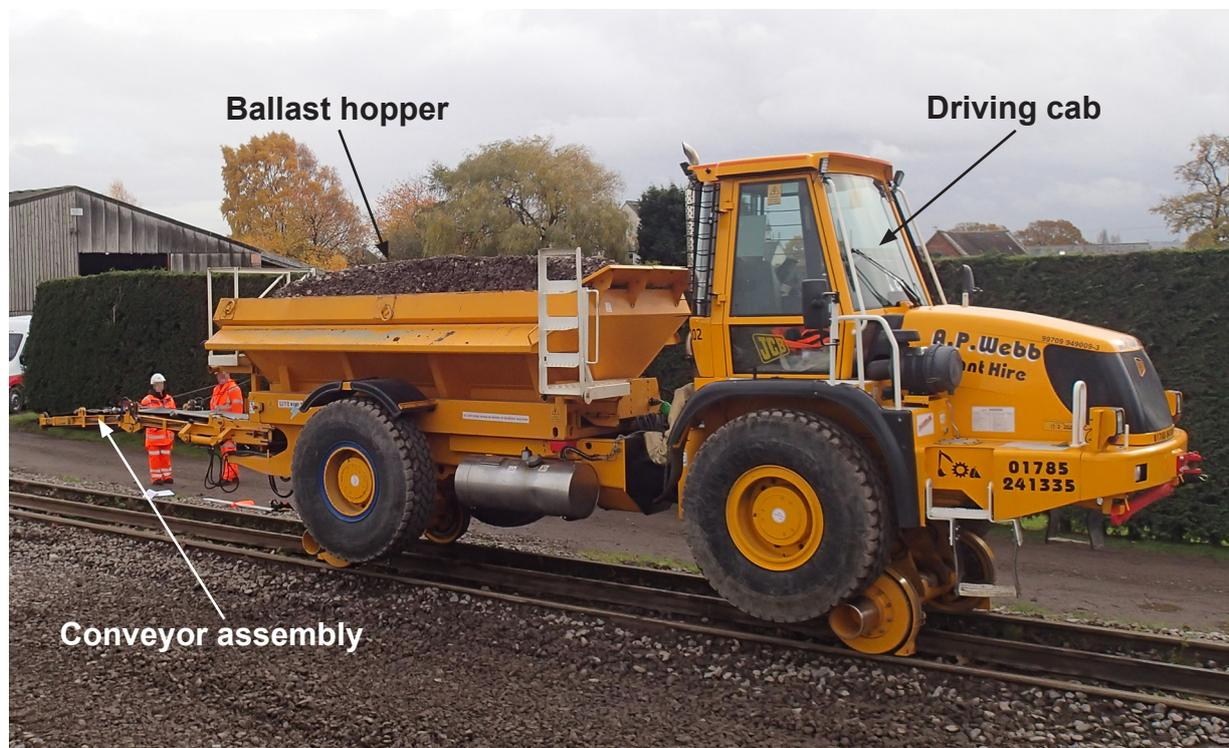
Figure 3: The ballast distributor road-rail vehicle
